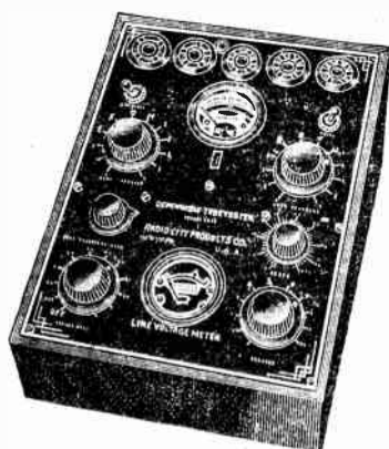
FIG. 10-5.—Dependable Model 304 tube tester. This is a direct-reading tester of the emission-test type. Its schematic circuit diagram is shown in Fig. 10-6.
