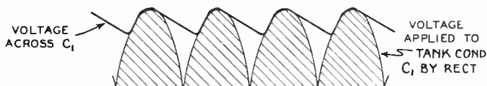
FIG. 20-23.—The wave-form of the voltage across the tank condenser C_1 in a condenser-input type filter such as is shown at (B) of Fig. 20-21.
