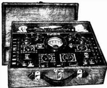
FIG. 14-5.—A typical single-meter point-to-point set analyzer. A unique switching arrangement makes jumper leads unnecessary. "Breakdown" schematic circuit diagrams of unique portions of this analyzer are shown in the next four illustrations. (Supreme Model 91.)
