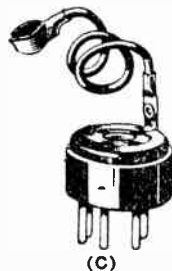
FIG. 8-19.—(A) Wiring of an adapter for testing the 57, 58, 77, 78, 6C6, 6D6, etc. tubes in the '27 or '37 sockets of tube checkers. (B) Adapter for testing the 57, 58, 6C6, 6D6, etc., in the '24 or '36 sockets. (C) A commercial adapter of this type. Notice the flexible lead and clip for connecting to the control-grid cap on the tube.
