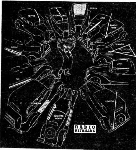
FIG. 27-23A. — Twelve different types of auto-radio aerials which are in popular use. All but the "screen" and "open" types are used on cars having "all-steel" tops, since they are mounted on the outside of the car proper. This makes a wide variety of aerials to choose from.
