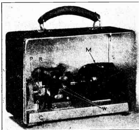
FIG. 25-35.—A portable motor-driven "frequency-wobbler" and saw-tooth voltage synchronizing unit for use with a cathode-ray oscilloscope when aligning tuned circuits. (Model TMV-128-A)
