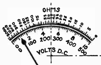
FIG. 5-9.—Reduced facsimile reproduction of the scale of the ohmmeter illustrated in Figs. 5-7 and 5-8.
