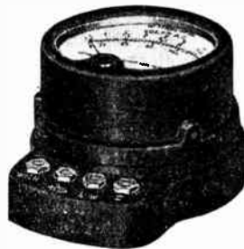
FIG. 2-32.—A portable triple-range a-c voltmeter of the movable-iron type. Four terminals are provided—one is a common terminal. (Weston Model 528.)
