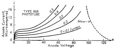
Fig. 10-7.—Current-voltage characteristics for the type 868 gas phototube.
