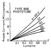
Fig. 10-8.—Static curves of anode current vs. luminous flux for the type 868 gas phototube.
