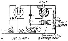
Fig. 9-37.—Thyratron relaxation oscillator in which the condenser charging current is controlled by a pentode.
