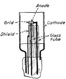
Fig. 9-14.—Electrode structure of the grid-glow tube.
