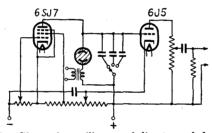
Fig. 9-10.—Glow-tube oscillator and direct-coupled amplifier.
