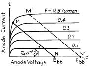
Fig. 10-21.—Anode diagram for vacuum phototube.
