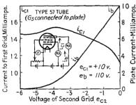
Fig. 3-10.—Characteristics showing first-grid current  $i_{c1}$  and plate current  $i_{b}$  of a space-charge tetrode as a function of second-grid voltage  $e_{c2}$ .
