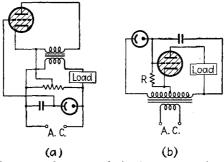
Fig. 10-19.—Thyratron phase-control circuits incorporating phototubes, by means of which large currents may be controlled by illumination.
