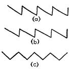
Fig. 8-20.—Typical waves of condenser voltage in the circuits of Figs. 8-18 and 8-21.
