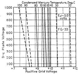
Fig. 9-23.—Grid-control characteristics of the type FG-33 thyratron.
