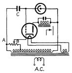
Fig. 10-16.—A-c-operated forward phototube circuit.
