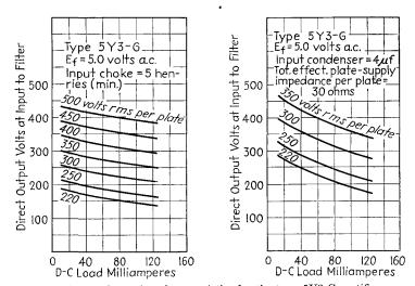
Fig. A-15.—Operation characteristics for the type 5Y3-G rectifier.
