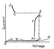
Fig. 9-1.—Current-voltage characteristic of a typical gas-filled cold-cathode diode.
