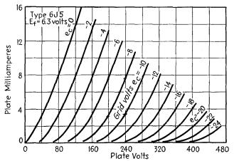
Fig. A-3.—Average plate characteristics for the type 6J5 triode.
