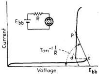
Fig. 9-2.—Anode diagram of a glow-discharge tube.
