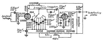
Fig. 12-16.—Sweep oscillator and amplifier.
