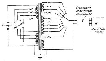
Fig. 6-31.—Circuit diagram of General Radio power-output meter.
