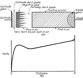
Fig. 9-3.—(a) Appearance of the glow discharge between plane-parallel electrodes; (b) potential distribution in the glow discharge between plane-parallel electrodes.
