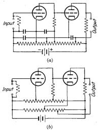
Fig. 5-3.—Direct-coupled amplifiers with single source of grid and plate voltages.
