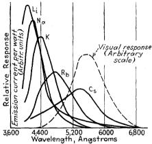
Fig. 10-1.—Current-wave-length characteristics for the alkali metals.
