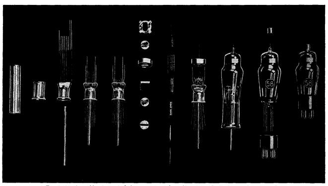
Fig. 2-13.—Assembly of a typical glass receiving tube. (Courtesy of Radio Corporation of America.)
