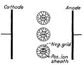
Fig. 9-12.—Formation of a positive-ion sheath around a negative grid in an ionized gas.
