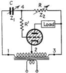
Fig. 9-41.—Simple type of practical phase-control circuit.
