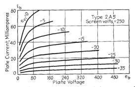
Fig. 3-14.—Plate characteristics of a typical power pentode.
