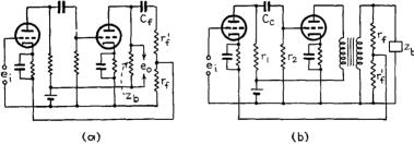
Fig. 6-35.—Inverse-feedback amplifier circuits.
