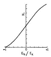
Fig. 7-8.—Ideal linear diode modulation characteristic.
