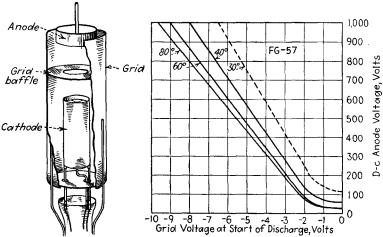
Fig. 9-20.—Electrode Fig. 9-21.—Grid-control characteristics of the structure of the type FG-57 type FG-57 thyratron. negative-grid thyratron.
