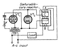
Fig. 9-51.—Phase-control circuit using saturable reactor.
