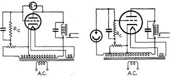
Fig. 10-14.—A-c-operated forward phototube circuit.
