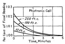
Fig. 10-33.—Curves showing fatigue in the Photronic cell.
