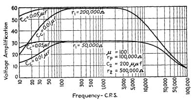
Fig. 6-14.—Frequency-response characteristics for a typical resistance-coupled amplifier.
