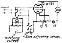
Fig. 12-11.—Slide-back voltmeter using tetrode with space-charge connection.
