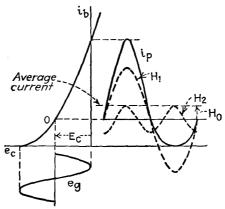
Fig. 3-21.—Generation of second-harmonic and steady components of plate current by tube with parabolic transfer characteristic.
