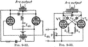
Figs. 9-32 and 9-33.—Self-excited parallel inverters.
