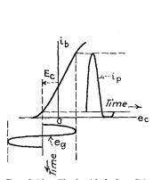
Fig. 5-16.—Single-sided class B2 operation.
