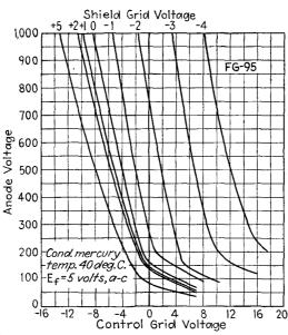
Fig. 9-25.—Grid-control characteristics of the type FG-95 shield-grid thyratron.
