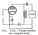
may be done by using an output transformer as in Figs. 5-7 to 5-10, 5-12, and 5-13, a resistance-capacitance network as in Figs. 5-5 and 5-11, a condenser-choke combination as in Fig. 5-14, or a tap on the voltage supply (bridge output), as in Fig. 5-3. The dotted lines in Figs. 5-5 and 5-14 show an alternative connection of the load. The advantage of this connection is that
