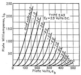
Fig. A-10.—Average plate characteristics for the type 2A3 triode.
