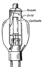
Fig. 9-18.—Electrode structure of the type FG-67 thyratron.
