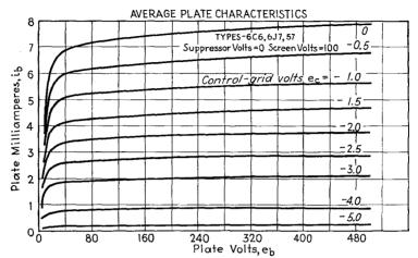
Fig. 3-13.—Plate characteristics of a typical voltage pentode.
