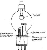
Fig. 9-55.—Structure of typical glass thyratron. (Courtesy of Westinghouse Electric and Manufacturing Company.)
