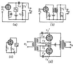
Fig. 6-34.—Inverse-feedback amplifier circuits.
