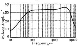
Fig. 6-18.—Frequency-response curve of a transformer-coupled audio-frequency amplifier.
