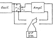
Fig. 6-23.—Circuit for the measurement of voltage amplification.
