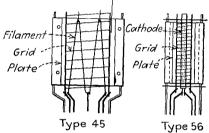
Fig. 3-1.—Electrode structure of typical filamentary and heater-type triode receiving tubes.
