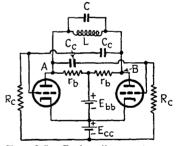
Fig. 8-5.—Push-pull negative-resistance oscillator.
