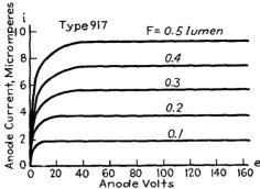
Fig. 10-4.—Current-voltage characteristics for the type 917 vacuum phototube.
