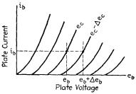
Fig. 3-5.—Method of determining triode amplification factor from plate characteristics.
