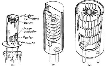
Fig. 9-16.—Typical indirectly heated cathodes used in hot-cathode are tubes.
