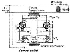
Fig. 9-52.—Thyratron welding control circuit.
