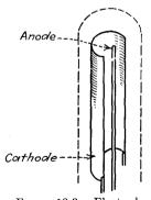
Fig. 10-3.—Electrode structure of a typical phototube.
