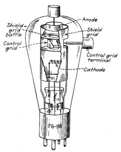
Fig. 9-24.—Electrode structure of the type FG-98 shield-grid thyratron.
