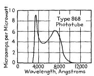
Fig. 10-2.—Current-wave-length characteristic for the type 868 phototube.
