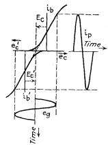
Fig. 5-17.—Push-pull class B2 operation.
