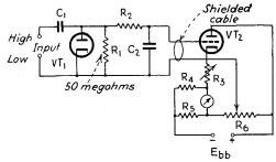
Fig. 12-9.—General Radio diode voltmeter.
