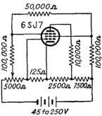
Fig. 6-27.—Pentode trigger circuit.
