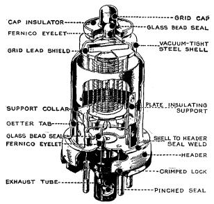
Fig. 2-14.—Structure of typical metal receiving tube.
