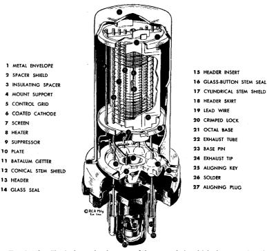
Fig. 3-11b.—Typical metal voltage-amplifier pentode in which the control-grid connection is brought out through the base. Note conical stem shield 12. (Courtesy of Radio Corporation of America.)
