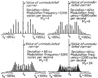
Fig. 7-20.—Amplitudes and distribution of side-frequency components of frequency-modulated wave for 60-ke deviation and four values of modulation frequency.
