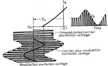
Fig. 7-9.—Linear grid modulation. A parallel resonant circuit converts the carrier and side-frequency components of plate current into output voltage.
