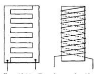
Fig. 10-24.—Two forms of grids used in selenium cells.
