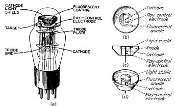
Fig. 12-17.—Structure of the type 6AB5 electron-ray tube.
