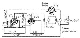
Fig. 6-25.—Vacuum-tube voltage regulator for a d-c generator.
