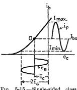
Fig. 5-15.—Single-sided class A1 operation.
