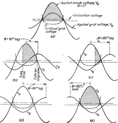
Fig. 9-38.—Variation of the firing period of a thyratron by change of phase angle between grid voltage and anode voltage.
