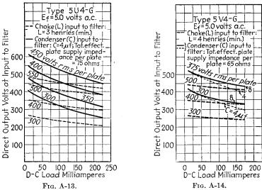
Figs. A-13, A-14.—Operation characteristics for the type 5U4-G rectifier.
