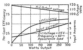
Fig. 9-34.—Performance curves for a parallel inverter.
