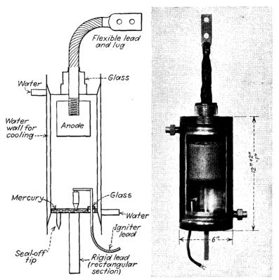
Fig. 9-56.—Structure of type WL-651 water-cooled metal ignitron. (Courtesy FG-258A water-cooled metal igniof Westinghouse Electric and Manufactur- tron. (Courtesy of General Electric ing Company.)
