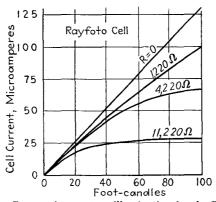
Fig. 10-28.—Curves of current vs. illumination for the Rayfoto cell.
