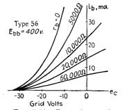
Fig. 3-24.—Dynamic transfer characteristics of the type 56 triode for five values of load resistance at fixed plate supply voltage.
