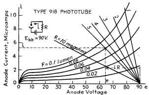
Fig. 10-22.—Anode diagram for the type 918 gas phototube.
