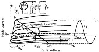
Fig. 4-11.—Exact plate diagram for nonreactive load.  $r_b > R_b$ . Conditions of operation such that average plate current increases with excitation.
