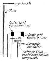
Fig. 9-63.—Strobotron electrode structure.
