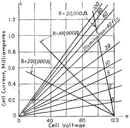
Fig. 10-27.—Typical current-voltage diagram for a selenium cell. value of illumination is independent of cell voltage, the current-voltage curves are straight lines and may be readily
