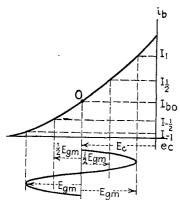
Fig. 4-15.—Use of the dynamic transfer characteristic in the application of Eqs. (4-25).
