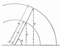
Fig. 75.—Current and voltage in phase. The maximum value of voltage greater (or drawn to different scale) than the maximum value of the current.
