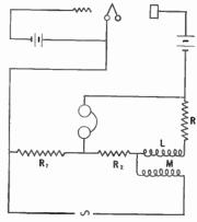
Fig. 127.—A bridge for measuring  $R_p$ .
