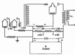
Fig. 256.—How the voltage divider originates.
