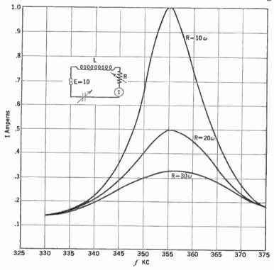
Fig. 92.—Effect of resistance on a resonance curve. Note that the current far from resonance is not shanged so much as the resonant current.
