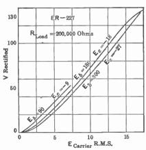
Fig. 210.—Plate rectification "power" detector characteristic.
