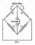
Fig. 54.—If A and B are so adjusted that there is no sound in the phones,
