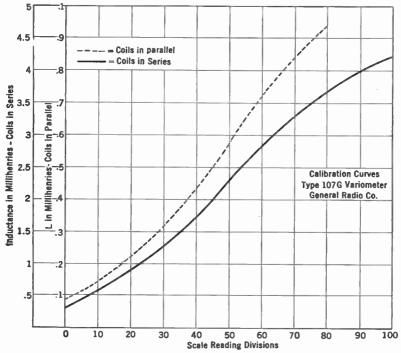
Fig. 60.—Calibration of a standard variable inductance.
