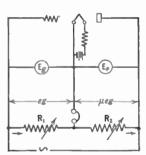
Fig. 125.—Bridge for determining amplification factor.
