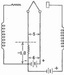
Fig. 134.—Obtaining grid bias by means of filament-current flowing through a resistance.
