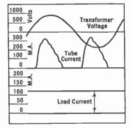
Fig. 253.—High instantaneous current required from rectifier with capacitive input.
