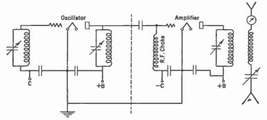
Fig. 283.—Master oscillator-power amplifier transmitting circuit.
