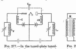
Fig. 277.—In the tuned-plate tuned-grid circuit  $C_{qp}$  acts as the feedback agency.
