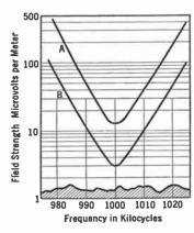
Fig. 229.—Illustrating real and apparent selectivity.
