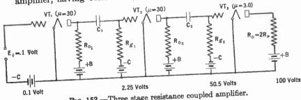
Fig. 153.—Three stage resistance coupled amplifier.
