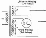
Fig. 238.—Operating rectifier filament from a. c.
