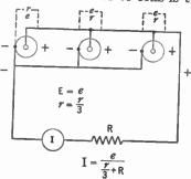
Fig. 39.—Cells in parallel.
