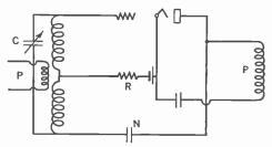
Fig. 195.—Rice neutralized circuit.
