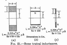
ones having over 100 henries in inductance. Broadcast frequency tuning coils are of the order of 300 microhenries, and may be from 1 to 3 inches in diameter wound with from No. 30 to No. 20 wire of from 50 to 100 turns or so. There
