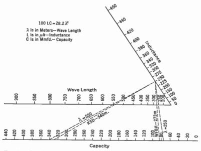
Fig. 93.—Drawing a straight line through two points (L and λ for example) and intersecting the third line gives the unknown quantity desired (C).
