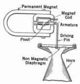
Fig. 231.—Horn type speaker mechanism.
