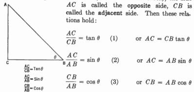
Fig. 71.—Trigonometric "functions."
