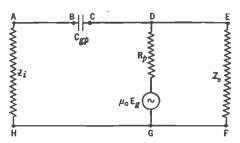
tiplied by the  $\mu$  of the Fig. 219.—Equivalent circuit of screen grid tube is shunted across — tube and input and output impedances.
