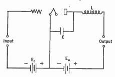
Fig. 204'—To keep radio-frequency currents from the output, a low impedance path (C) and a high series impedance (L) are used.
