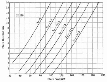
Fig. 120.—Plate current—plate voltage curves.
