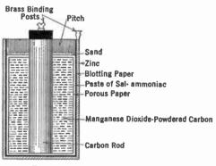
Fig. 36.—Construction of dry cell.
