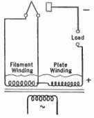
Fig. 245.—Single wave rectifier circuit employed by some Western Electric systems
