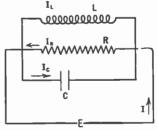
Fig. 84.—In a parallel correct I may be very small compared to  $I_L$  or  $I_C$ .
