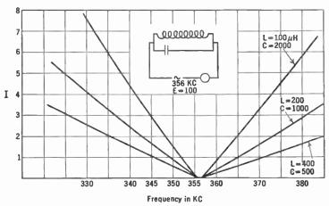
Fig. 100.—How varying  $\frac{L}{C}$  affects sharpness of tuning of an anti-resonant circuit.
