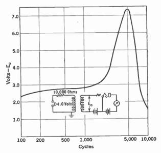
Fig. 161.—Characteristic of single andio transformer.
