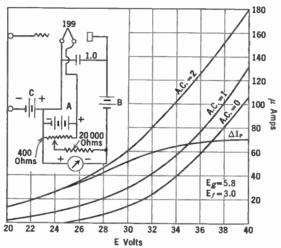
Fig. 205.—Calibration and circuit of vacuum tube voltmeter
