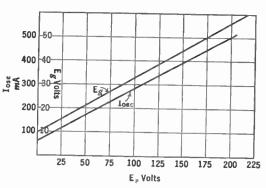
output Fig. 280.—Relation between plate voltage and compli- oscillatory current and grid bias.
