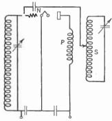
Fig. 197.—Hazeltine neutralized circuit.
