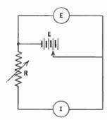
Fig. 12.—A circuit for testing Ohm's law.
