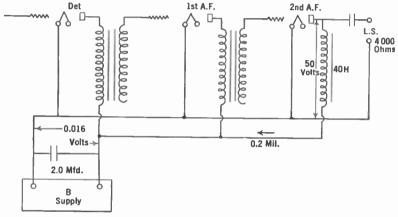
Fig. 174.—The proper output connection.
