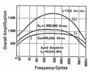
Fig. 157.—Frequency characteristic of resistance- and inductance-coupled amplifiers.
