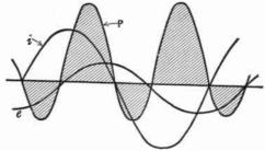
Fig. 87.—Power in a capacitive circuit.
