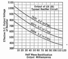
Fig. 252.—Output of modern rectifier.
