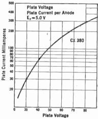
Fig. 242.—Characteristic of double wave rectifier tube.
