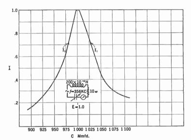
Fig. 98.—If I<sub>1</sub>, and I<sub>2</sub> are equal to 0.707 times the resonant or maximum current, the resistance of the circuit may be calculated.
