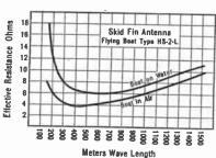
Fig. 300.—Antenna resistance.
