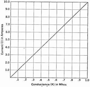
Fig. 15.—Conductance  $\left(\frac{1}{R}\right)$  plotted against current.
