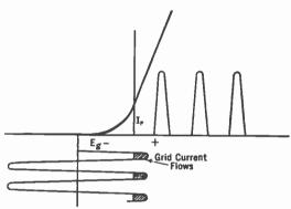
Fig. 272.—Form of plate current waves when tube current is so biased that lower part of characteristic is used. Thus  $\, c \,$
