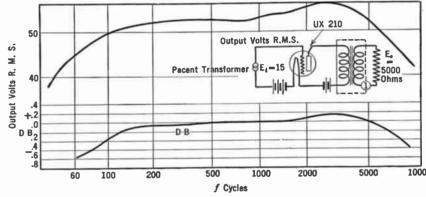
Fig. 169.—Transmission characteristic of output transformer.
