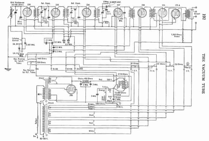
Fig. 130.—Circuit diagram of 1929 receiver—Majestic Model 70-B.
