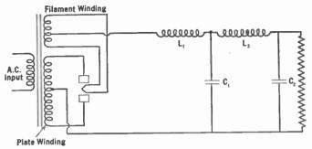
Fig. 254.—Inductance input type of filter.
