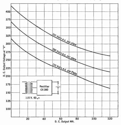
Fig. 7.—A "B eliminator" regulation curve.
