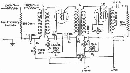
Fig. 176.—A high quality, well-filtered audio amplifier.
