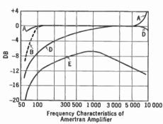
Fig. 177.—Effect of filtering the audio amplifier of Fig. 176.
