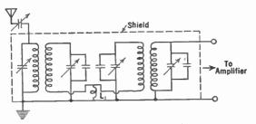
Fig. 224.—Band pass circuit.
