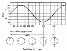
during which the voltage is in the same direction, is voltage as shown on the graph—called a called an alternation.
