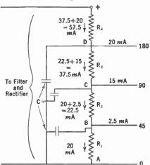
Fig. 261.—Designing the voltage divider.
