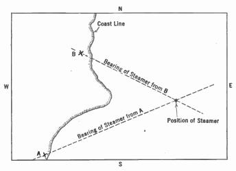
Fig. 304.—Method of plotting a ship's position by obtaining two bearings from land stations.
