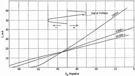
Fig. 164.—Flattening effect of increasing load resistance.
