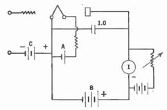
scale is available then  $_{\rm Fig.}$  206.—Method of balacing out the steady for plate current changes plate current from the indicating meter.
