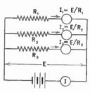
Fig. 21.—A parallel circuit.
