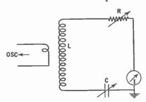
Fig. 88.—When L is coupled loosely to a generator and C is varied, the current indicated at I will go through a maximum like that in Fig. 90.
