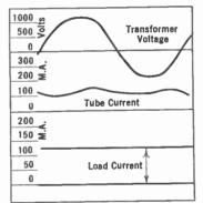
Fig. 255.—Reduced tube current in an inductance input filter.
