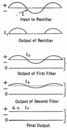
Fig. 63.—How the current in a "B eliminator" varies. The half waves from the rectifier are smoothed out by series inductances and parallel condensers until at I<sub>4</sub> it is pure direct current.
