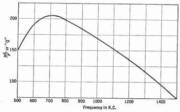
Fig. 101.—How the "Q"  $(L\omega/r)$  of a coil varies with frequency.
