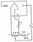
Fig. 113.—Circuit for testing effect of plate voltage on emission.
