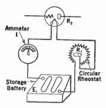
Fig. 18.—A series circuit used in radio apparatus.
