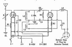
Fig. 220.—A screen grid blocking tube between antenna and oscillating detector; all arranged to be plugged into a broadcast or other receiver.
