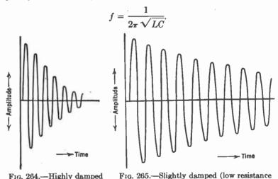
If the resistance is too great, the spark will not set up such waves. The circuit is then non-oscillatory. If the resistance is decreased to a very low value, the number of oscillations that take place before the spark finally dies out becomes very great.
