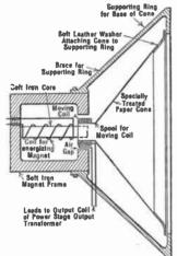
Fig. 233.—Modern "dynamic" or moving coil loud speaker.
