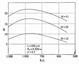
How Fig. 189.—Relation between mutual inductance ity is and gain in an r.-f. amplifier.
