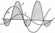
Fig. 86.—In an inductive circuit some power curve results although is consumed and some (the shaded areas the instantaneous power below the line) is returned.
