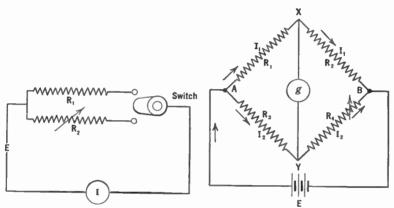
Fig. 31.—Measuring resistance by comparison.
