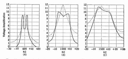
Fig. 225.—Quantitative data on band pass amplifier-tube and tuned coils.
