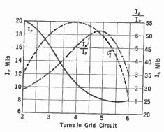
Fig. 279.—Effect of varying grid turns, thereby changing excitation.
