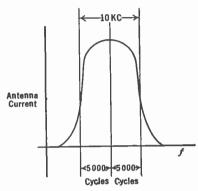
if not impossible to attain. In Fig. 181.—A flat-topped steep-sided repractice, the response curve is sponse curve is the ideal. This curve either so broad that stations approaches it.
