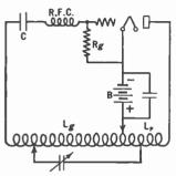
Fig. 273. — Hartley oscillator; grid current through  $R_{\sigma}$  provides negative bias for the grid; choke R.F.C. prevents high-frequency oscillations.
