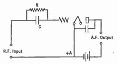
Fig. 207.—Grid leak-grid condenser detector.
