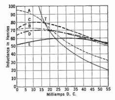
FIG. 62.—Variation of inductance with air gap.
