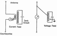
Fig. 292.—Current feed and voltage feed antenna circuits.
