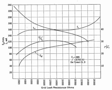
Fig. 281.—Effect of varying grid leak resistance.
