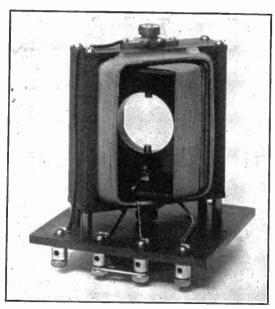
Fig. 59.—General Radio Company variable inductance.
