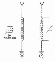
Fig. 109.—To measure capacity of an antenna.
