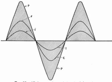
Fig. 85.—All the power in a resistive circuit is used up.
