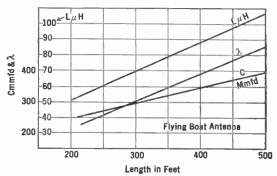
Fig. 305.—Characteristics of airplane antenna.
