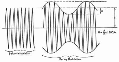
Fig. 201.—Unmodulated and modulated wave.
