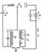
Fig. 271.—Tuned plate circuit (grid tickler) oscillator.
