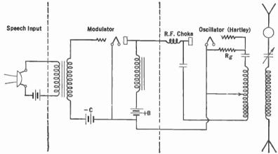
Fig. 295.—Practical modulated oscillator circuit.
