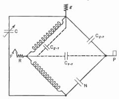
Fig. 196.—Equivalent bridge circuit of Fig. 195.
