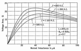
Fig. 187.—Relation between coupling and amplification.
