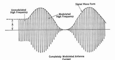
Fig. 296.—A radio frequency wave before and after complete modulation.
