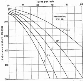
Fig. 111.—Curves showing the inductance of a coil as a function of length of winding and turns per inch.
