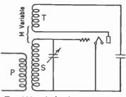
Fig. 191.—A simple regenerative circuit.
