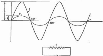
Fig. 74.—Current and voltage in phase.
