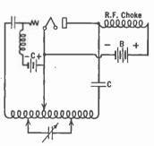
Fig. 274.—Shunt-feed Hartley osfrom tuning condenser plates.
