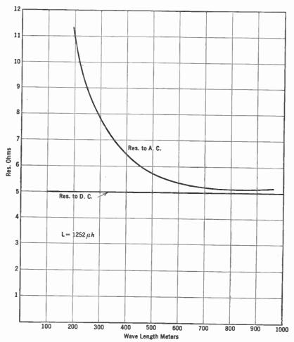
Fig. 102.—High-frequency resistance of a coil.
