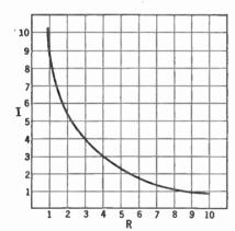
Fig. 14.—The result of plotting current ratus is at hand, connect it up as in against resistance.
