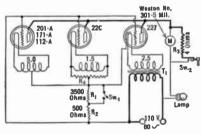
Fig. 129.—An a.-c. tube-tester.
