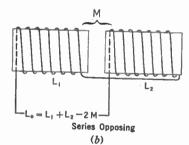
Fig. 52.—Coils may be connected so that their fields aid or "buck" and hence so that the total inductance is increased or decreased.
