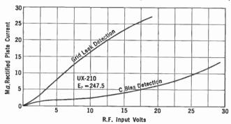
Fig. 212.—Comparison of grid leak and C bias detection.
