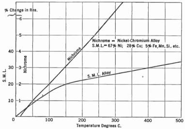
Fig. 3.—Effect of temperature on resistance.
