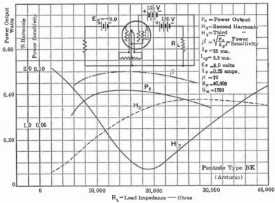
Fig. 149.—Power output and harmonic content of output of pentode tube.
