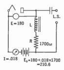
Fig. 10.—A choke-condenser coupling circuit.
