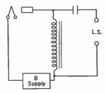
Fig. 172.—Here the loud-speaker currents must flow through the B supply to return to the filament.
