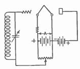
Fig. 194.—Potentiometer method of controlling oscillations.
