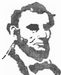
FIG. 309.—Picture transmitted by very simple 1933 system (Hogan).
