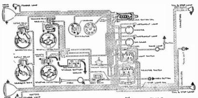
Note: 931-R Generator has Model 5540 Voltage Control Unit mounted M Generator Field Frame.
