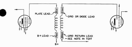
Standard RMA Color Code for the leads of intermediate-frequency transformers. (See accompanying text for explanation).
