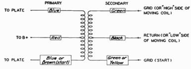
Standard RMA Color Code for the leads of audio-frequency transformers. (See accompanying text for explanation).
