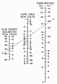
TRANSFORMER TURNS-PER-VOLT CHART: Knowing the flux density and the core area, the turns-per-volt for either a primary or a secondary winding may be determined by merely drawing the straight line (A-A) from the proper point on the "FLUX DENSITY" line through the proper point on the "CORE AREA" line—the extension of this line intersects the "TURNS-PER-VOLT" line at the point which represents the turns-per-volt of the transformer.
