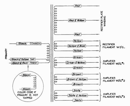
Standard RMA Color Code for the leads of radio power transformers. (See accompanying text for explanation).
