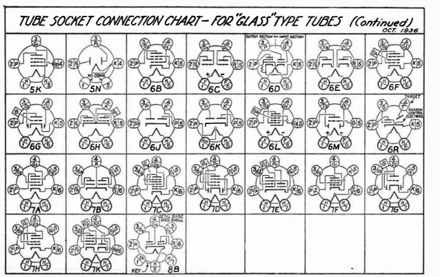
SEC. ഗ "GLASS" RADIO TUBE CHARACTERISTICS CH'T. 9-9
