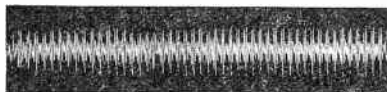
Fig. 158. Photograph of Wave Form of "Middle A" International-Pitch Tuning Fork, 435 Vibrations Per Second.
