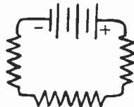
Fig. 31. Three Resistance Coils in Series.
