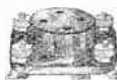
Fig. 269b. Socket for "The New X Tubes." This will accommodate either dry-cell or storage-battery tubes.
