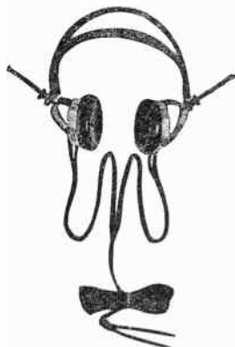
Fig. 163a. Modern Telephone "Head Set" used in Radio.
