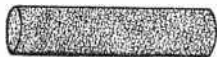
Fig. 10. The Position of the Molecules in an Unmagnetized Piece of Iron or Steel, or of Steel Filings in a Glass Tube.
