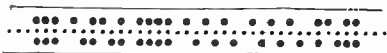
Fig. 524a. Piece of Code Tape Produced by the Machine Shown in Fig. 523. This Spells the Word "School."
