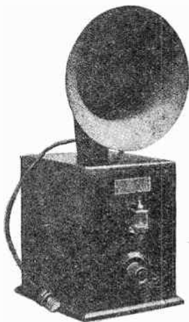
Fig. 468. A Receiver for "Wired Wireless." (Radio Broadcast.)
