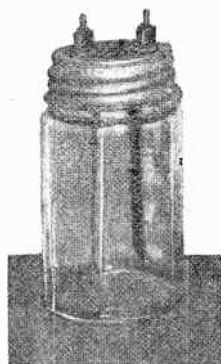
Fig. 318b. A Home-Made Chemical Rectifier.
