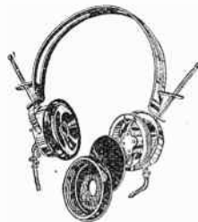
Fig. 165b. Four-Pole Telephone.
