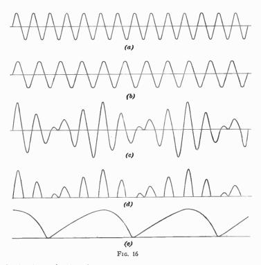
indication of what is known as a *beat current*. The amplitudes of the individual alternations of the beat current are not uniform. Periodical increases and decreases of amplitude are formed by the addition of the two separate waves. Maxi-
