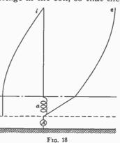
the capacity is increased in greater ratio than the decrease in inductance, which lowers the velocity and increases the fundamental wavelength.
