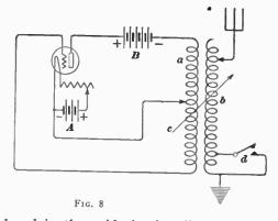
small oscillation produced in the grid circuit will produce a greater change of current in the plate circuit, including the coil a. This coil being coupled to the inductance coil b produces oscillations in the coil b which react upon coil c in the grid circuit. The feed-back then serves further to amplify or increase
