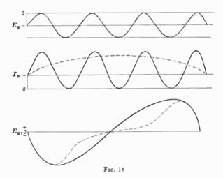
current reaches zero, and again goes to maximum positive when the average plate current suddenly reaches zero.
