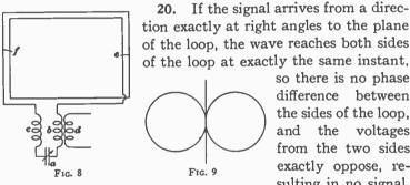
so there is no phase difference between the sides of the loop, and the voltages from the two sides exactly oppose, resulting in no signal.
