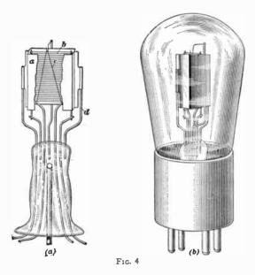
skeleton, construction, hence the name. It is placed between the filament and plate and is therefore directly in the electron path.
