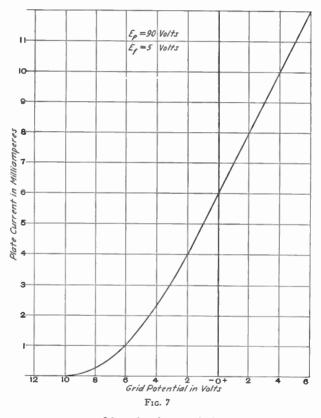
these measurements 90 volts is applied to the plate circuit. The designation for plate voltage is  $E_p$ , for filament voltage  $E_I$ , and for grid voltage  $E_q$ . Similarly, plate current is usually written as  $I_p$ , grid current as  $I_q$ , and filament current as  $I_I$ .
