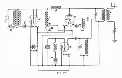
the current changes enough to produce a potential across the tube e suitable to require it to follow these changes. The radio-frequency output energy from tube e is therefore modulated in accord with the desired voice or music.
