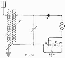
The action of breaking the circuit cuts up the received radio-frequency waves in t o groups of a few highfrequency oscillations, with quiet intervals separating the periods during which current is passing in the circuit. As has been explained, a detector rectifies any alternat-
