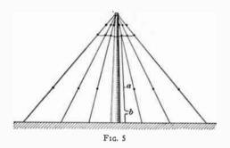
the wires, and there will be very little radiation. The wires should not make an angle of less than 50 or 60 degrees with the mast, and the lower ends should be insulated at some distance from the ground, so that the lower ends of the wires are half the mast height or more from the ground.
