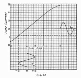
voltage to the most advantageous position on the tube's characteristic curve. Reference to Fig. 12 will clear this statement. The signal voltage  $E_g$  is shown impressed on
