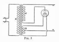
as shown in Fig. 3. The primary winding a of the transformer connects with an alternating-current supply line. The secondary winding b, known as the filament winding, gives a low-voltage output for heating the filament of the rectifier tube.
