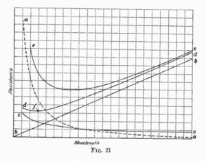
has one or more decided peaks. These peaks are usually caused by something in the field of the antenna which absorbs energy at that particular wavelength, as, for example, resonance in a guy wire, a mast, nearby antenna, tin roof, or other mass of metal.
