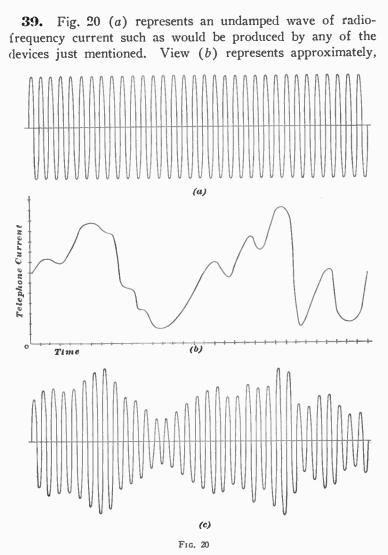
the variation in current in a circuit consisting of a transmitter in action, a battery, and connecting wires. The current waves, view (b), as produced by the human voice are, in general, of irregular form. When the oscillations, view (a), are modi-
