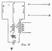
this reverses the direction of the loop voltage without changing the direction of the vertical antenna voltage, as already explained. The resultant reception diagram is a *cardioid*, or heart-shaped, curve, as shown in Fig. 11 at *a*. If the vertical-antenna voltage is not as strong as the loop voltage, the loop effect predominates, resulting in the
