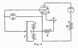
negative filament terminal. This makes the plate positive with reference to the filament and obtains the required condition of establishing a flow of current in the plate circuit, which is indicated on the milliammeter e.
