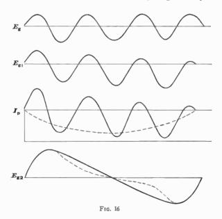
ing negative bias were placed on the grid. The actual voltage on the grid will, therefore, appear like that shown at  $E_{g1}$ , Fig. 16. The plate current  $I_p$  will follow the variations in the
