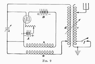
enough to sustain oscillations in the oscillating circuit a, c, d, this circuit may be used as a source of sustained waves.
