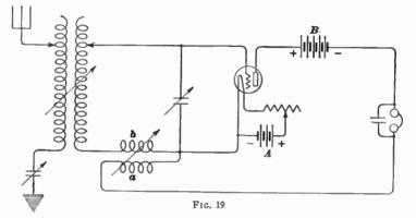
some of the plate current back to the grid could probably be applied with advantage to other circuits using the three-element tube, especially those using one or more stages of radio-frequency amplification.
