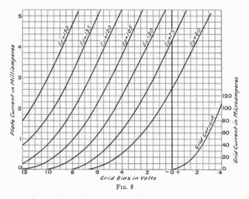
26. A number of curves may be combined in one figure to show the characteristics of a tube under different operating conditions. The curves in Fig. 8 show the grid-voltage plate-current condition of the 201-A type radio tube with plate potentials  $E_p$  of 60 to 150 volts. The grid-current curve shown in the lower right-hand corner is useful in some types of service. This curve is obtained with positive grid potentials, and is usually steeper with the lower plate potentials.
