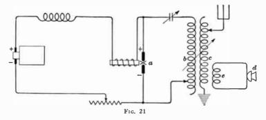
lating the carrier current. The arc set a shown in Fig. 21, operates in the usual manner to produce undamped waves of radio-frequency. These oscillations in the inductance coil b are transferred by induction to coil c in the antenna circuit. An ordinary telephone transmitter d, when spoken into, produces
