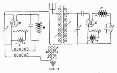
tion as a generator of high-frequency current oscillations as well as to function as a rectifier for the beat current.
