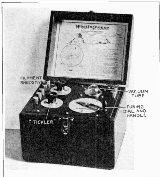
A medium-priced receiving set making use of a special vacuum tube which operates on a single dry cell, instead of a 6-volt storage battery.
