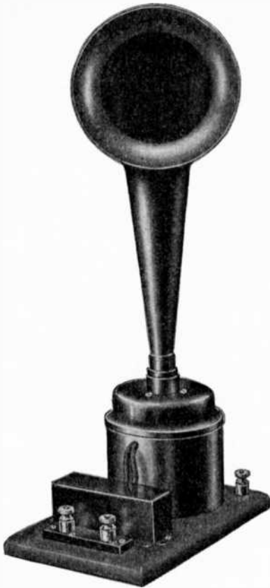
A popular small sized type of loud-speaker employed with the usual two-stage amplifier of the radio receiving set. A 6-volt storage battery is used to energize the field coils.
