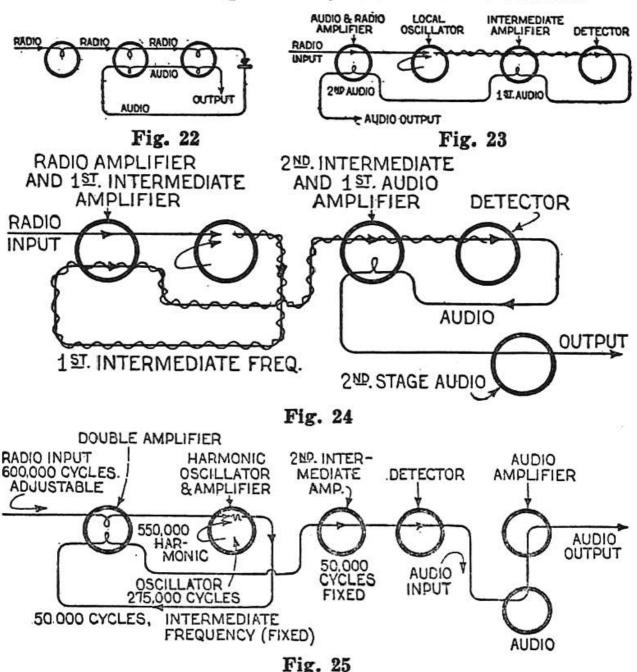
The heterodyne method of amplification brought out by Fessenden, improved by Armstrong and others, also permits use of reflex methods. Figs. 23, 24 and 25 show use of intermediate frequency or audio frequency reflex in heterodyne amplifier circuits.
