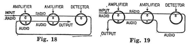
tion, proposed by Latour. Fig. 19 shows a reverse feed method for proportioning inputs and outputs. Fig. 20
