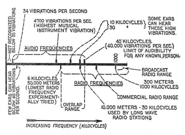
Fig. 3. Showing the overlap range between radio and audio frequencies.
