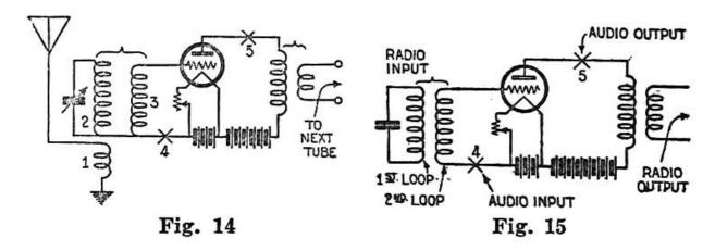
ings of the coils. Fig. 15 shows how insertion of audio input and output coils at such points tends to assist stabilization. Seldom will a series resistance 6, (shown in Fig. 16) be necessary, but when a very short aerial is employed, such a resistance, adjustable up to 300 ohms,
