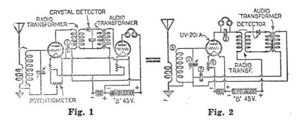
One stage of radio-frequency amplification, crystal detector and one stage of audio frequency amplification
