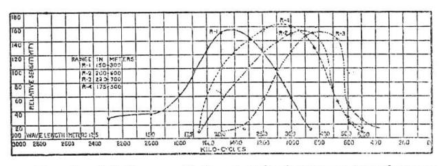
Fig. 49. Relative sensitivity of radio-frequency transformers at various wavelengths.
