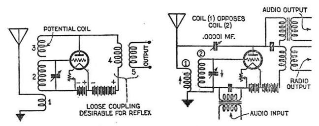
Fig. 12. A method of sta- Fig. 13. Another effective bilizing suggested by the author.method of stabilizing a reflex circuit.
