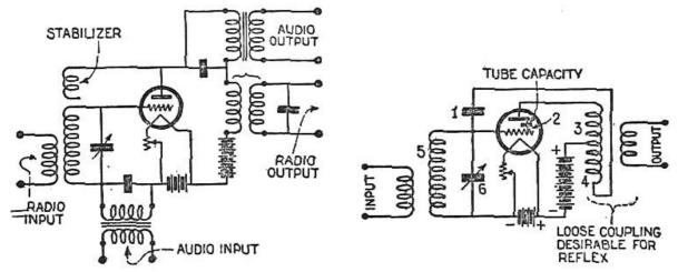
Fig. 8. Radio and audio inputs and outputs in combined amplification.
