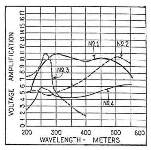
Fig. 48. Amplification curves of fixed radio-frequency transformers.
