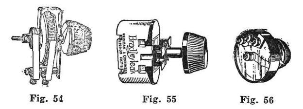
tiometer are shown in Figs. 54, 55 and 56. Non-inductive types are preferable for some circuits.
