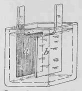
FIG. 1.—Simple arrangement of a lead acid cell.
