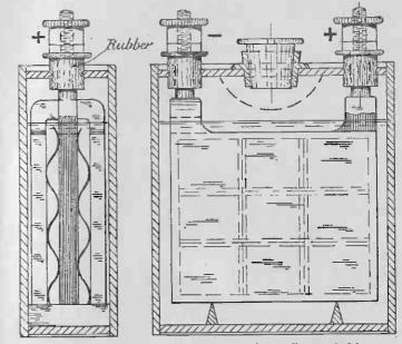
FIG. 2.—Typical construction of a 3-plate cell mounted in a celluloid case.
