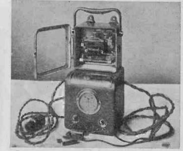
FIG. 31.—A transformer rectifier for charging from 200 volts, 50 cycles, down to 6 volts direct. Half-cycle rectification.
