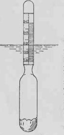
FIG. 35.—An acidometer or form of hydrometer for acid testing.
