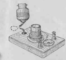
FIG. 26.—Sketch of small charging lampboard with directional galvo.
