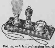
FIG. 25.—A lamp-charging board with directional ammeter or milliampmeter.
