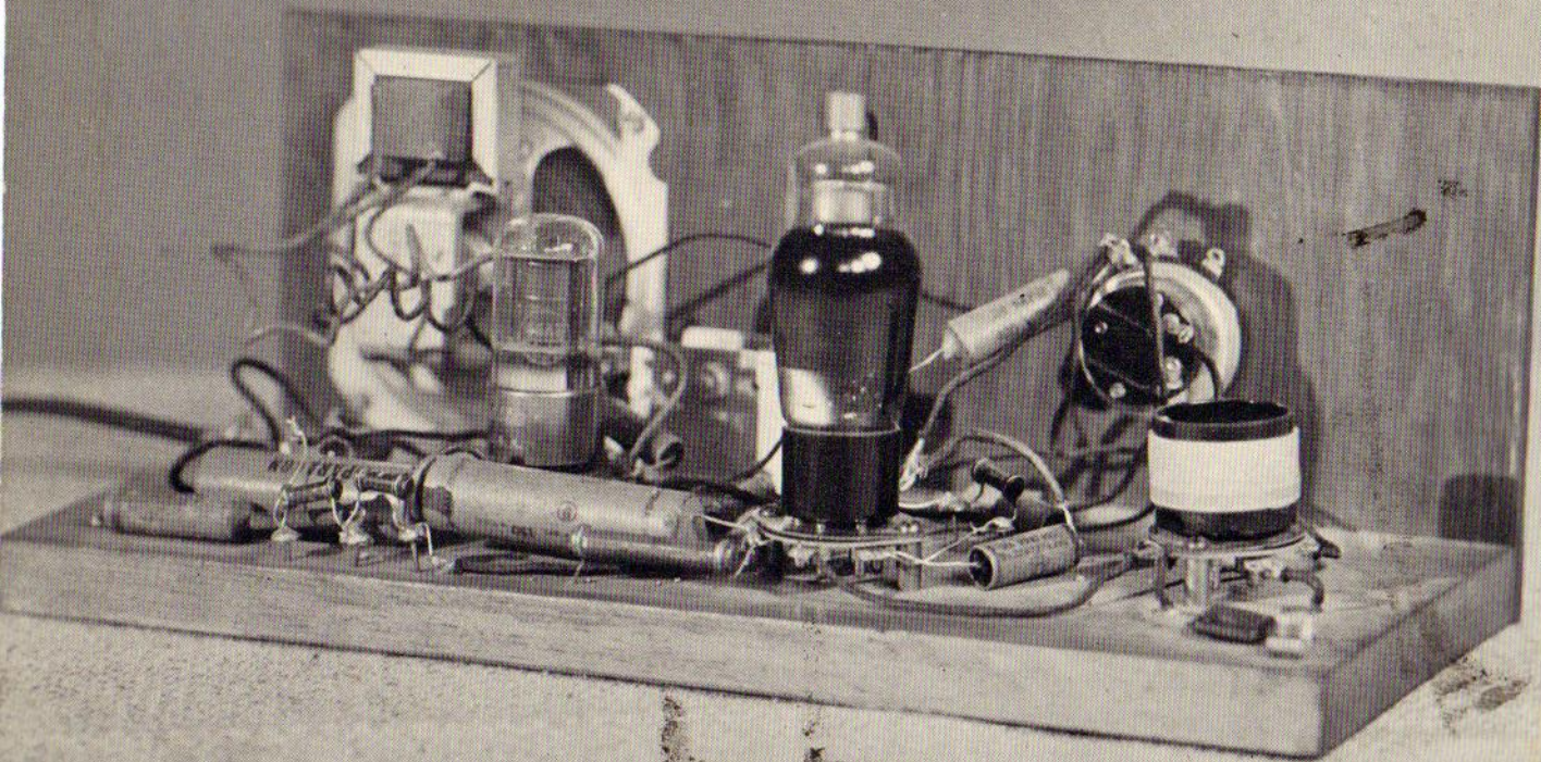
Rear view of the 2-tube A.C.-D.C. receiver with speaker.
