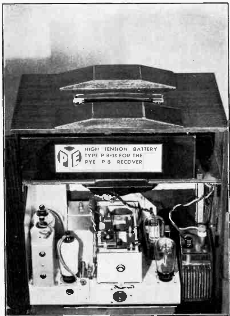
A MODERN BATTERY RECEIVER OF THE SEMI-PORTABLE TYPE
