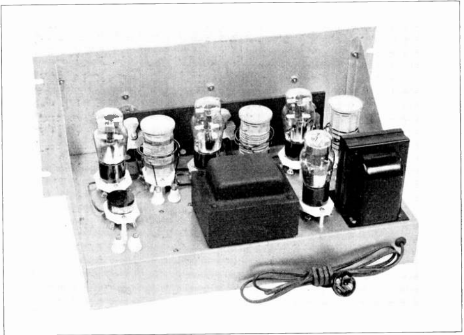
"3-53" 1936 Jones Exciter, 160 meters to 10 meters. The power supply, mounted on the Exciter chassis, makes this a complete and independent driving unit for a buffer-amplifier stage.
