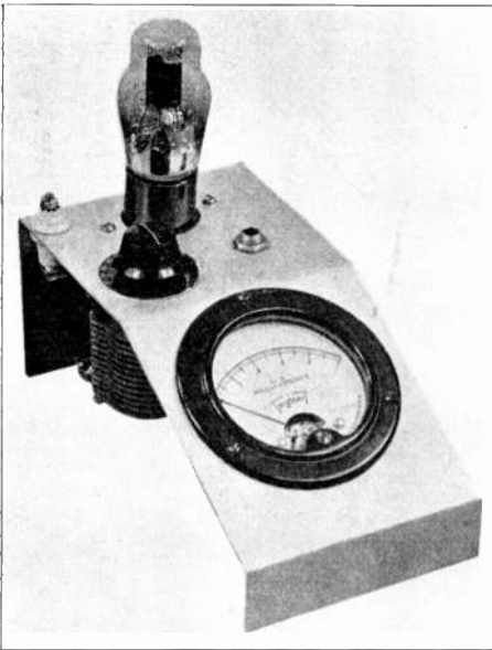
A piece of No. 12 gauge aluminum is bent in one piece to provide a mounting stand for the Overmodulation Indicator.
