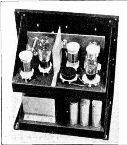
Relay rack mounting for exciter and buffer. Power supply on lower deck
