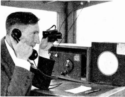
5-meter radiotelephony plays a major role in aiding the bridge builder. The illustration shows the San Francisco Bay Bridge operator conversing with the construction crew.
