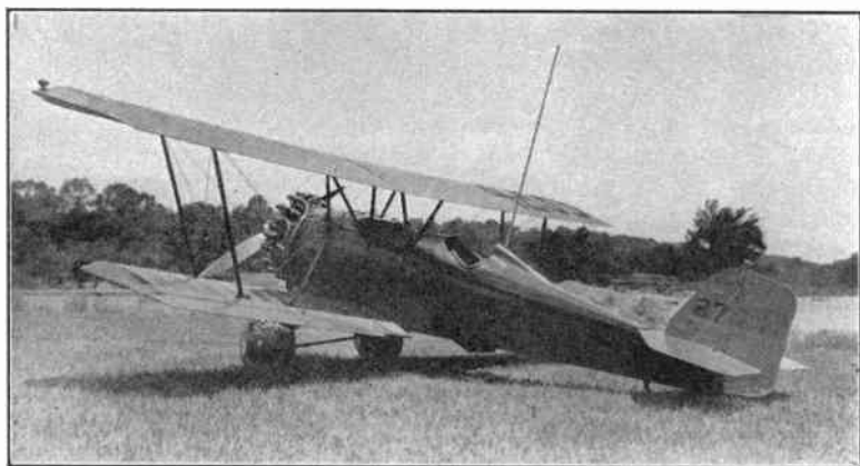
FIG. 276. Installation on Pitcairn PA-5 Mail Plane Showing Short Rigid Vertical Antenna.
