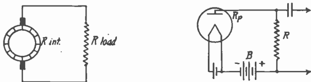
FIG. 87. The Output Rule—Showing that when Load Resistance is Equal to Internal Resistance Maximum Output is Obtained.
