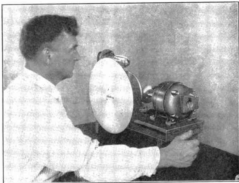
FIG. 324. Experimental Scanning Disc Arrangement and Driving Mechanism.
