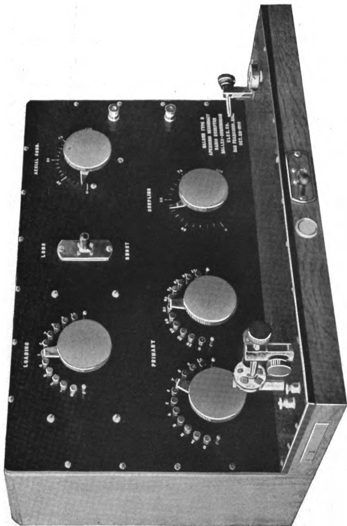
PLATE XXVIII. Short Wave Untuned Secondary Receiver. (Crystal Detectors.)
