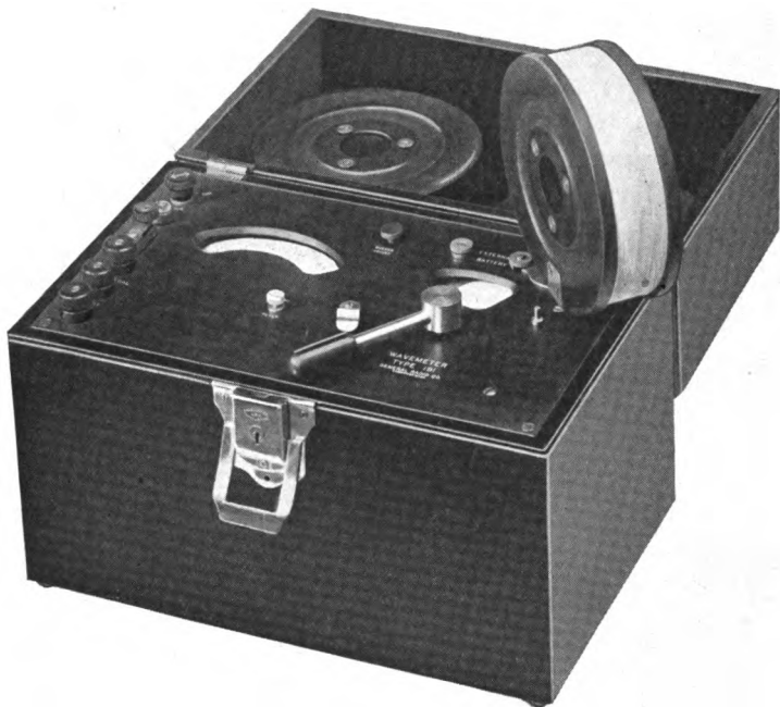
PLATE XX. Wave Meter and Decrometer.
