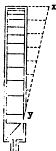
FIG. 5.—AMPLITUDE OF PRESSURE VARIATION IN A CLOSED ORGAN PIPE, INDICATED BY THE ORDINATES OF THE DOTTED LINE xy .
