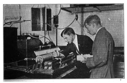
Fig. 4b-Scudents at Marconi School Measuring Wave Length With Fleming's Cymometer.
