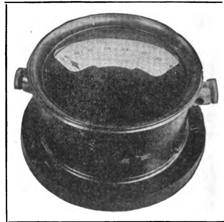
An aerial hot wire ammeter.
