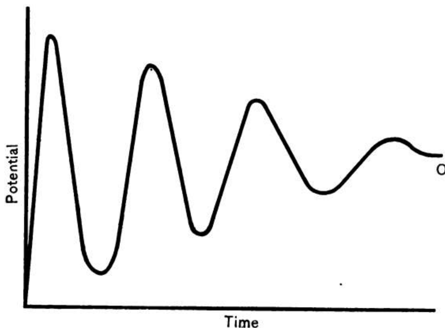
FIG. 17.—Electric Discharge through a Large Resistance.
