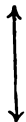
FIG. 52.—A Hertzian wave is plane-polarized, i. e., the vibration takes place always in one plane.
