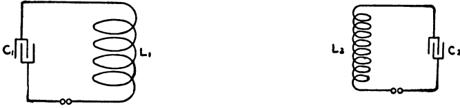
FIG. 126.— Two closed oscillating circuits with their capacities C_1 , C_2 , and inductances, L_1 , L_2 , so adjusted that the product L_1C_1 = L_2C_2 . The two circuits are then in tune.
