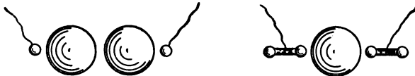
FIGS. 24 and 25.—Two forms of Lodge's oscillator. In the former the oscillations play across between the two middle spheres; in the latter, they surge, like tidal waves, over the surface of the large sphere.
