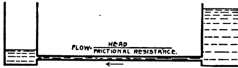
FIG. 4.— Ohmic resistance is analogous to friction of water flowing through a slender tube. The flow depends upon the difference in level, the bore of the tube and (inversely) on its length. The energy lost goes into heat.
