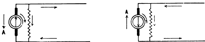
FIG. 193.—Shunt Generator and Motor.
