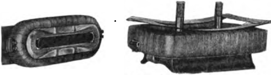
FIG. 147.—Interpole and Main Pole.
