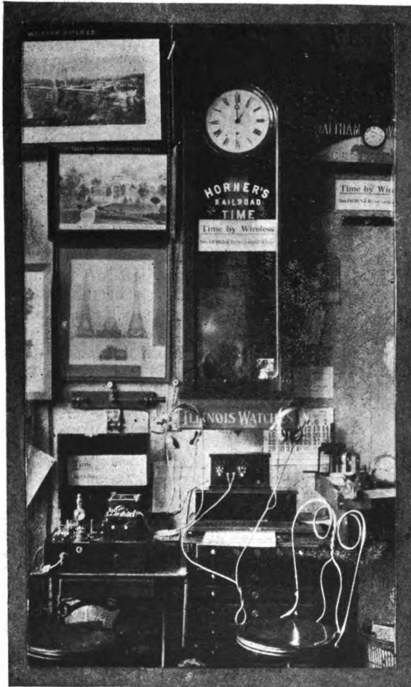
A Jeweler's amateur outfit used for receiving the time signals sent out daily from the high power naval stations
