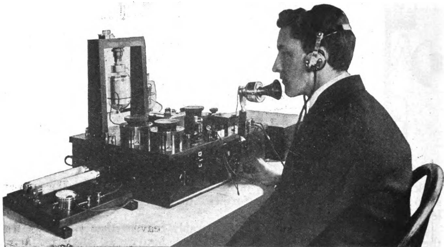
An early type of experimental wireless telephone using a vacuum tube
