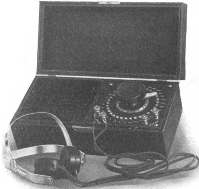
Fig. 238—Audibility Meter (American Marconi Company).
