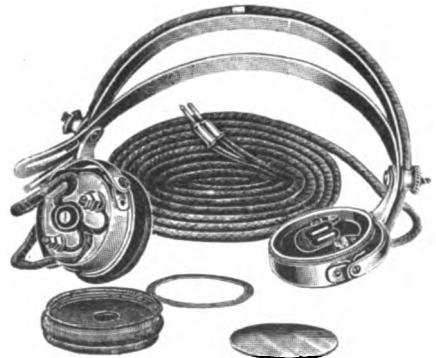
Fig. 194a—3 000-Ohm Head Telephone Receiver.
