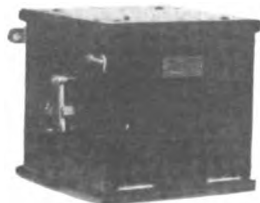
Fig. 269—Tuned Buzzer Tester.
