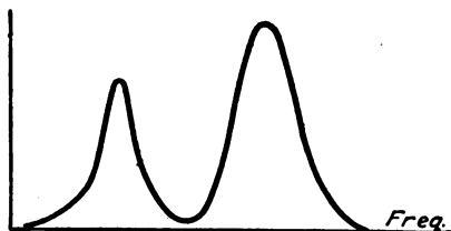
Fig. 48.—Resonance curve for circuits of Figs. 41 and 42.
