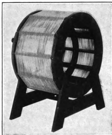
FIG. 216.— Multiple-layer standard coil
