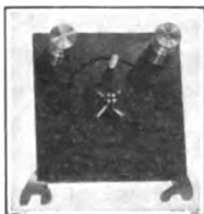
FIG. 111.—Mounted thermocouple with protecting cap removed
