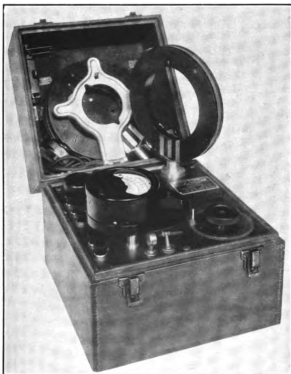
FIG. 218.—Exterior view of Kolster decremeter type D
