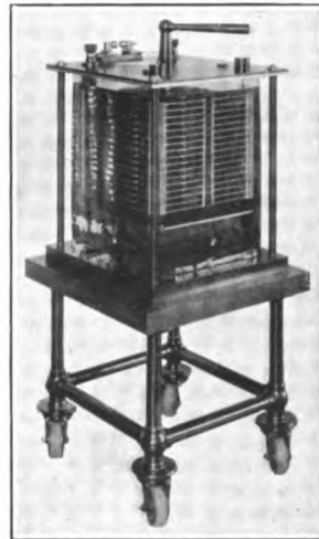
FIG. 85.—Type of variable condenser suitable for high voltages, with double set of semicircular moving plates
