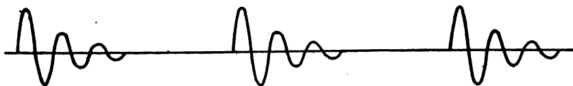
FIG. 68.—Series of wave trains similar to that generated by a damped wave source
