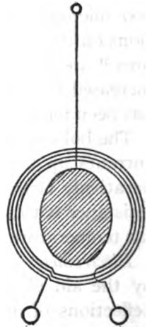
FIG. 117.—Type of electro-dynamometer suitable for radio current measurement
