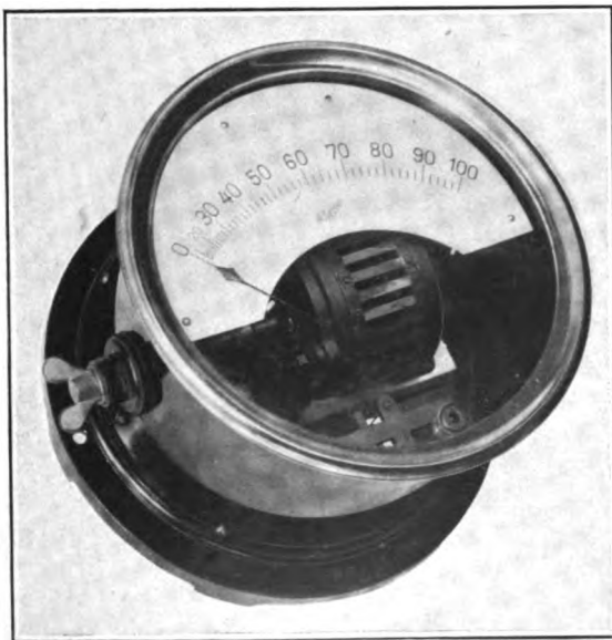
FIG. 102.—Hot-strip ammeter with cylindrical arrangement of heating elements
