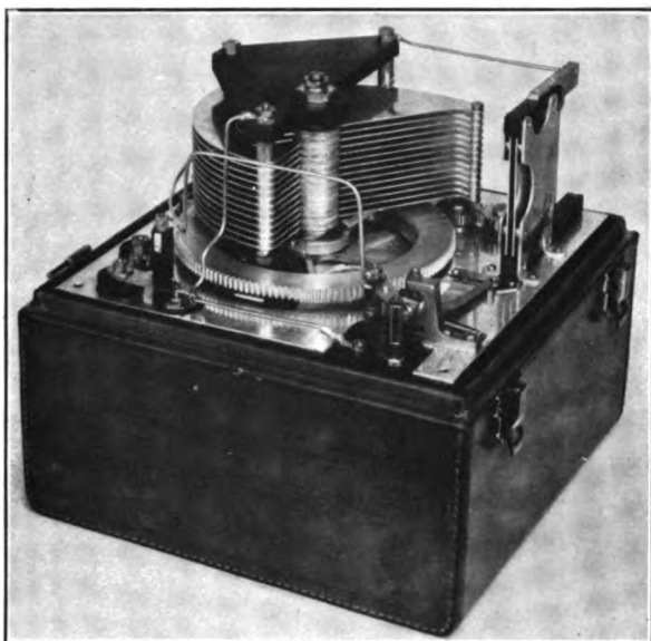
FIG. 217.—Interior view of Kolster decremeter type D
