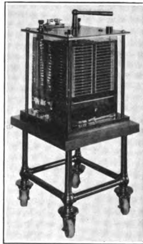
FIG. 85.—Type of variable condenser suitable for high voltages, with double set of semicircular moving plates
