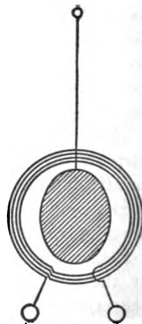
FIG. 117.—Type of electrodynamometer suitable for radio current measurement
