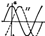
FIG. 4.—Graph of the electromotive forces in a quarter-phase alternator, plotted against time.
