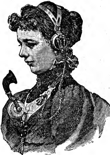
FIG. 40 OPERATOR'S SET (ERICSSON PATTERN)
