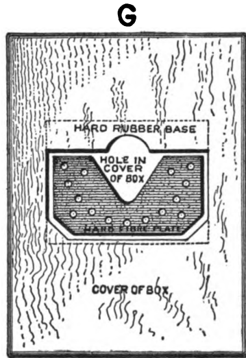
FIG. 84.—PLAN VIEW OF HARD FIBRE PLATE IN COVER OF BOX.
