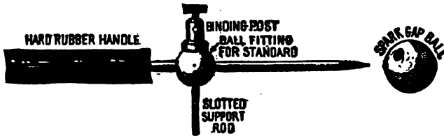
FIG. 102.—SPARK GAP TERMINAL WITH BALL DETACHED.
