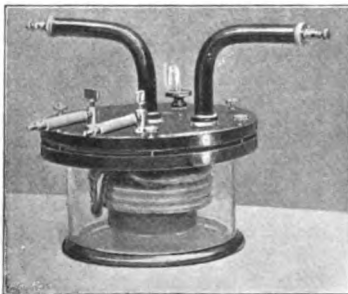
FIG. 52.—Oscillation Transformer in Transmitter Circuit. From "The Electrical Review."
