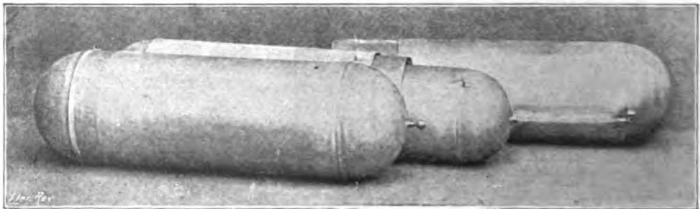
FIG. 56.—Balancing Capacities used instead of Earth Connections in Braun-Siemens Transmitter and Receiver.
