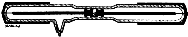
Fig. 40.—Metallic Filings Cymoscope used in Slaby-Arco Receiver.
