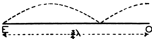
FIG. 5.—Distribution of Potential along a Finite Cable having a Simple Periodic E.M.F. placed at E ( First Harmonic Oscillation ).
