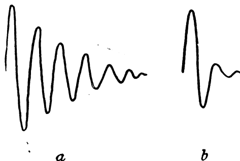
FIG. 8.—Oscillograph records of feebly damped (a) and highly damped (b) oscillations.
