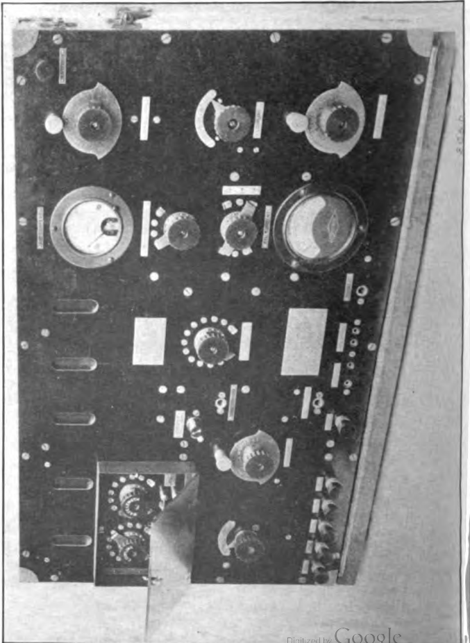
Operating Panel of Set Box Type BC-13 used in Set Type SCR-67 Showing Covered Panel Lid Partly Open.
