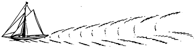
FIG. 33.—Echelon waves made by a model yacht.
