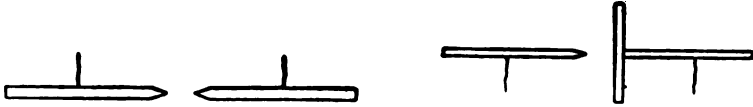
FIG. 41 a .—SPARK-GAP WITH POINTED ELECTRODES. FIG. 41 b .—SPARK-GAP WITH POINT AND DISK.
