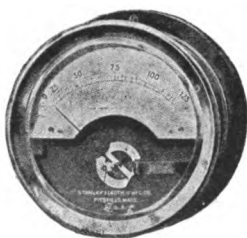
FIG. 64.—Hot-Wire Ammeter or Current Measurer.
