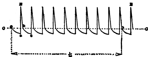
FIG. 33.—Diagram of Electric Impulses Delivered to Antenna by Induction Coil.
