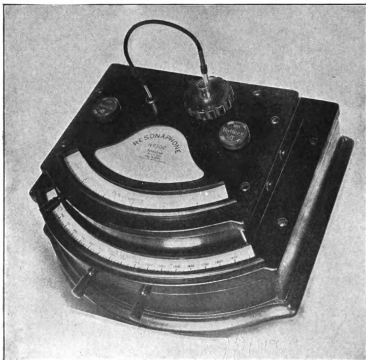
FIG. 13.—DETECTOR MOUNTED ON WAVE METER.
