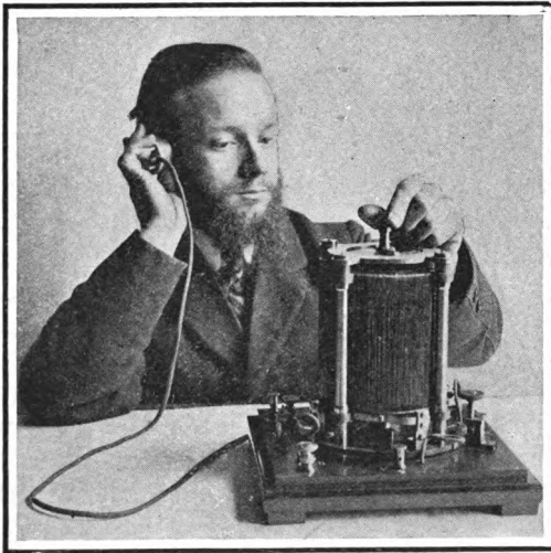
FIG. 97.—Bellini-Tosi radio-goniometer for directive wireless telegraphy.
