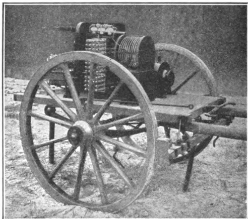
FIG. 101.—Telefunken wireless cart, showing transmitter.
