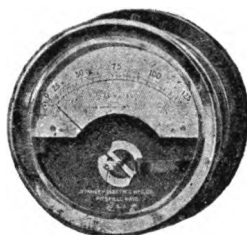
FIG. 64.—Hot-Wire Ammeter or Current Measurer.
