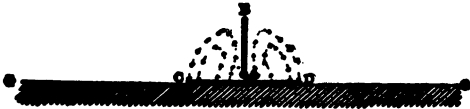
FIG. 13.—Electric Flux Induced by the Ring Distribution of Magnetic Flux in Fig. 12.
