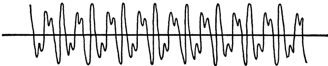
Fig. 5. Oscillogram of a Telephone Current
