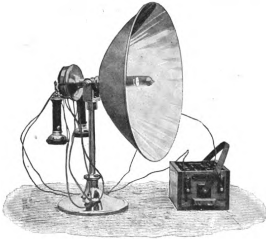
FIG. 50. Portable Photophonic Receiver.
