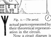
merely a collection of *theoretical signs* connected together by a series of lines representing connecting wires. These theoretical signs are stan-
