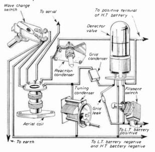
Fig. 63.—.4 typical detector stage in pictorial form.
