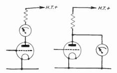
Fig. 30.—The working of a value stage may be checked in two different ways as shown here.
