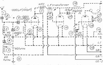
Fig. 20.—The circuit revised for applying bias to both L.F. stages. Tne solid lines show the additional wiring.
