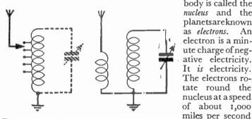
Fig. 34.—A simple aerial tuning circuit. Greater selectivity is obtained when a coupling coil is included and a tuning high speed condenser is employed.
