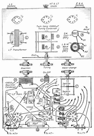
Fig. 74.—Top and underneath views of a receiver built to the circuit showing position of wires. The numbers on the circuit correspond to the numbers on the wiring diagrams.
