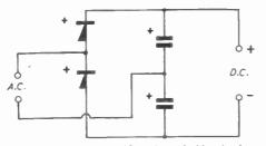
Fig. 99.-A metal rectifier voltage doubler circuit.
