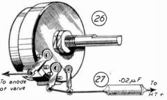
ted. By making Fig. 26.—The variable resistor and condenser necessary for adding tone control.
