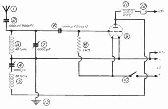
Fig. 1.—Circuit diagram of a simple one-valver for medium wavebands only. A pictorial diagram of the receiver built from this circuit is given on page 17 Where crossing lines are connected by a dot, they are to be joined by solder, or connected to a terminal.
