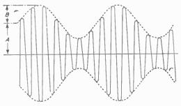
Fig. 52.—The form of the modulated carrier wave.
