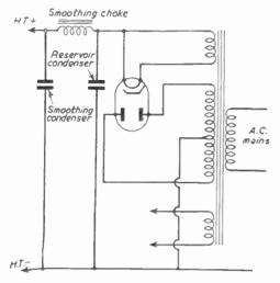
In order to ascertain the most suitable size of stamping, it is necessary to know the power, in watts, which the transformer has to handle. For example, assume that the transformer has to supply 20 volts at 2 amperes; the wattage would be 20 multiplied by 2, or 40 watts, assuming an effi-
