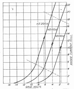
crease in grid bias. In this case Fig. 22.—Typical characteristic curve of an amplifying valve, showing the variation in grid bias resulting from variation in H.T. voltage. be referred to as 2 milliamps. per volt or, as it is expressed on the valve chart, 2mA/V.
