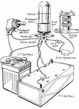
Fig. 65.—Battery connections.
