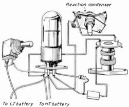
Fig. 66.—The reaction circuit.
