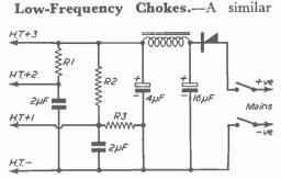
state of affairs exists with regard to low-frequency chokes, for one which is rated at, say, 20 henries would have an approximate D.C. resistance of 250 ohms. But the impedance of the choke to an alternating current of 50
