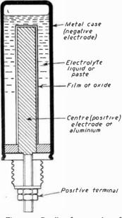
Fig. 49.—Details of construction of a typical "wet" electrolytic condenser.
