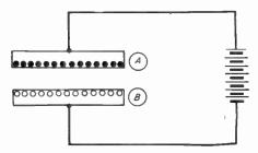
Fig. 39.-Dielectric strain in charged condenser.
