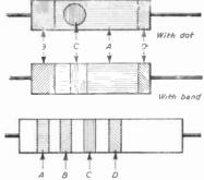
In older resistances it will be found that the body of the Fig. 29a.—The colour code diagram.
