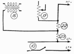
Fig. 23.—Modified circuit for providing automatic grid bias.
