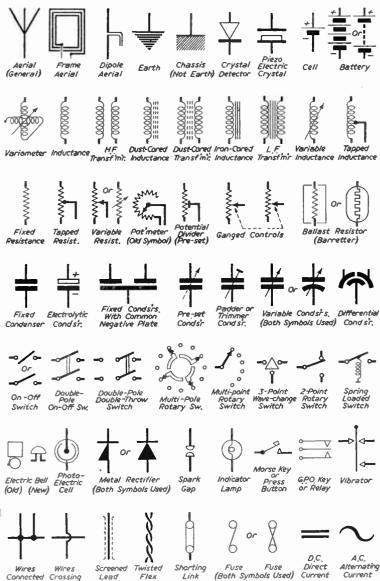
Conventional signs used in drawing a wireless circuit, which merely consists of a number of these signs joined together. Pictorial diagrams showing the actual components represented are given in the book in their correct alphabetical order.
