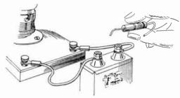
Fig. 82.—Measuring resistances by the flash method.
