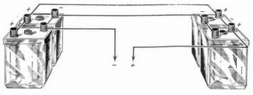
Fig. 103—Accumulators [in parallel.
