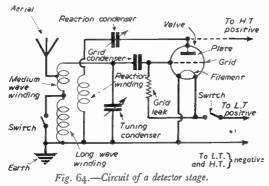
that when the current in the aerial circuit flows one way it reduces the plate current and when the aerial current flows in the other direction the opposite happens.
