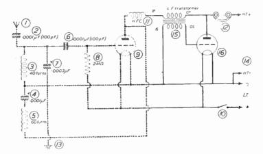
Fig. 13.—Theoretical circuit of a two-valve receiver, which is modified from the one-valve circuit given in Fig. 1. The one-valve circuit is shown by means of dotted lines. The new wires and additional components are shown by solid lines. The only additional components are shown by solid lines. The only additional parts are a low-frequency transformer, a valve and c-valve holder (parts 15 and 16).
