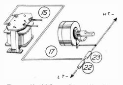
positive than at the upper end where it joins H.T. -. Therefore, the point to which the first grid circuit is connected (the L.F. transformer secondary) is at a lower negative voltage than the point to which the end of the volume control is connected. With the cur-
