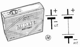
Fig. 11.—The theoretical signs for low tension (L.T.)and high tension (H.T.) batteries. Note that the thin line always represents the positive terminal, and the thick line the negative terminal. On the left is a pictorial view of an all-dry combined L.T. and H.T. battery, but in most cases the accumulator is of the wet type: that is to say it contains dilute sulphuric acid and can be recharged.
