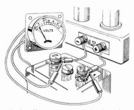
ment noted. The coils which are to be compared can then be connected in circuit, one at a time, and the reading carefully noted in each case. In each instance, the efficiency of the coil is represented by the change in anode current when it is in circuit.
