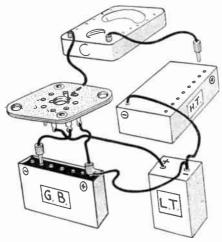
Fig. 88.—Set-up for taking valve measurements.
