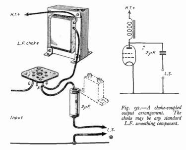
There are two types of output filters—the output choke and the transformer.
