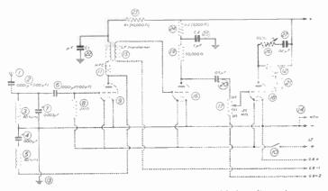
Fig. 25.—The three-value circuit shown by Fig. 20 with decoupling resistances and condensers and tone control added.
