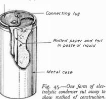
Direct Anode Bypass Condenser,  $0001-0005 \ \mu\text{F}$ . Resistance-capacity Coupling Condenser,  $011-\mu\text{F}$ . Decoupling Condenser H.F. (M.W., L.W. and S.W.),  $1-1 \ \mu\text{F}$ , U.S.W.  $001 \ \mu\text{F}-11 \ \mu\text{F}$ . Decoupling Condenser (L.F.),  $2-8 \ \mu\text{F}$ . Smoothing Condenser (Mains Unit),  $2-60 \ \mu\text{F}$ .
