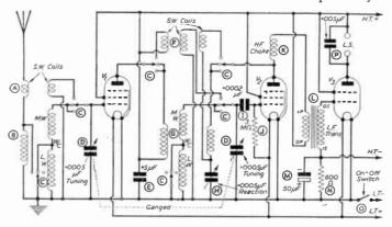
Fig. 73.—Theoretical circuit of a modern three-value receiver.
