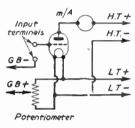
Using Valve Voltmeter.—In H.T.- using a valve voltmeter adjust the grid-bias voltage by altering the position of the negative tapping and by varying the potentiometer setting LT+ until the milliammeter shows a reading of about .5 milliamps. When that is done, any tuned circuit which is connected to aerial and earth lead can be connected to the two termin-
