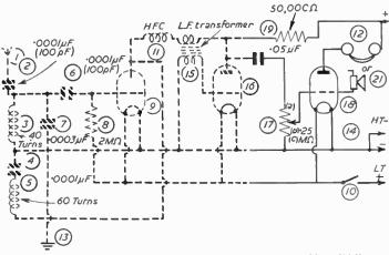
Fig. 18.—Theoretical circuit of the three-value arrangement. The solid lines show the wiring for the additional stage.
