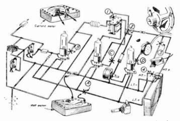
Fig. 31.—The three-value receiver circuit in pictorial form showing the points to which meters are joined for testing.
