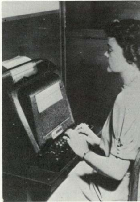
Fig. 9-3. One of three operator stations for the Model I, also known as the complex number computer. [Tropp, IEEE Spectrum 11 (1974): 70.]
