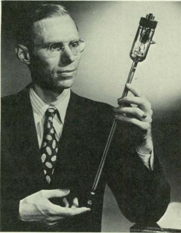
Fig. 5-12. J. R. Pierce with the traveling wave tube of 1946. In addition to his pioneering contributions to traveling wave research, Pierce made fundamental contributions to satellite and digital communications research.
