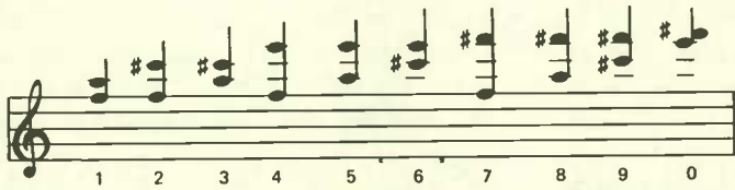
Fig. 1-25. The two-out-of-five code was invented for tone signaling between telephone offices. The ten possible combinations of five basic tones (F, A, C # , E, F # ), taken two at a time, represent the ten digits 1, 2, . . . , 0. The code is error-detecting because reception of numbers of tones different from two can only result from a transmission error. More elaborate codes can correct errors as well as detect them.
