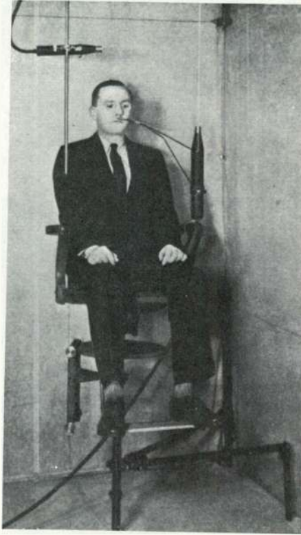
Fig. 2-6. H. K. Dunn conducting acoustic measurement of the sound field around a talker's head. [Dunn and Farnsworth, J. Acoust. Soc. Am. 10 (1939): 186.]
