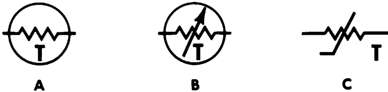
Fig. 2-5. Temperature compensating resistor symbols.
