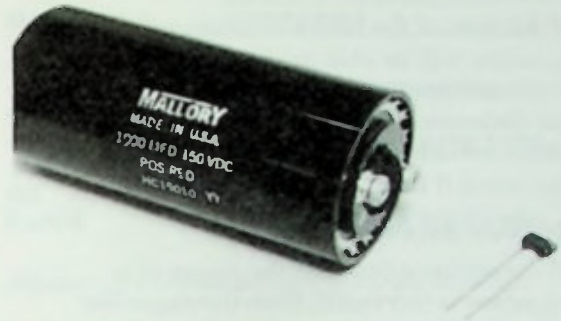
Figure 6.11 Typical Small-Value and Large-Value Capacitors
