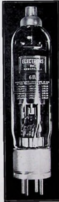
FIG. 8.7. A type EL6B gas rectifier tube. (Courtesy Electrons, Inc.)
