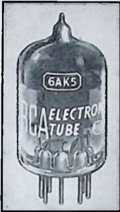
FIG. 4.5. A miniature pentode designed for television amplifier service. (Courtesy RCA.)
