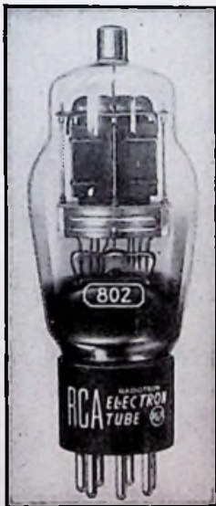
FIG. 4.7. A low-power transmitter pentode designed for oscillator and amplifier service. (Courtesy RCA.)
