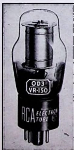
FIG. 7.3. A voltage-regulator tube. (Courtesy RCA.)
