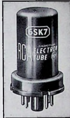
FIG. 4.6. A metal-envelope pentode designed for radio-frequency voltage-amplifier service. (Courtesy RCA.)
