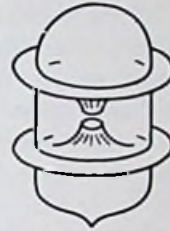
FIG. 7.4. A T-R (transmit-receive) tube used in radar systems.
