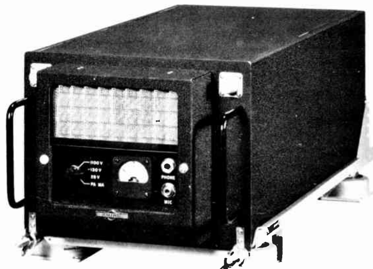
Collins 618T Single Sideband Transceiver Provides Communication on All Aeronautical Bands in the 2 to 30 Mc Range with 400 Watts PEP
