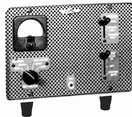
Figure 13-19. 312B-4 Station Control
