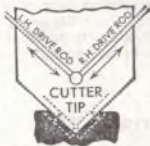
Fig. 4. How a stereo disc is cut
