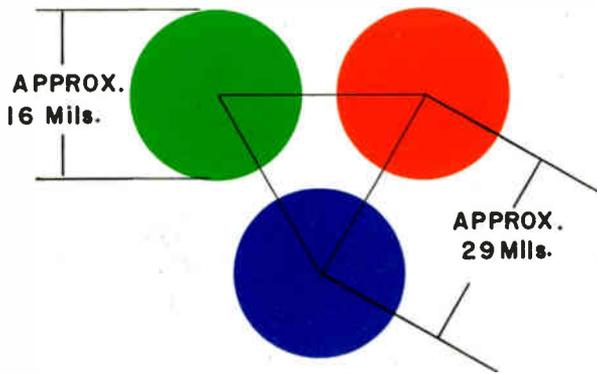
Figure 5-7. Phosphor dot triad.
