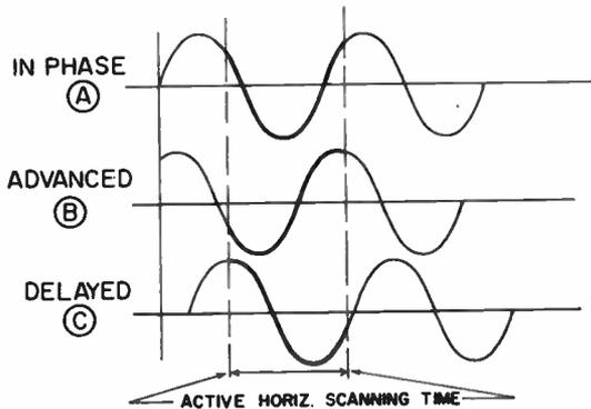
Figure 5-52. Relation of horizontal dynamic convergence voltage to active horizontal scanning time.
