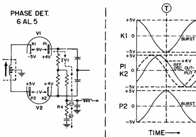
Figure 4-27. Phase detector in unbalanced condition.
