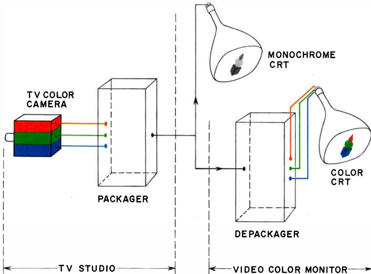
Figure 3-4. Composite color signal and compatible monochrome signal are developed from the primary color signals.
