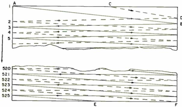
Figure 1-3. Beam pattern for interlace scanning
