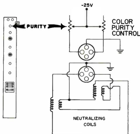
Figure 6-10. Color purity control, location and circuitry.
