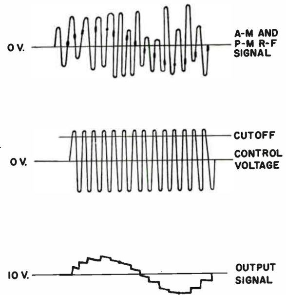
Figure 4-15. Detecting an amplitude-and phase-modulated signal.
