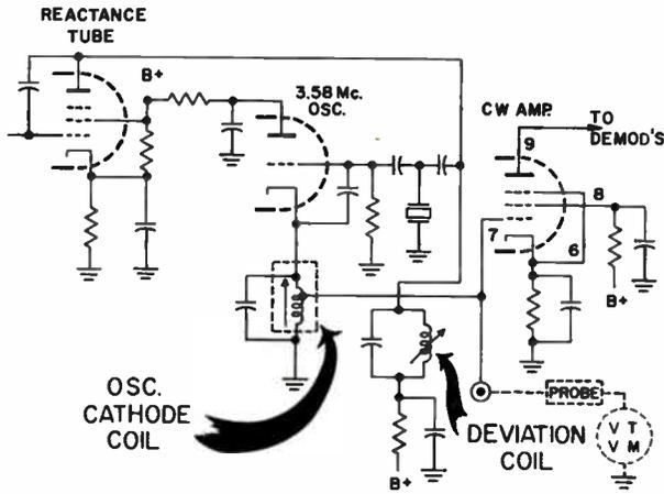
Figure 7-15. 3.58-mc oscillator adjustment.
