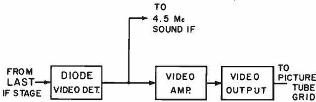
Figure 1-9. Video circuits, block diagram
