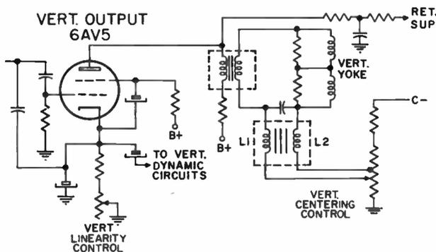
Figure 4-34. Vertical output stage.
