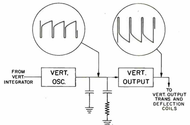
Figure 1-18. Vertical deflection circuits
