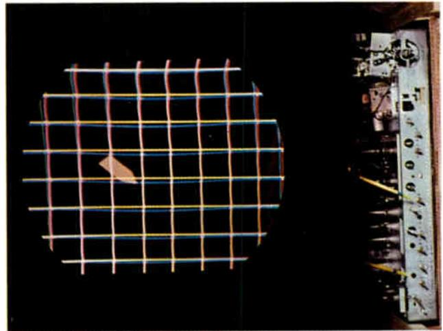
Figure 6-23. Adjustment of blue horizontal dynamic phase control.
