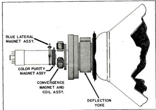
Figure 5-35. Location of electron beam deflection assemblies.
