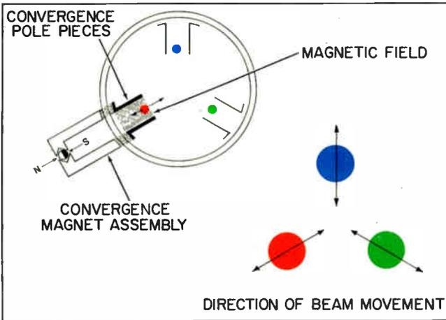
Figure 5-18. Deflection of electron beams by convergence assembly.
