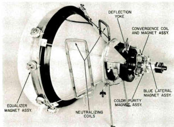
Figure 6-1. Adjustments for color cathode ray tube assembly.
