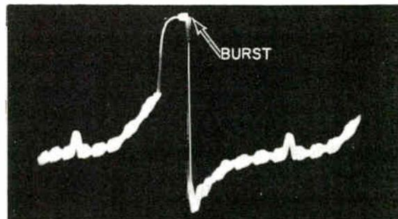
Figure 8-29. Burst amplifier input signal.
