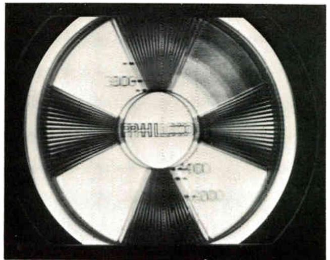
Figure 8-9. Phase distortion of the monochrome test pattern caused by a defective delay line.
