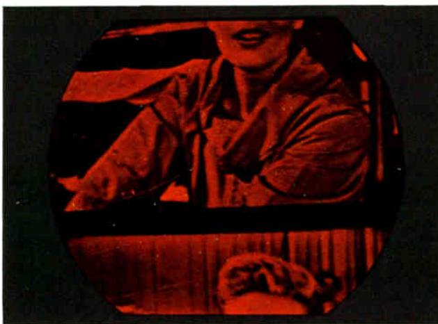
Figure 6-48. Adjustment of red G2 control.
