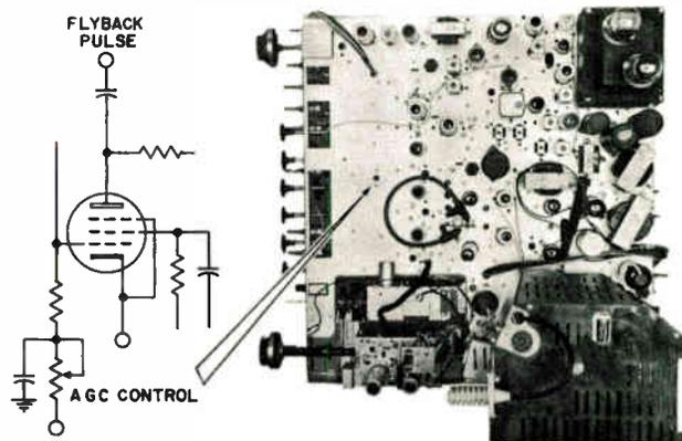
Figure 6-4. AGC control, location and circuitry.
