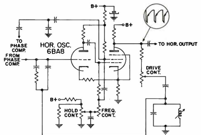
Figure 4-39. The horizontal oscillator.
