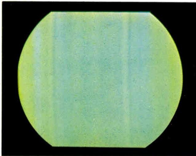
Figure 8-24. Color-bar presentation when common cathode resistor is open.
