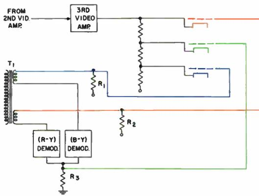
Figure 4-23. Applying the color-difference signals to the cathode ray tube.
