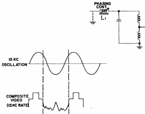
Figure 5-51. Horizontal dynamic phasing control circuit.
