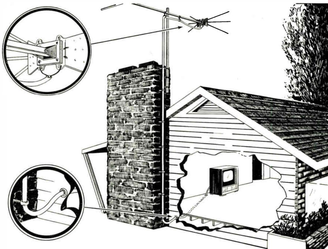
Figure 9-13. Home installation of antenna and lead-in.
