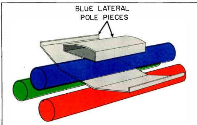
Figure 5-20. Blue beam lateral pole pieces.
