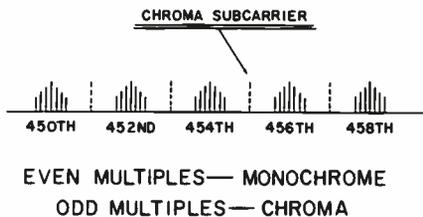
Figure 3-39. Grouping of video signal about harmonics of one-half horizontal line frequency.
