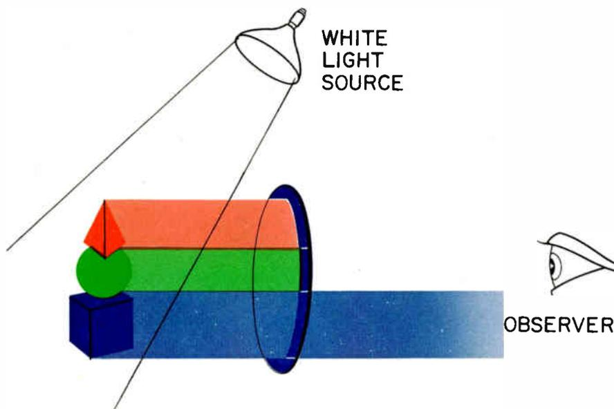
*Figure 2-13. Separating reflected light*
