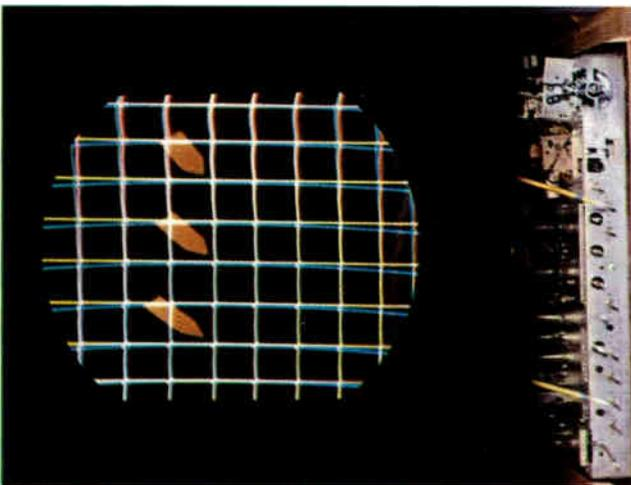
Figure 6-19. Adjustment of blue vertical dynamic amplitude control.
