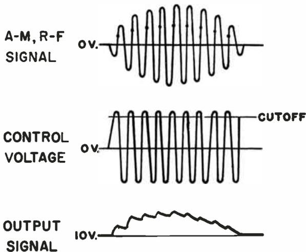
Figure 4-14. Detecting an a-m, r-f signal at a relative phase angle of 30°.
