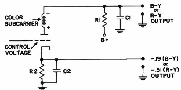
Figure 4-17. Obtaining the G-Y color-difference signal.
