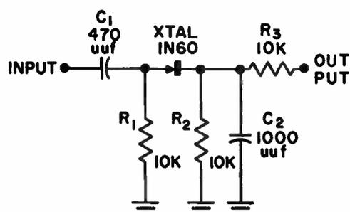
Figure 7-4. Low-impedance detector.
