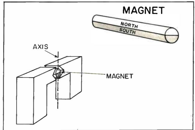
Figure 5-17. Convergence magnet assembly.
