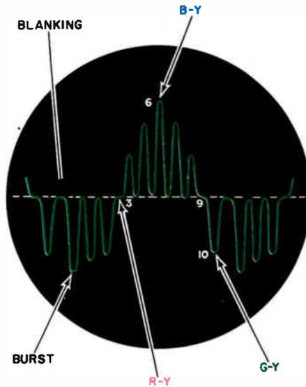
Figure 7-22. Oscilloscope waveform, grid of CRT blue gun, with color-bar-generator signal.
