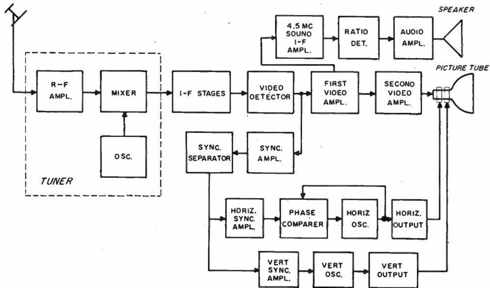
Figure 1-4. Intercarrier television receiver, typical block diagram
