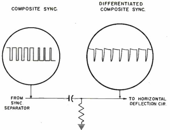
Figure 1-17. Differentiator circuit
