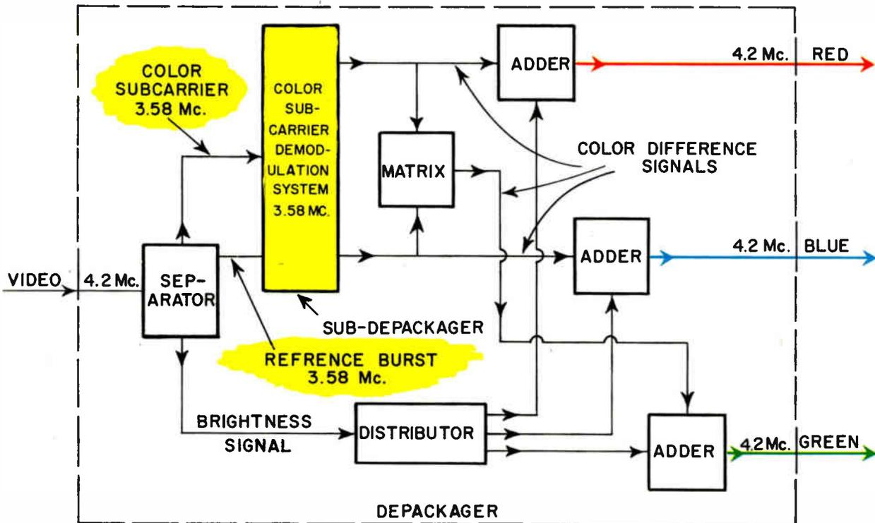
Figure 3-6. Reception of the composite color signal.
