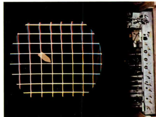
Figure 6-25. Final red, green, blue static convergence of preliminary convergence procedure.
