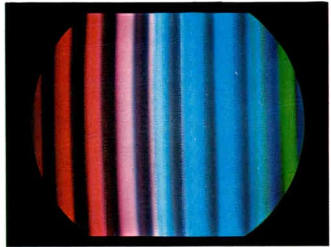
Figure 8-8. Color-bar pattern when luminance signal is missing.
