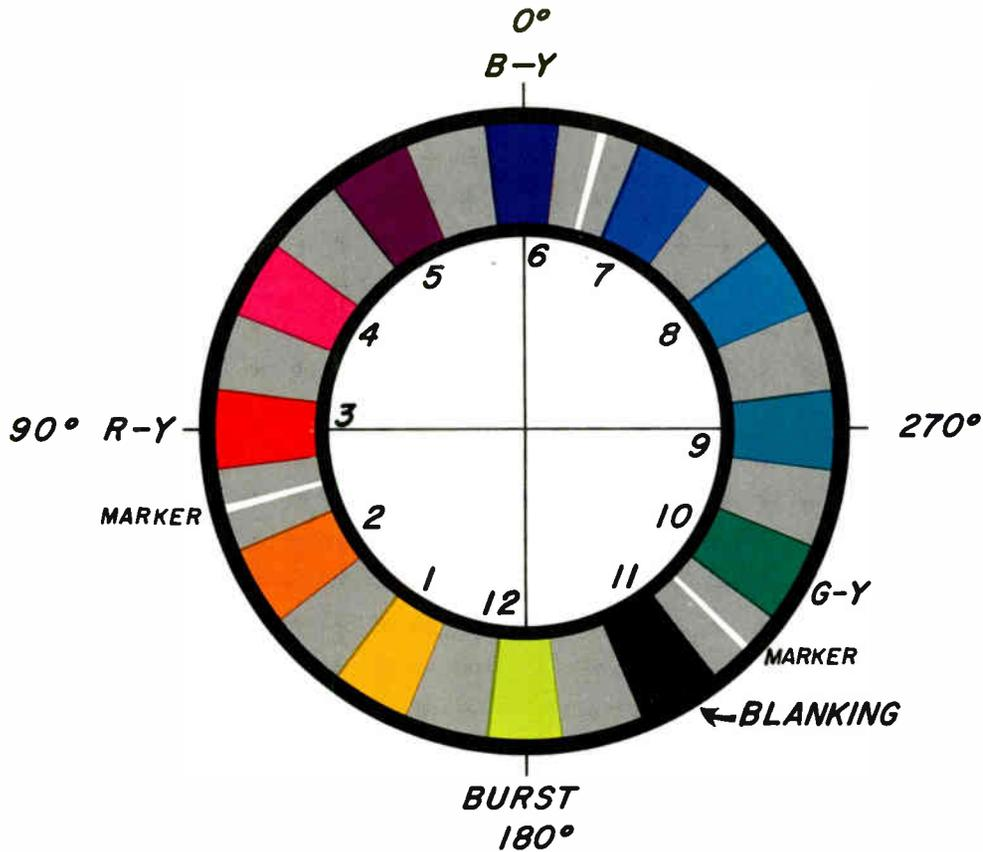
Figure 7-21. Color-bar-generator quadrature graph for quadrature adjustment.
