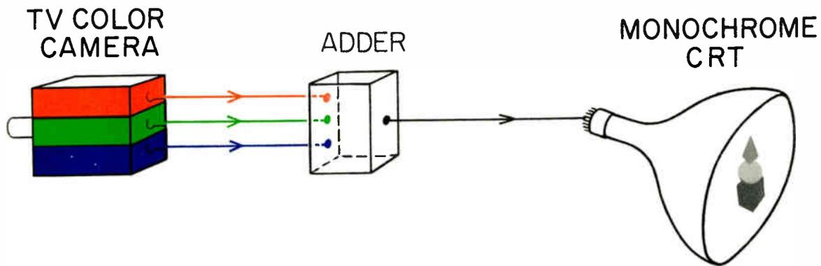
Figure 3-2. Forming the brightness signal.
