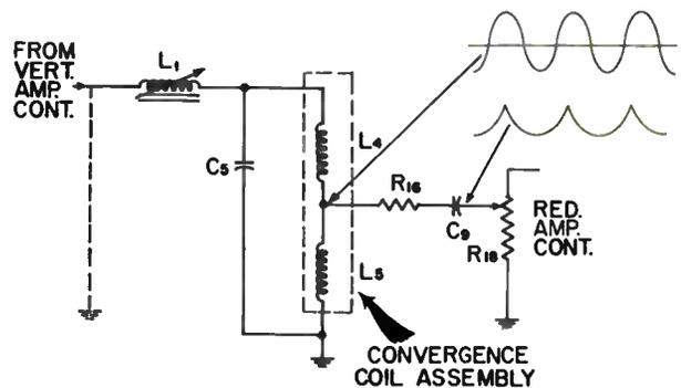
Figure 5-50. Development of horizontal dynamic convergence voltage.
