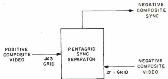
Figure 1-13. Sync separator and noise clipper
