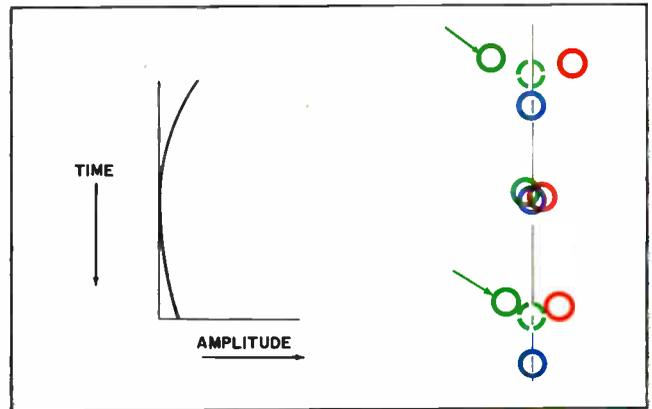
Figure 5-28. Vertical dynamic convergence of green beam.
