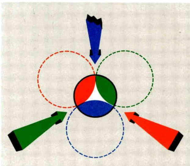
Figure 5-9. Principle of shadow mask operation.
