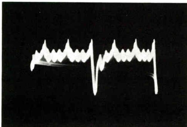
Figure 8-17. Waveform of bar pattern at plate of the chroma and sound detector.
