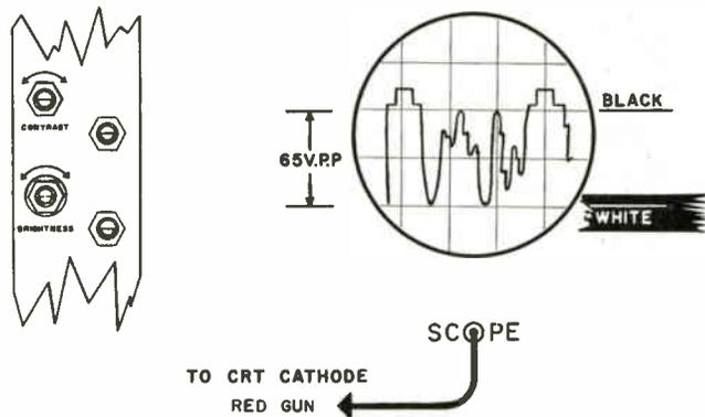
Figure 6-47. Pre-white balance adjustment of brightness and contrast controls.
