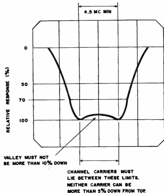
Figure 7-8. Typical tuner response curve.
