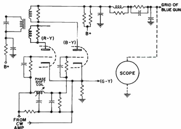
Figure 7-20. Circuit diagram, quadrature adjustment.
