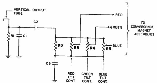
Figure 5-47. Vertical dynamic tilt control circuit.
