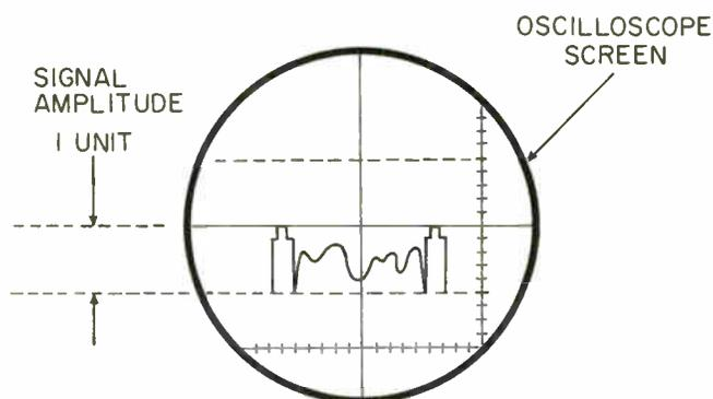
Figure 8-10. Video signal on cathode of blue gun.
