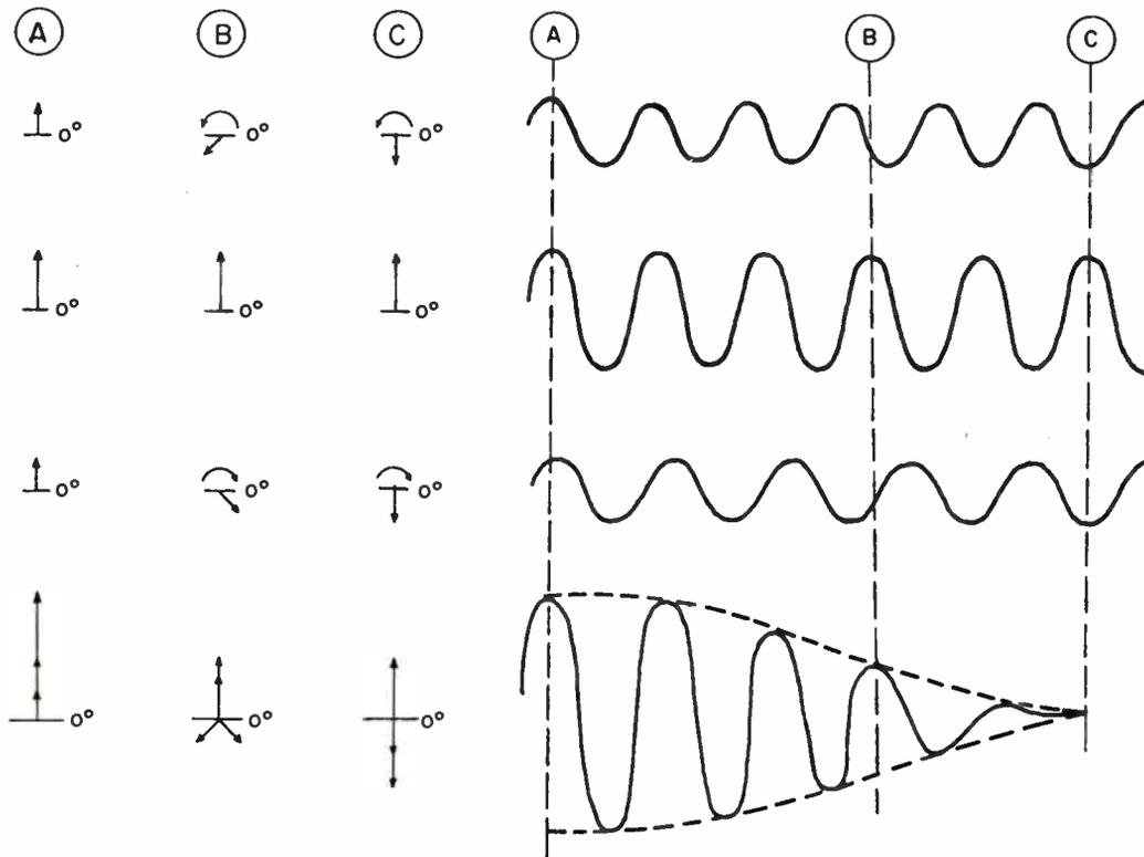
Figure 3-19. Forming the modulation envelope from the carrier, the upper sideband and the lower sideband.
