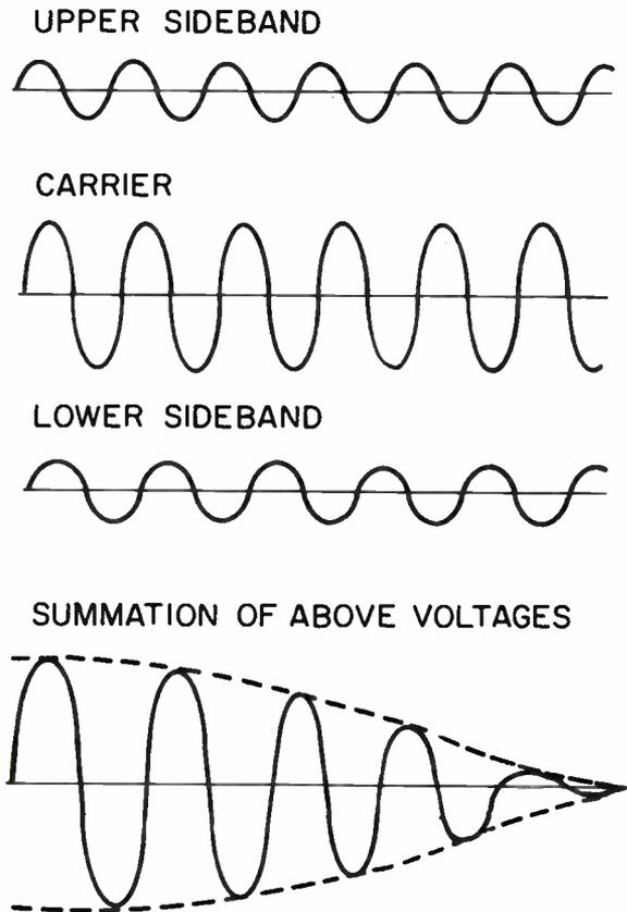
Figure 3-17. The amplitude modulated signal.
