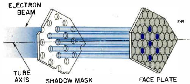
Figure 5-10. Paths of electron beams through shadow mask.
