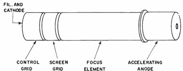
Figure 5-2. Electron gun assembly.
