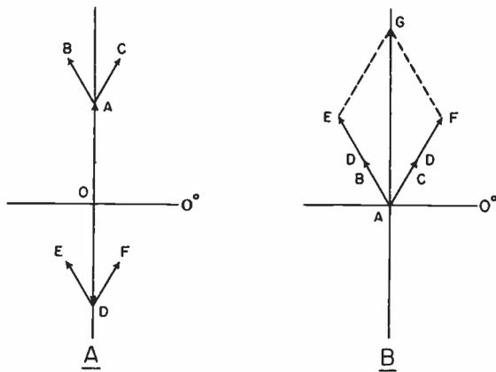
Figure 3-21. Voltage relationship of the suppressed-carrier modulation system at time A.
