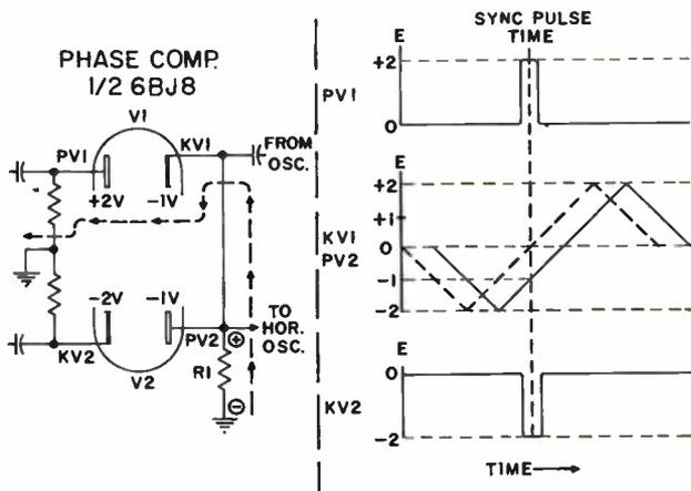
Figure 4-38. Oscillator frequency lower than sync pulse frequency.
