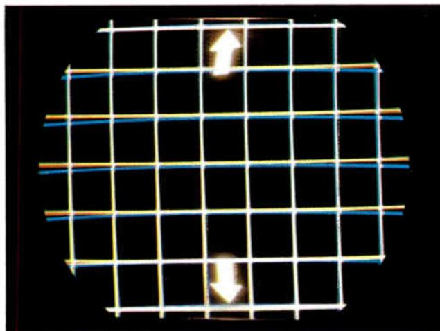
Figure 6-37. Adjustment of blue vertical tilt control.
