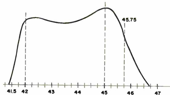
Figure 7-12. Overall response, chroma and sound detector output.
