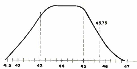
Figure 7-11. Overall response, video detector output.
