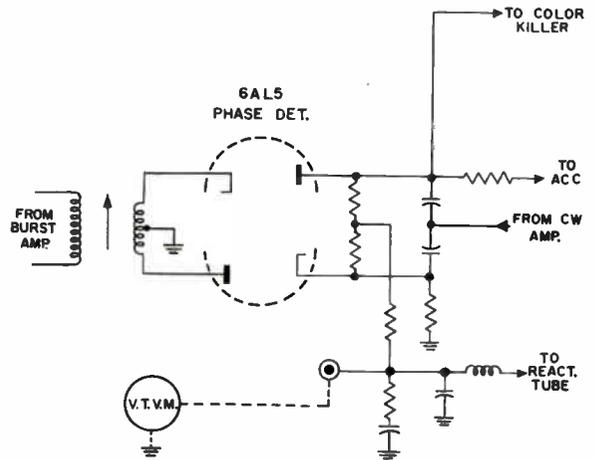
Figure 7-23. Checking the phase-detector circuit for balance.
