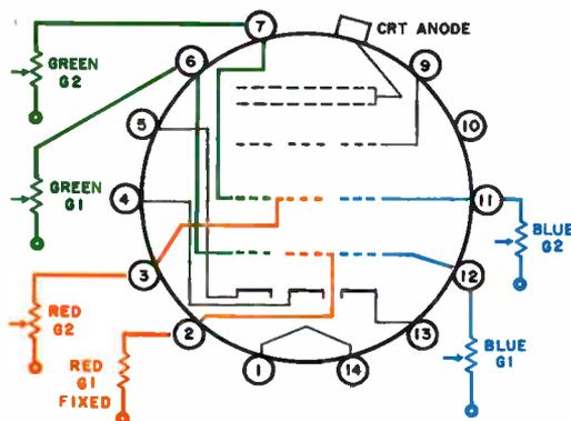
Figure 6-3. G1 and G2 control circuitry.
