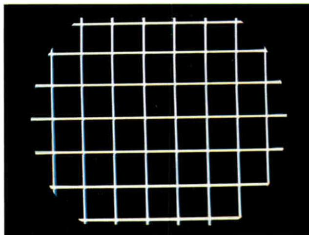
Figure 6-45. Overall convergence of the red, green and blue beams.
