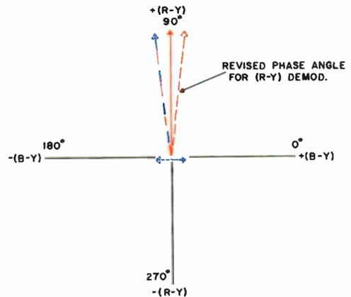
Figure 4-20. Revised phase angle for the  $R-Y$  demodulator.
