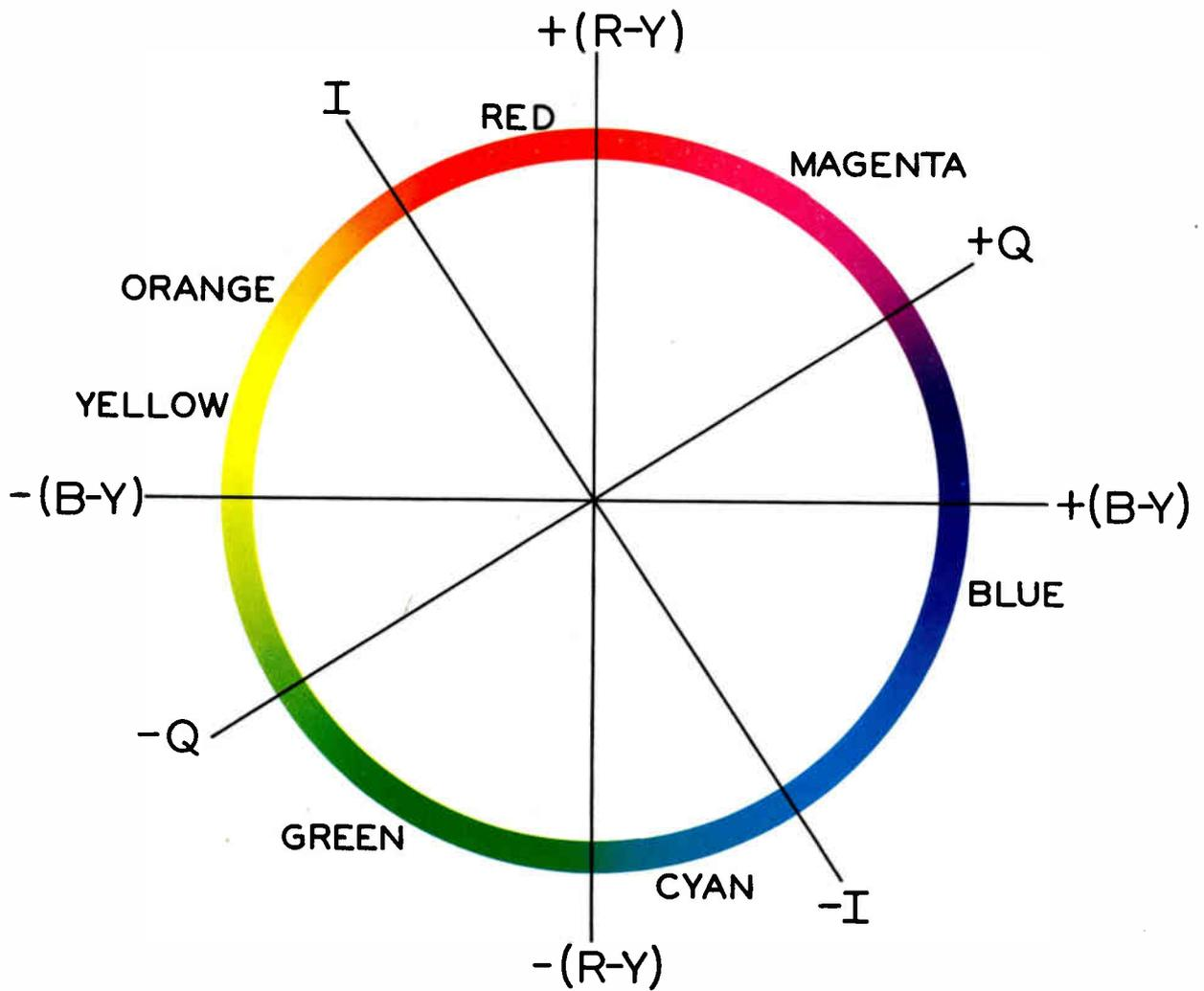
Figure 3-36. Relationship of I-Q co-ordinates and (R-Y)-(B-Y) co-ordinates indicating the colors associated with each color-difference signal.
