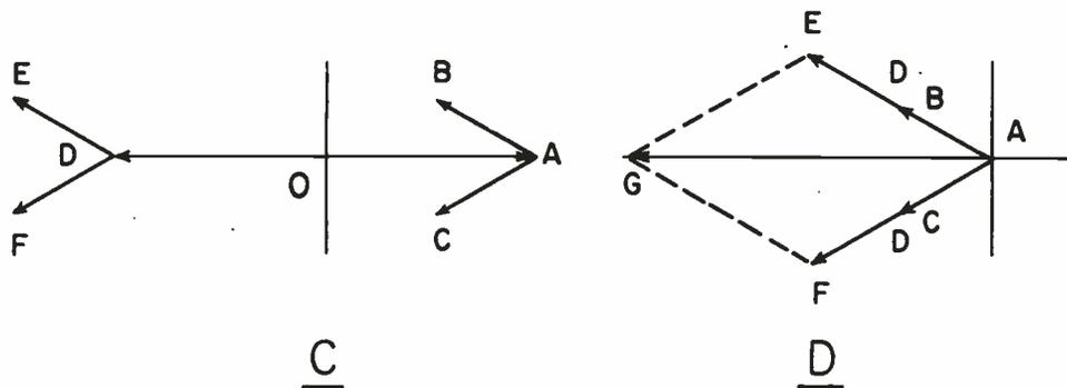
Figure 3-25. Voltage relationship of the suppressed-carrier modulation system with delayed carrier at time B.
