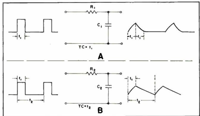
Figure 5-40. Effect of time constant to sawtooth output.
