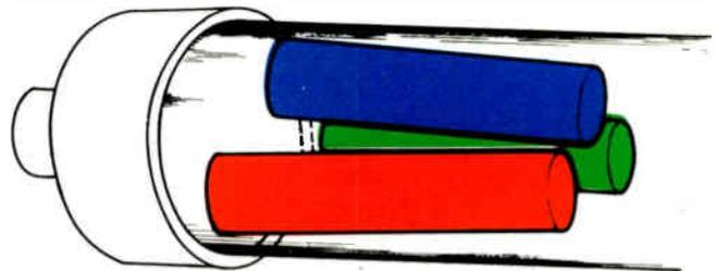
Figure 5-5. Axial tilt of electron guns.
