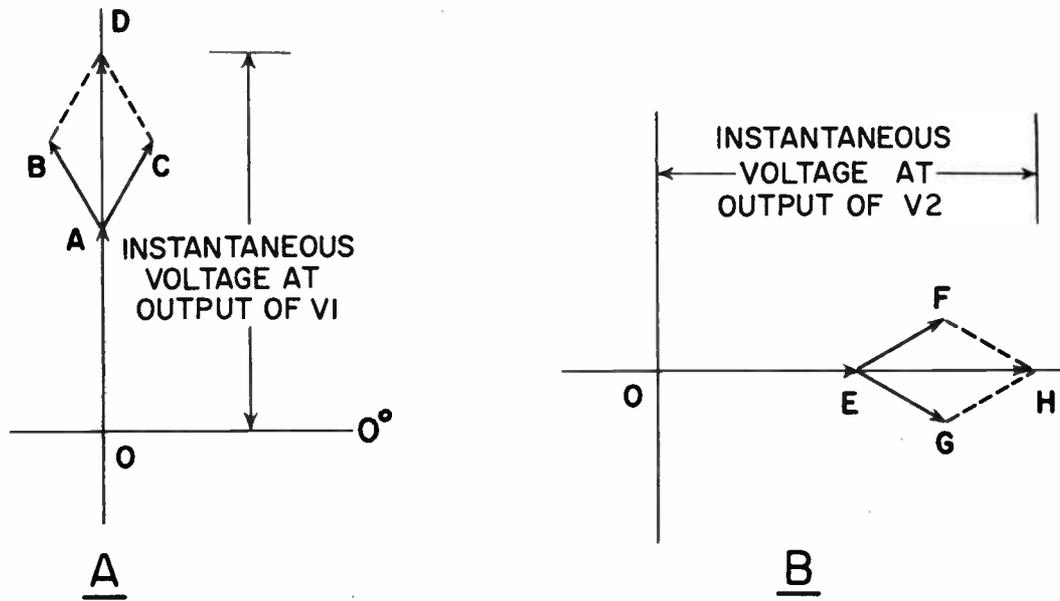
Figure 3-29. Voltage relationship of the color-subcarrier demodulator.
