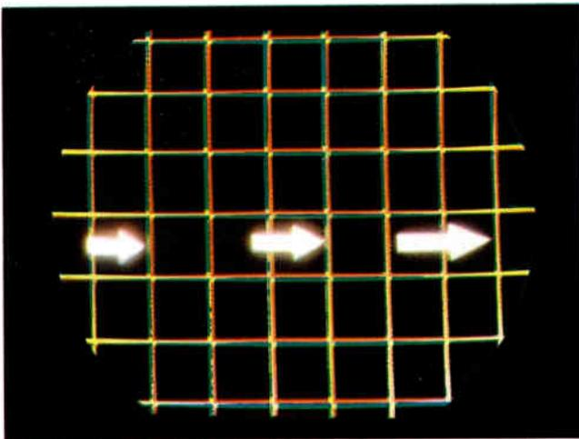
Figure 6-41. Adjustment of green horizontal phase control.
