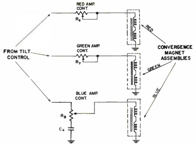
Figure 5-48. Vertical dynamic amplitude control circuit.
