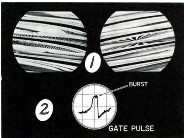
Figure 6-15. Horizontal frequency and burst timing adjustments.
