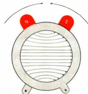
Figure 5-13. Adjustment of color purity magnet assembly.
