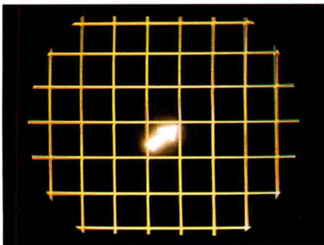
Figure 6-36. Static convergence of the red and green beams at center of screen.
