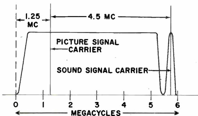
Figure 1-1. Composite television signal
