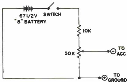
Figure 7-2. Bias supply circuit.
