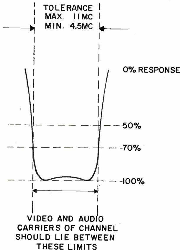
Figure 1-5. R-F response curve with bandpass limits
