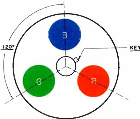
Figure 5-4. Relative position of electron guns.
