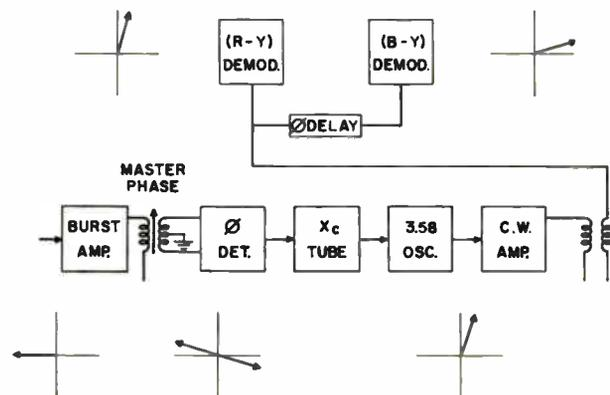
Figure 4-22. Phase angles of the burst and the R-Y and B-Y carriers.
