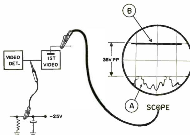
Figure 6-46. Adjustment of agc control
