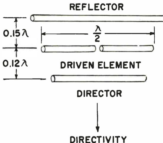
Figure 9-9. Physical arrangement of a three-element parasitic array.
