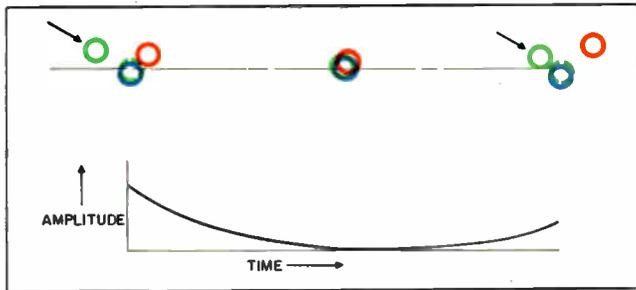
Figure 5-32. Horizontal dynamic convergence of green beam.
