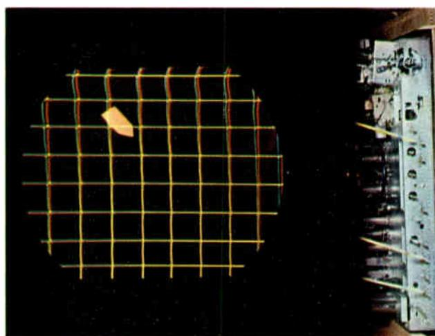
Figure 6-17. Adjustment of red and green vertical dynamic amplitude controls.
