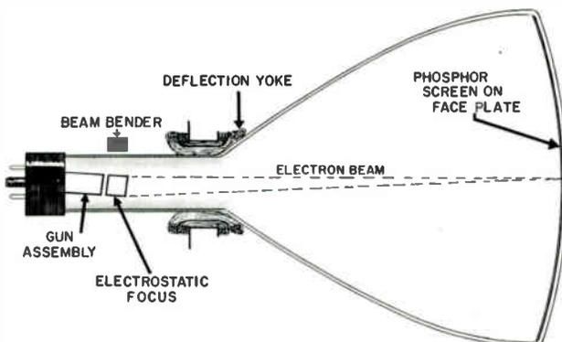
Figure 5-1. Monochrome cathode ray tube.
