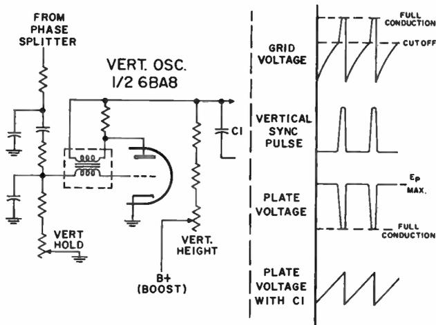
Figure 4-33. Vertical oscillator.
