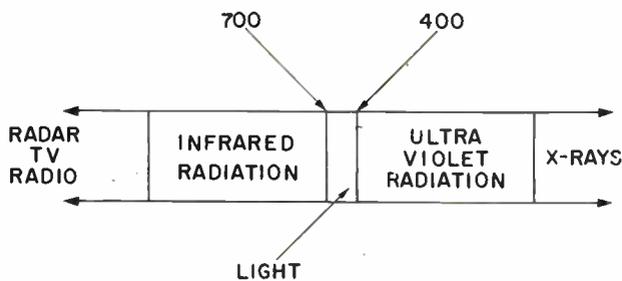
Figure 2-1. Frequency spectrum
