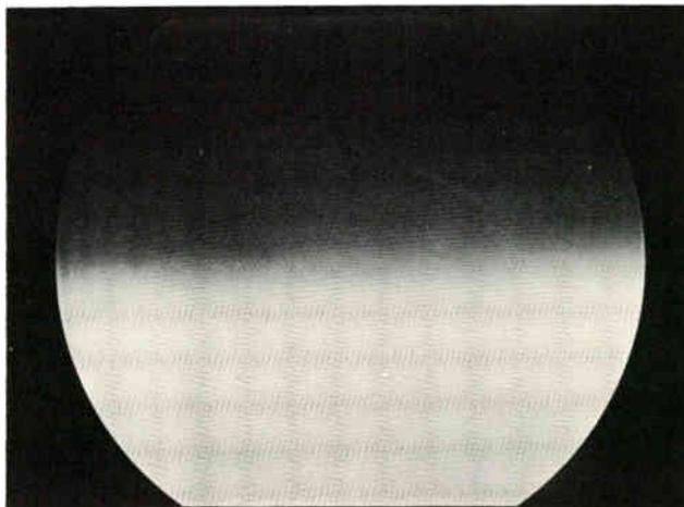
Figure 6-50. Adjustment of blue G1 and G2 controls for final white balance.
