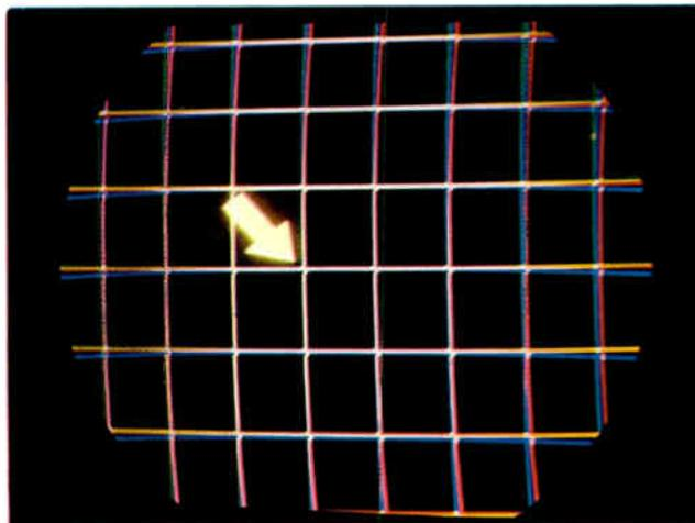
Figure 6-30. Static convergence of red, green and blue beams.
