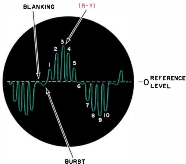
Figure 7-19. Oscilloscope waveform, grid of CRT red gun with color-bar-generator signal.
