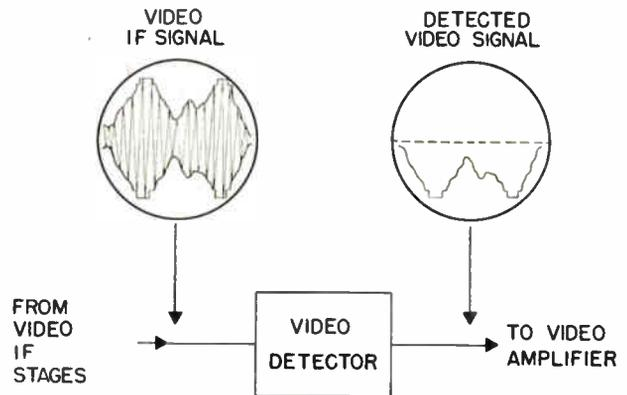
Figure 1-8. Input and output waveforms of video detector
