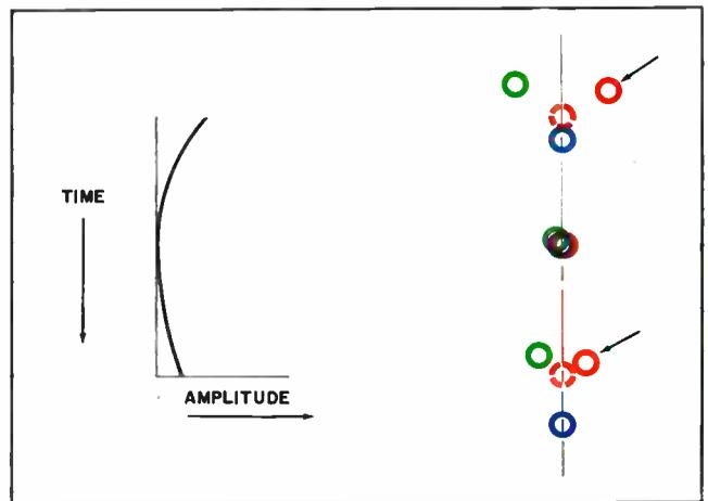
Figure 5-29. Vertical dynamic convergence of red beam.
