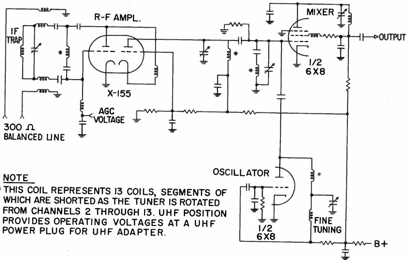
Figure 4-2. Simplified schematic diagram of a tuner.
