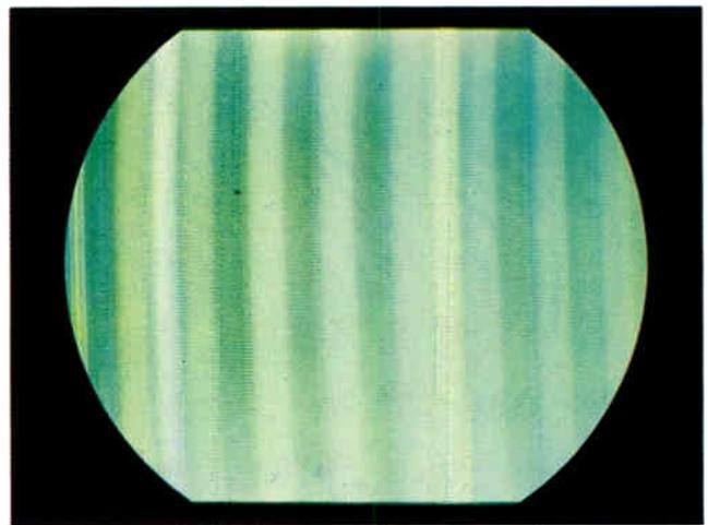
Figure 8-22. Color-bar presentation when bias on the grid of the green electron gun increases.
