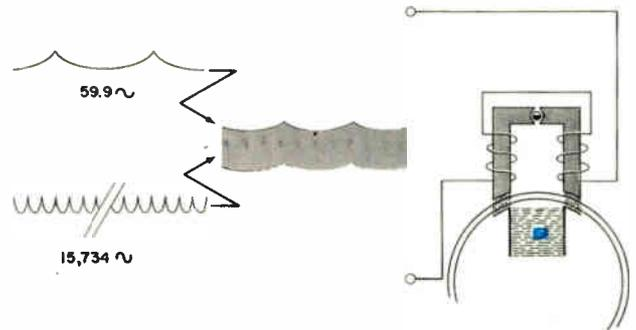
Figure 5-53. Dynamic convergence assembly and applied voltages.
