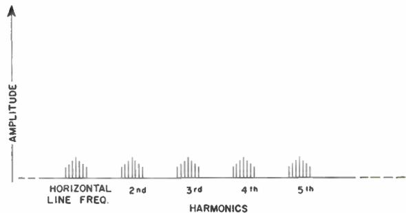
Figure 3-38. Grouping of video signal about horizontal line frequency and harmonics.
