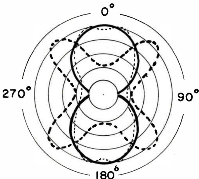
Figure 9-7. Field pattern of channel 3 dipole used for channels 3, 6 and 10.
