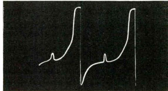
Figure 8-28. Gate clamp output signal.
