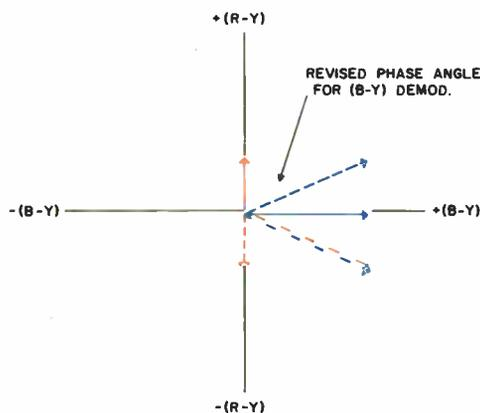
Figure 4-21. Revised phase angle for the B-Y demodulator.
