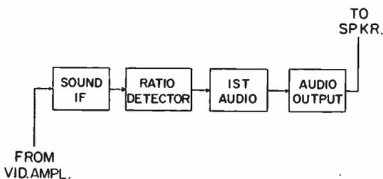
Figure 1-10. Audio circuits, block diagram
