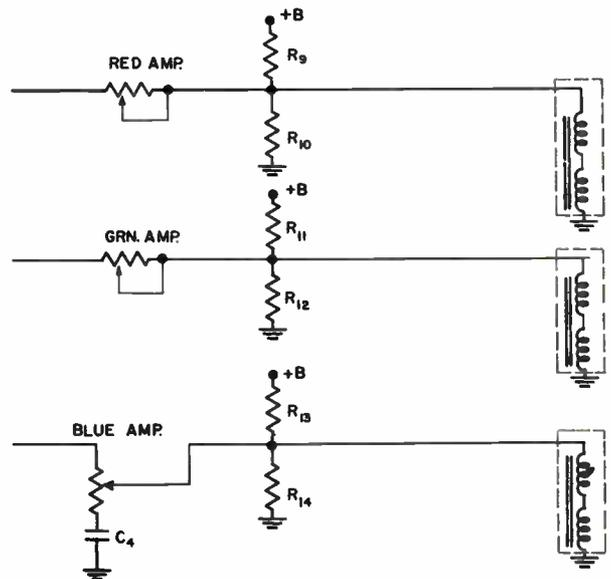
Figure 5-54. Static convergence stabilization.
