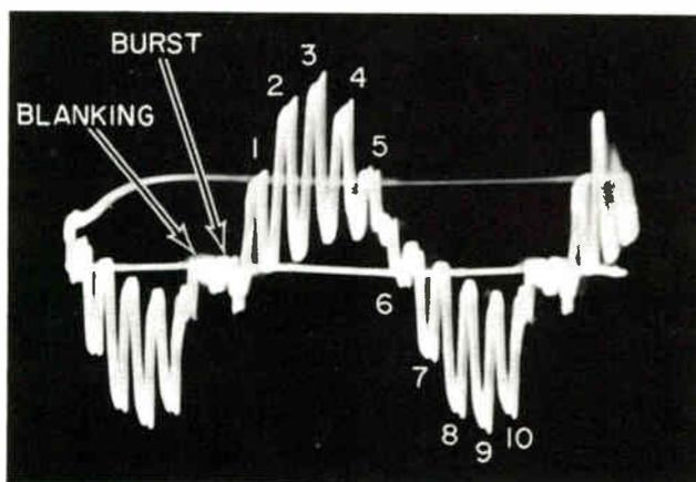
Figure 8-18. Demodulated chroma signal on grid of red electron gun.
