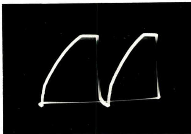
Figure 8-16. Grid waveform of horizontal output tube.
