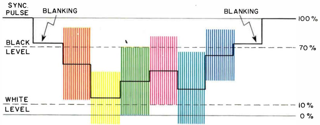
Figure 3-35. Waveform of color-video signal with R-Y and B-Y signals proportionately reduced.
