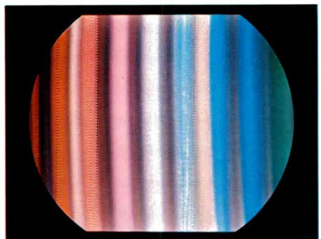
Figure 8-23. Color-bar presentation when G-Y signal is reduced in amplitude.
