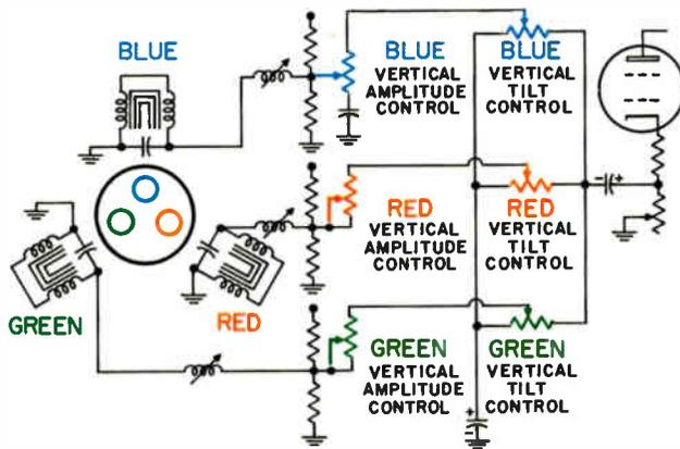
Figure 6-8. Vertical dynamic convergence controls, schematic diagram.
