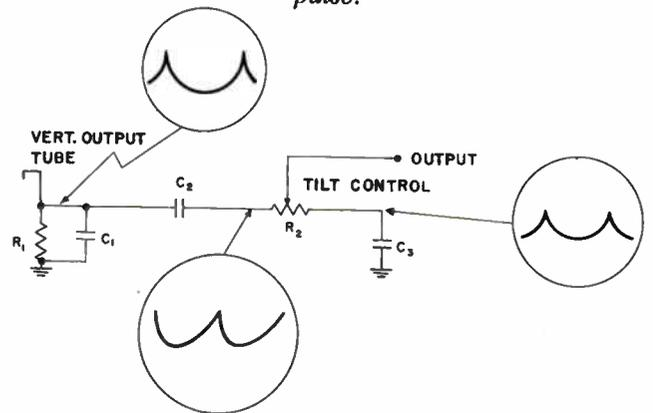
Figure 5-46. Basic vertical dynamic convergence circuit.
