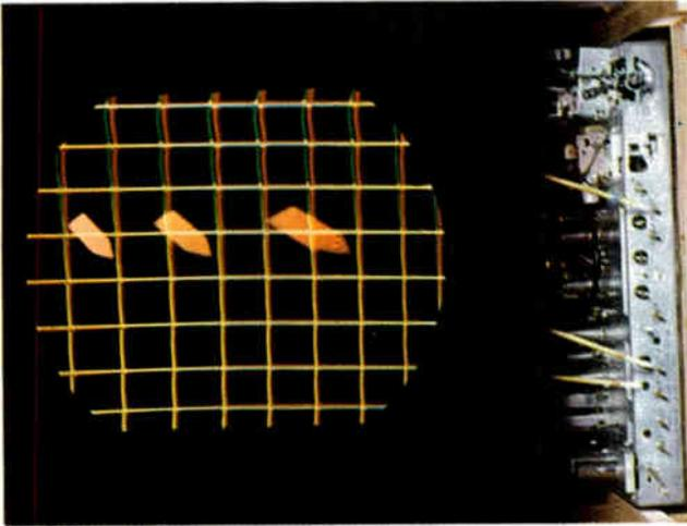
Figure 6-21. Adjustment of red horizontal dynamic phase control.
