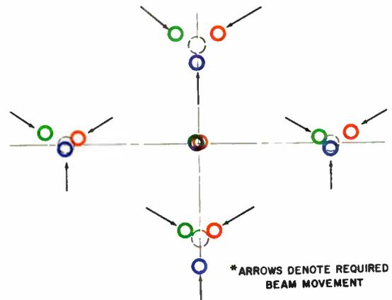
Figure 5-25. Horizontal and vertical convergence corrective forces.
