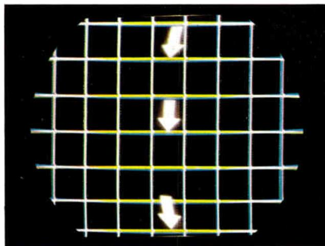
Figure 6-38. Adjustment of blue vertical amplitude control.
