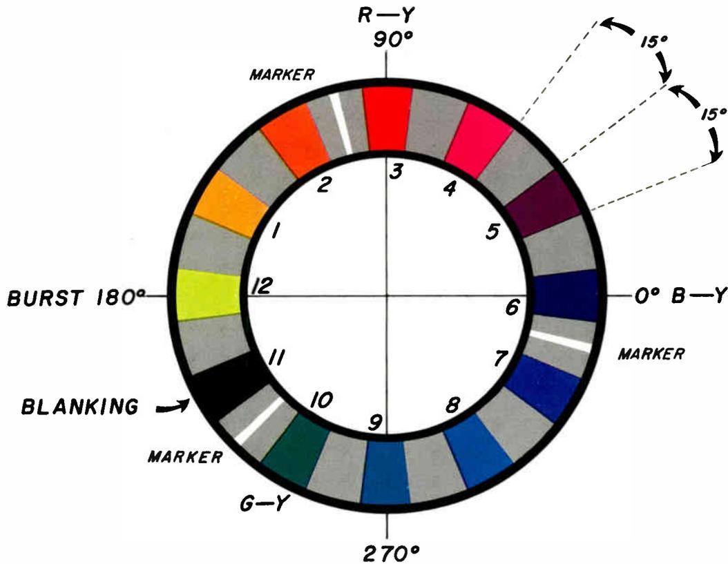
Figure 7-18. Color-bar-generator quadrature graph for master phase adjustment.
