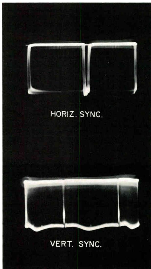
Figure 8-11. Output waveform of sync separator.
