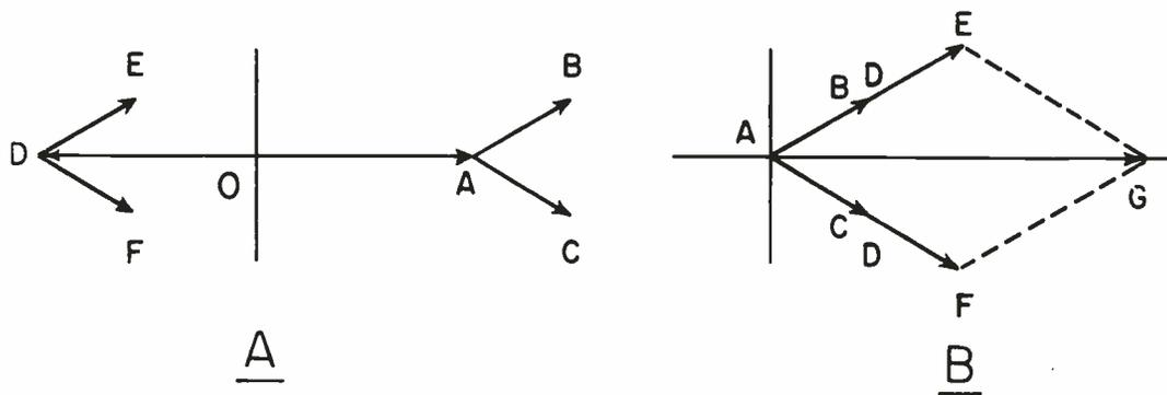
Figure 3-24. Voltage relationship of the suppressed-carrier modulation system with delayed carrier at time A.
