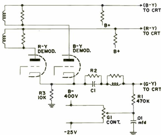
Figure 8-21. Simplified schematic of the demodulator circuit.
