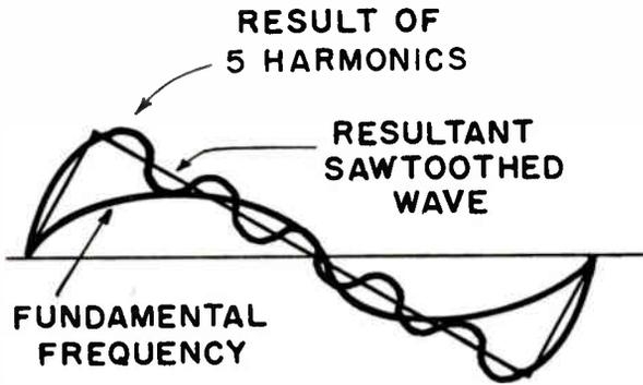
Figure 3-41. Derivation of a sawtooth wave.
