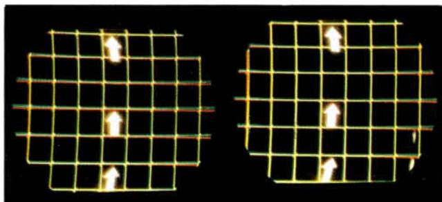
Figure 6-34. Incorrect (left) and correct (right) ratio of red to green vertical amplitude.
