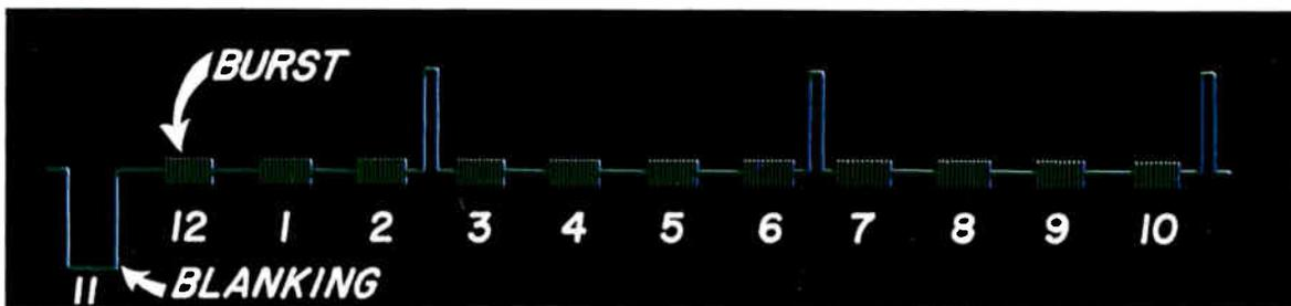
Figure 7-17. Comparison of color-bar-generator signal to color-bar chart on CRT.
