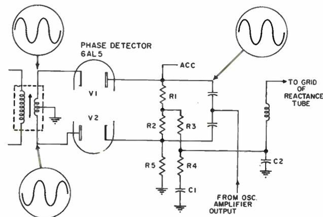
Figure 4-25. Phase detector.
