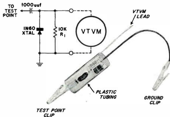
Figure 7-6. R-F probe for vacuum tube voltmeter.
