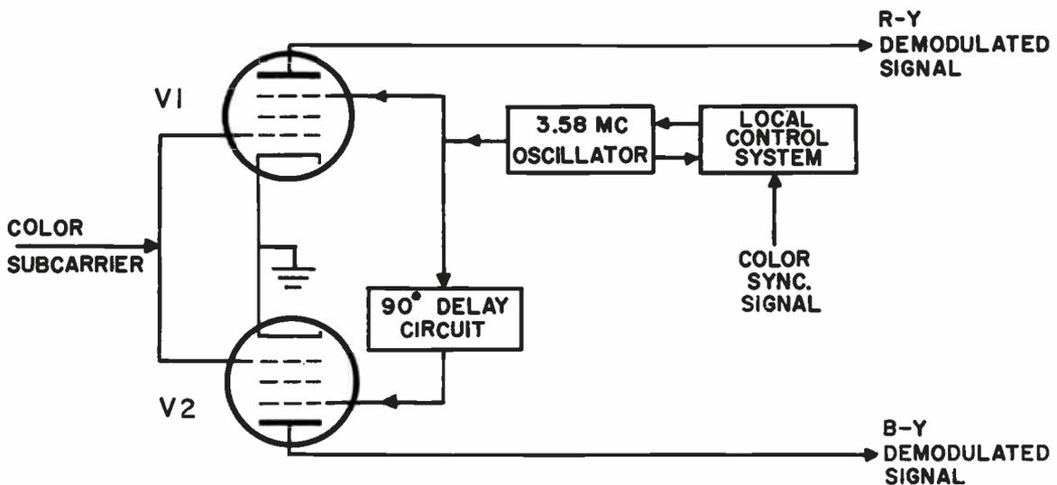
Figure 3-28. Color-subcarrier demodulator.
