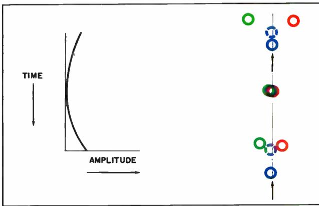
Figure 5-27. Vertical dynamic convergence of blue beam.
