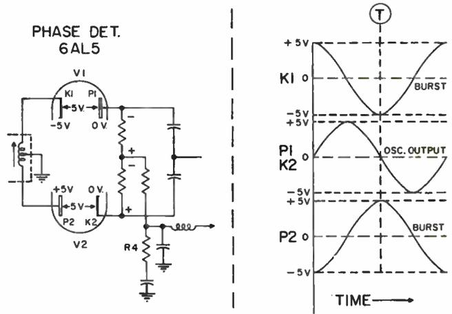
Figure 4-26. Phase detector in balanced condition.
