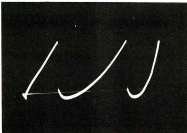
Figure 8-13. Waveform at grid of vertical output tube.
