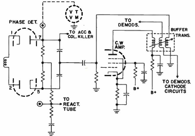
Figure 7-16. C-W amplifier adjustment.
