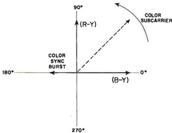
Figure 3-31. Phase relationships of the R-Y, B-Y and burst signals.
