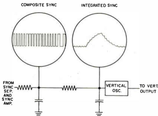
Figure 1-16. Integrator circuit
