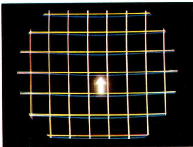
Figure 6-43. Adjustment of blue horizontal phase control.
