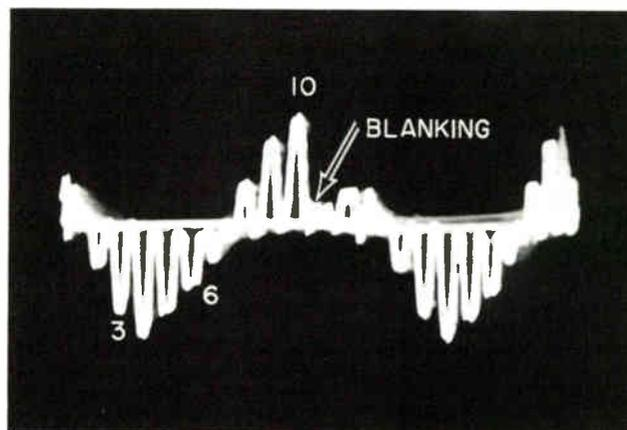
Figure 8-20. Demodulated chroma signal on grid of green electron gun.
