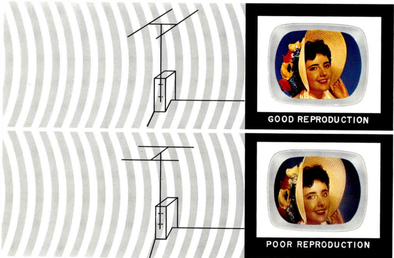
Figure 9-1. Effect of antenna installation.
