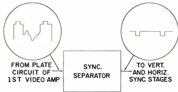
Figure 1-11. Sync separator, input and output waveforms
