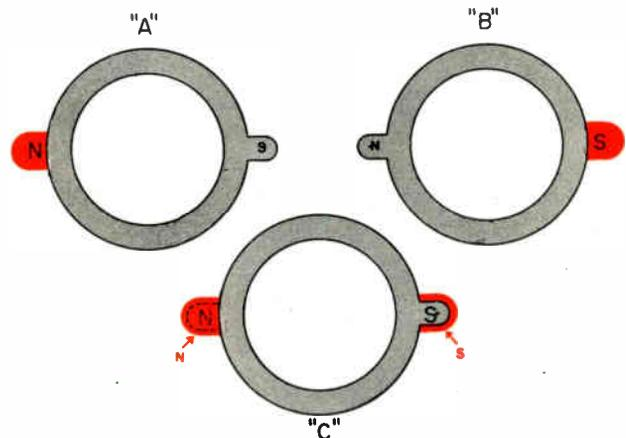
Figure 5-12. Color purity magnet assembly.
