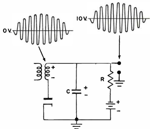
Figure 4-12. Detector circuit with voltage applied.
