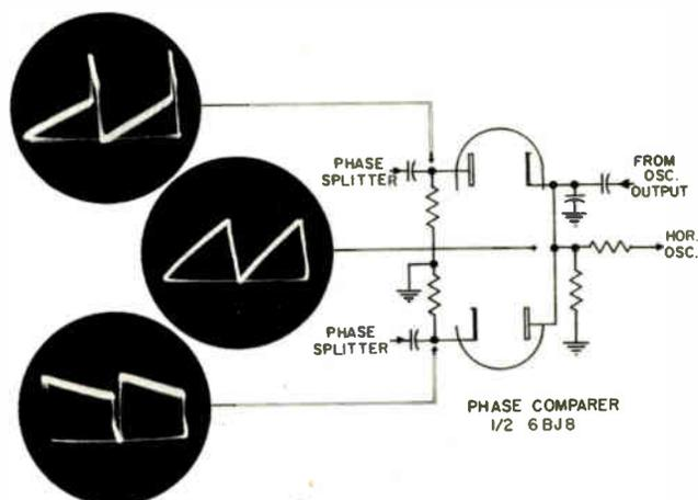
Figure 8-15. Waveforms of phase comparer.
