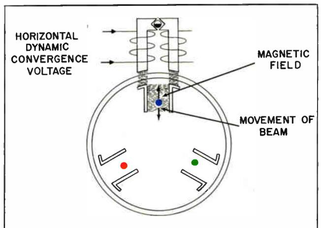
Figure 5-30. Blue convergence assembly with winding for horizontal dynamic convergence.
