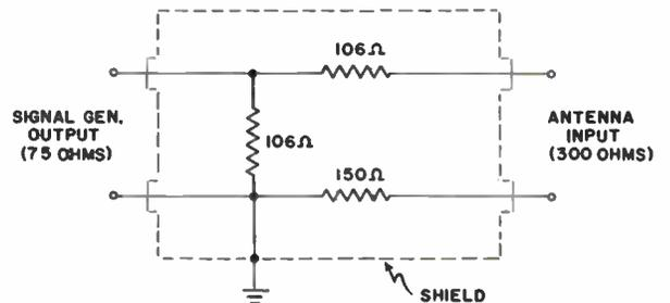
Figure 7-3. Antenna-matching network.
