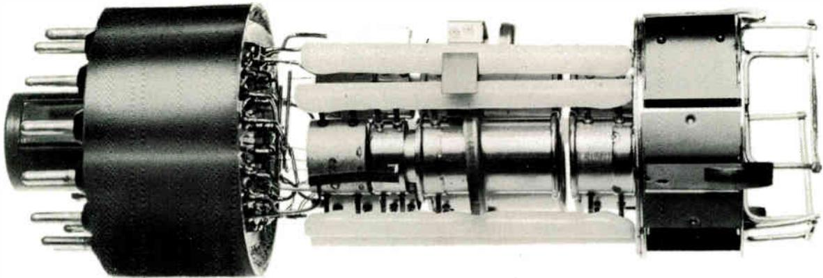
Figure 5-3. Tri-gun assembly.
