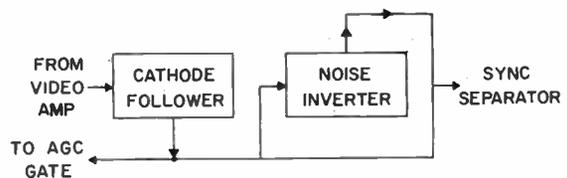
Figure 1-12. Noise inverter, block diagram
