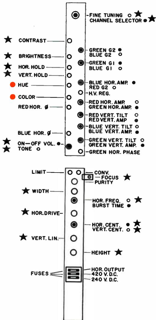
Figure 6-2. Location of receiver chassis adjustment controls.
