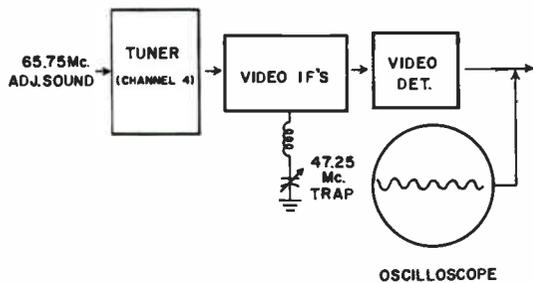
Figure 7-9. Centering the fine tuning control, block diagram.
