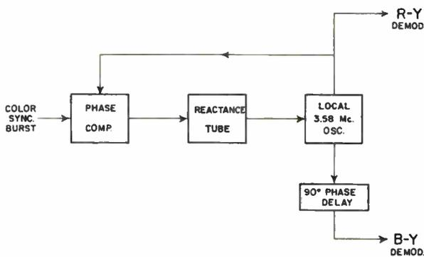
Figure 3-32. Synchronizing the carrier signals.
