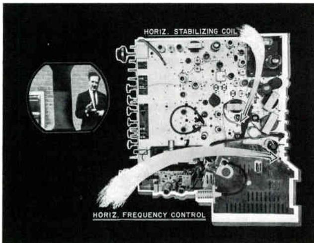
Figure 6-14. Adjustment of horizontal oscillator circuit.
