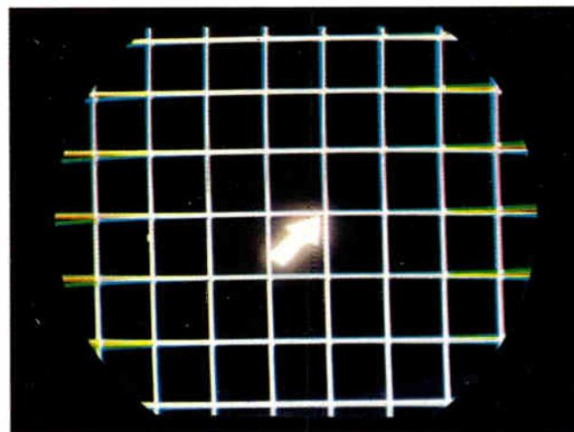
Figure 6-39. Static convergence of the red, green and blue beams at center of screen.
