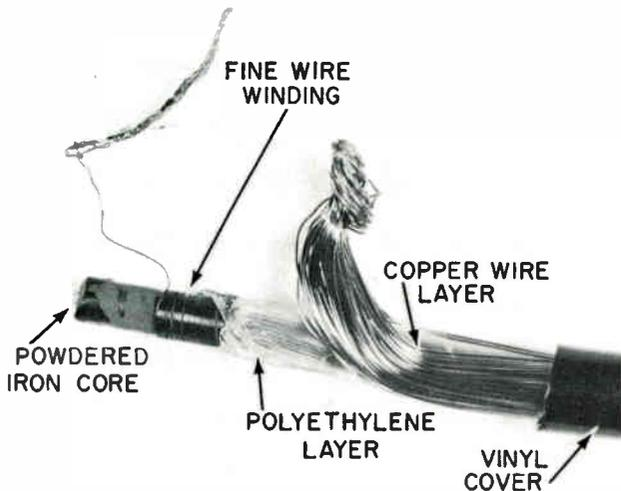
Figure 4-5. The delay line.
