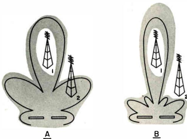
Figure 9-12. Change in reception pattern with change in channel frequency.
