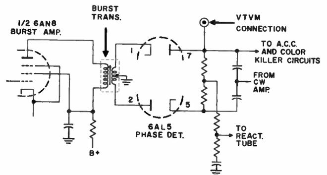
Figure 7-14. Burst phase-detector circuit with VTVM connected for test.
