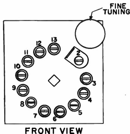
Figure 7-7. Tuner oscillator adjustments.
