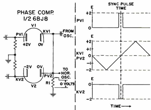
Figure 4-36. Oscillator frequency in synchronism with sync pulses.
