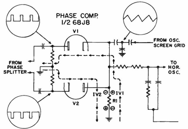
Figure 4-35. Horizontal phase comparer.
