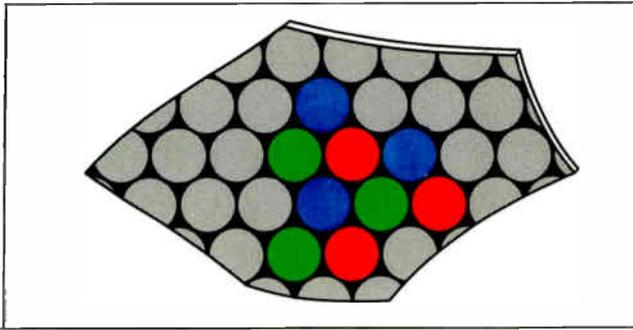
Figure 5-14. Convergence of the three electron beams.
