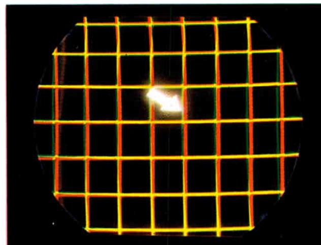
Figure 6-32. Adjustment of green vertical tilt control.
