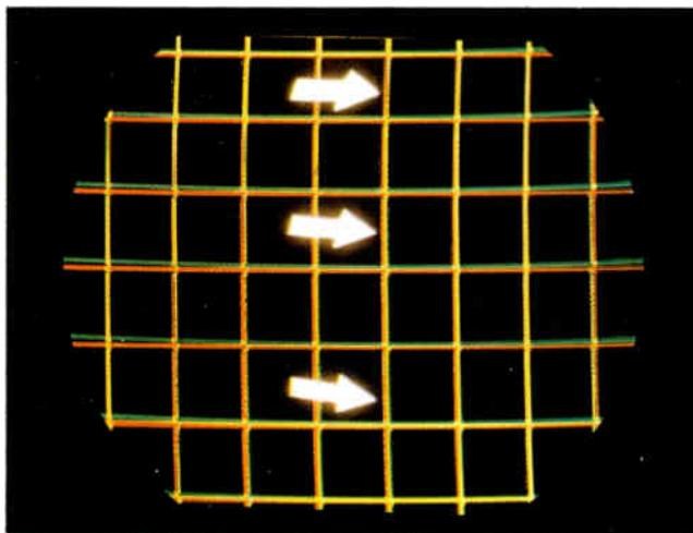
Figure 6-33. Final adjustment of red and green vertical amplitude controls.
