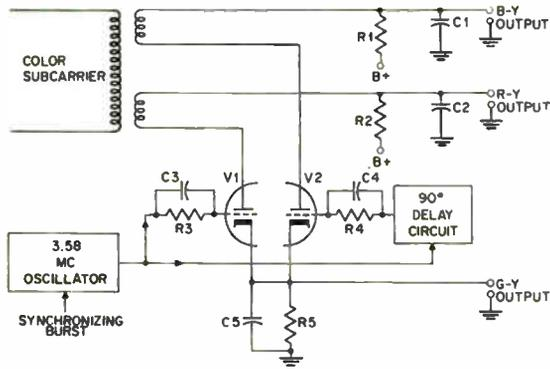
Figure 4-18. Complete demodulator circuit.
