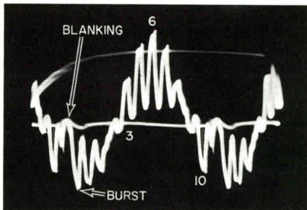
Figure 8-19. Demodulated chroma signal on grid of blue electron gun.
