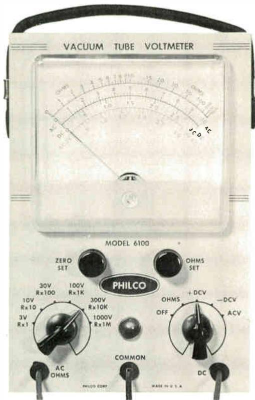
Figure 8-1. Philco Vacuum Tube Voltmeter, Model 6100.
