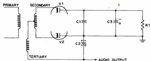
Figure 4-8. Simplified schematic of a ratio detector.
