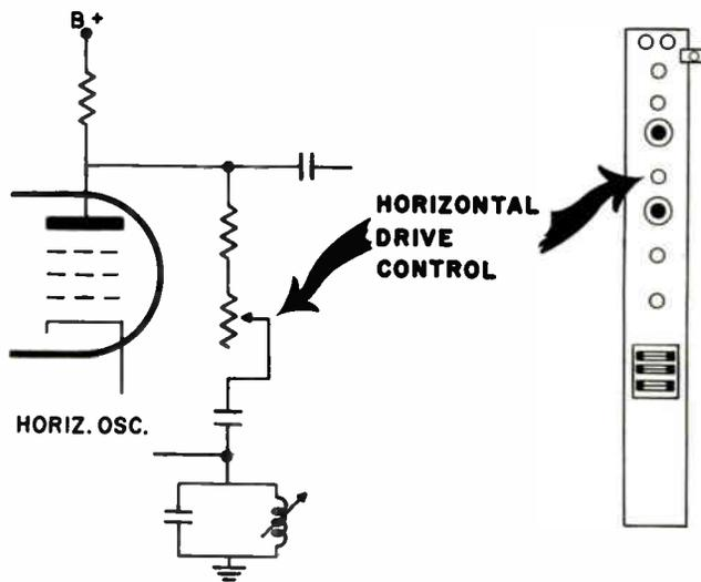
Figure 6-6. Horizontal drive control, location and circuitry.
