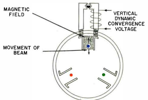
Figure 5-26. Blue convergence assembly with winding for vertical dynamic convergence.
