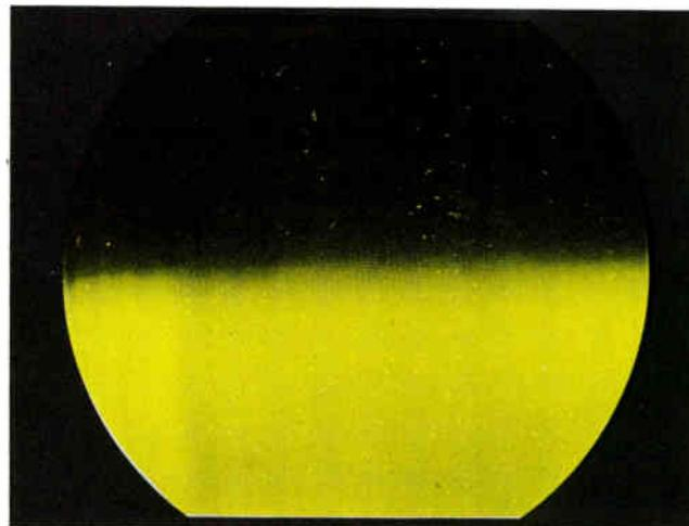
Figure 6-49. Adjustment of green G1 and G2 controls for yellow field.
