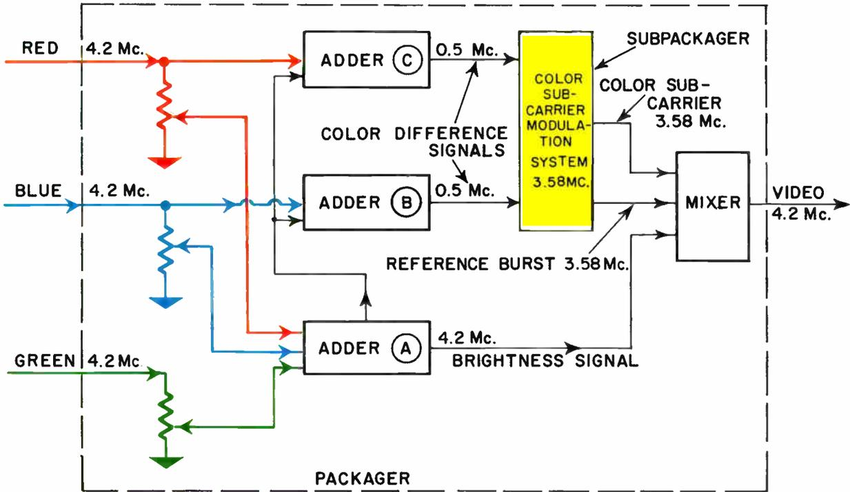
Figure 3-5. Transmission of the composite color signal.
