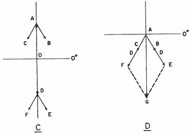
Figure 3-22. Voltage relationship of the suppressed-carrier modulation system at time B.
