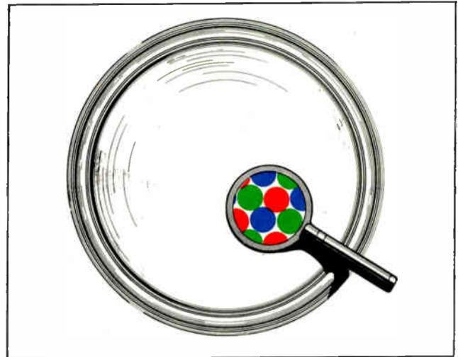
Figure 5-15. Magnified area of phosphor screen.
