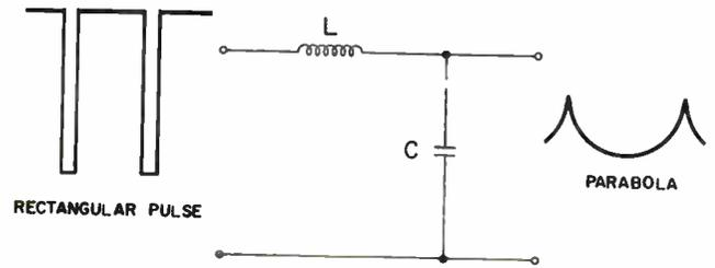
Figure 5-45. Double integration of a rectangular pulse.
