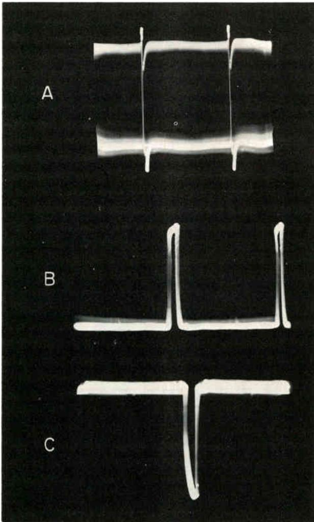
Figure 8-12. Output waveforms of phase splitter.
