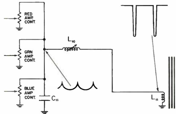
Figure 5-49. Horizontal dynamic amplitude control circuit.
