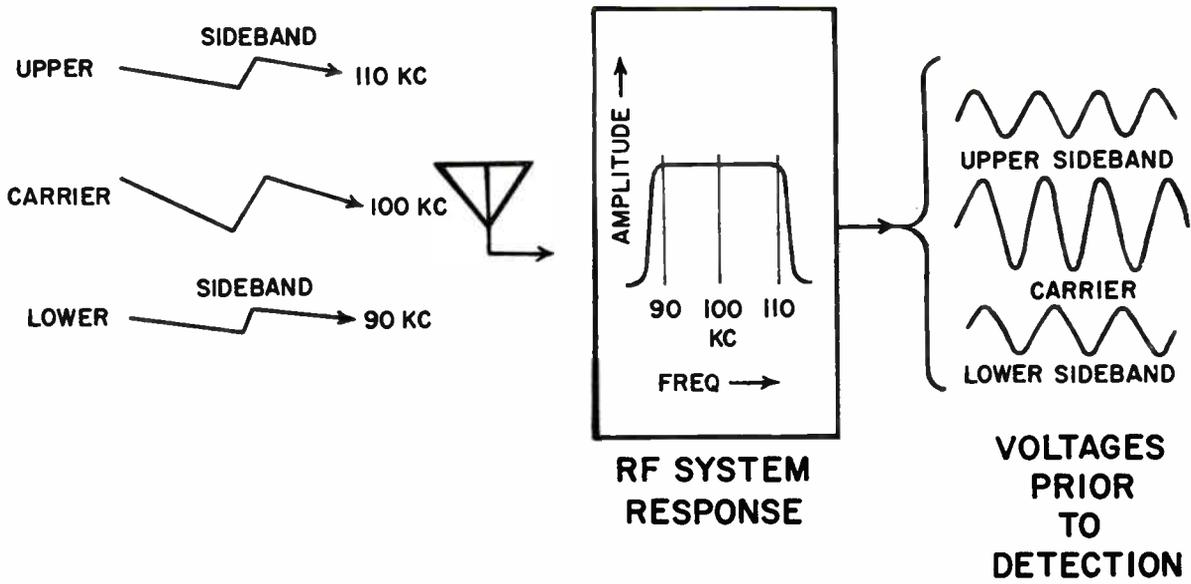
Figure 3-18. Reception of an amplitude modulated signal.
