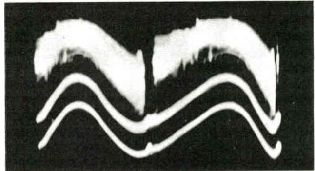
Figure 8-5. Composite color signal with 60-cycle hum.
