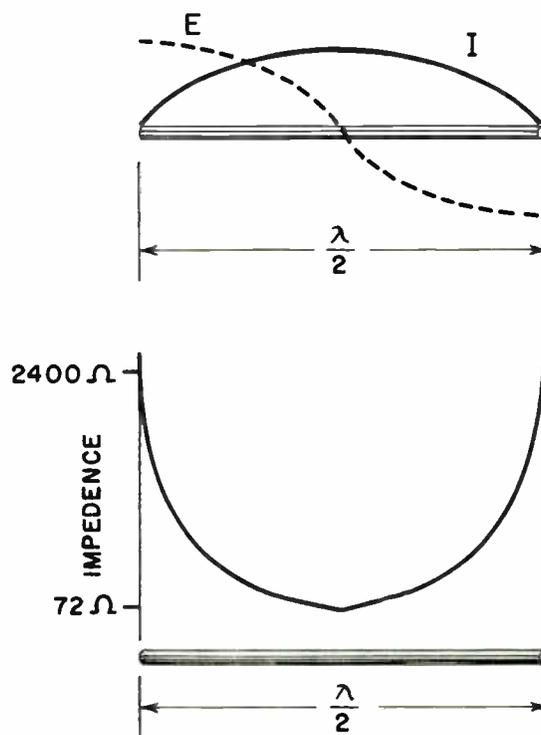
Figure 9-8. Voltage and current distribution and the corresponding impedance curve for a half-wave antenna.
