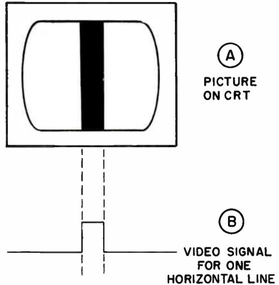
Figure 3-42. Rectangular wave video signal.
