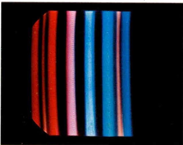
Figure 8-25. Color-bar presentation when common cathode resistor reduces in value.
