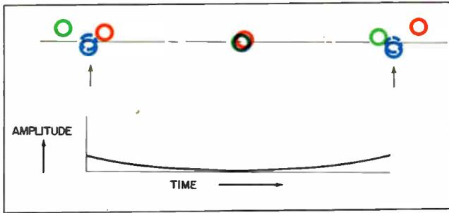
Figure 5-31. Horizontal dynamic convergence of blue beam.
