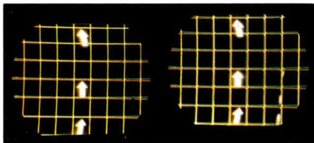
Figure 6-35. Incorrect (left) and correct (right) ratio of red to green vertical tilt.
