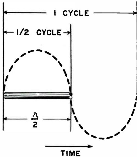
Figure 9-5. Determination of half-wave antenna.
