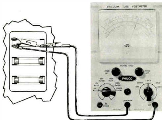
Figure 6-12. Measuring the horizontal output circuit current.
