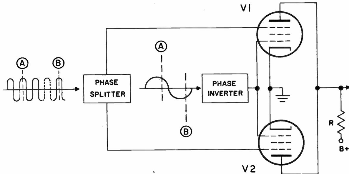
Figure 3-20. Suppressed-carrier modulation system.
