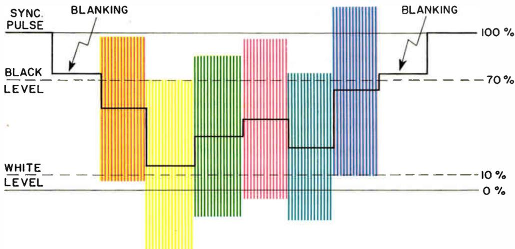
Figure 3-34. Waveform of the color-video signal with R-Y and B-Y signals containing saturated colors.
