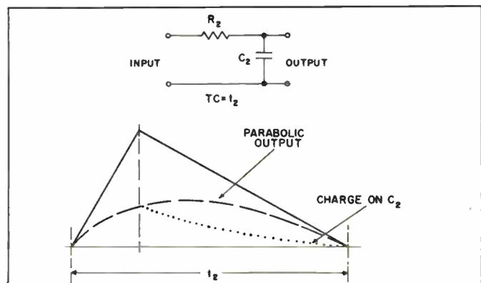
Figure 5-43. Effect of time constant to parabolic output.
