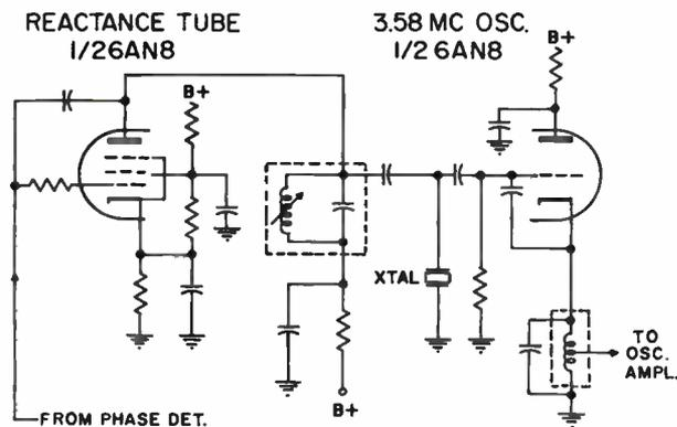
Figure 4-28. Reactance tube and 3.58-mc oscillator.
