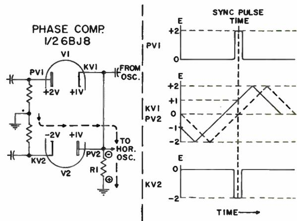
Figure 4-37. Oscillator frequency higher than sync pulse frequency.
