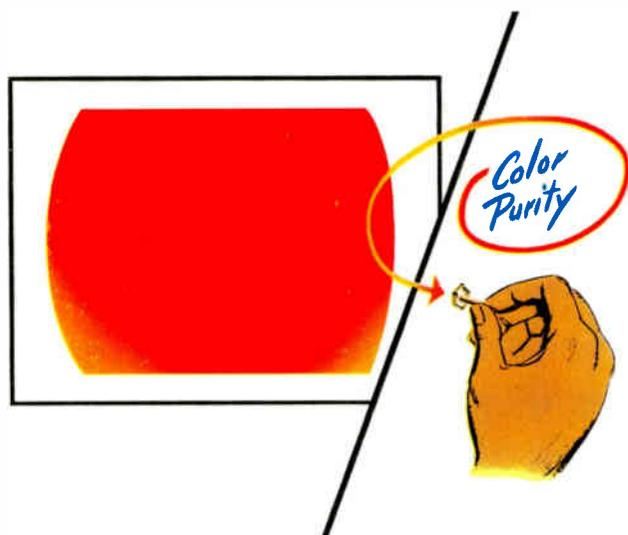
Figure 9-3. Color purity adjustment.
