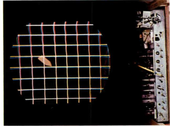
Figure 6-24. Adjustment of blue horizontal dynamic amplitude control.
