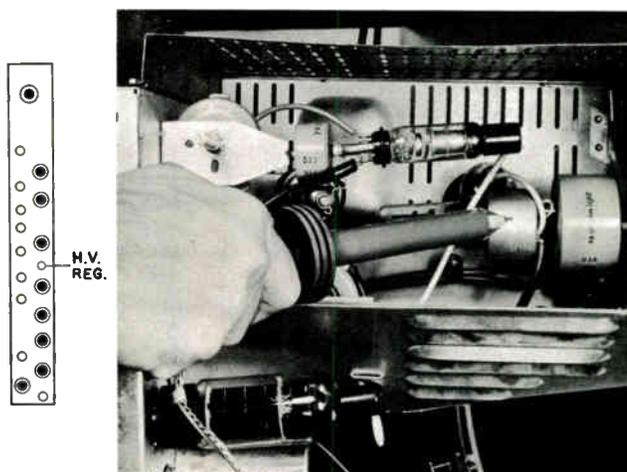
Figure 6-11. Test point for measuring the high voltage.
