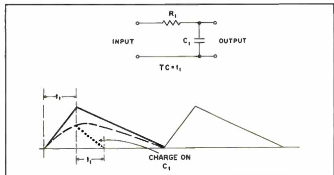
Figure 5-42. Development of a parabolic from a sawtooth.
