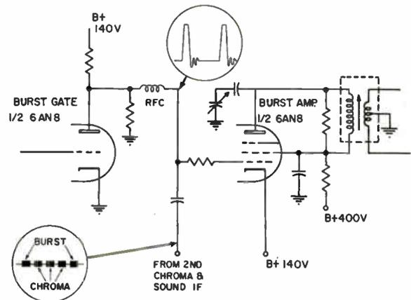
Figure 4-24. The gate clamp and burst amplifier.
