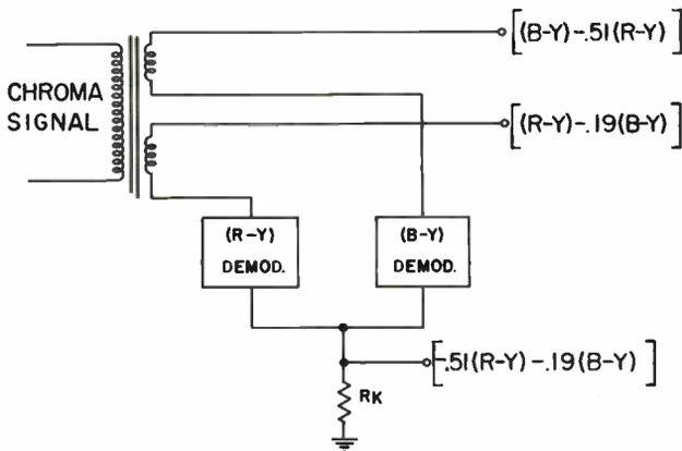
Figure 4-19. Plate output signals indicate the need for a revision of the demodulation phase angles.
