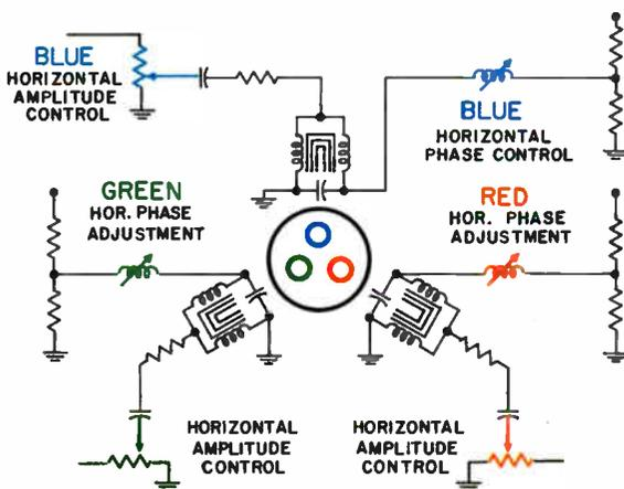
Figure 6-9. Horizontal dynamic convergence controls, schematic diagram.
