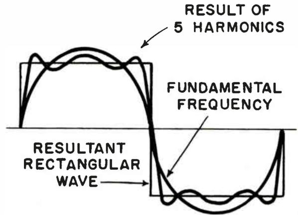
Figure 3-40. Derivation of a rectangular wave.
