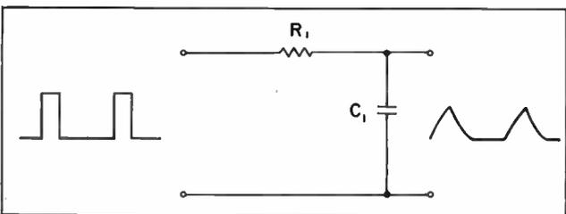
Figure 5-39. Integration of a rectangular wave.
