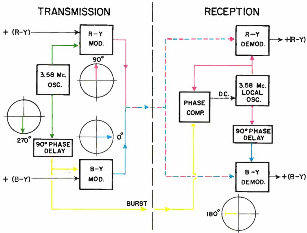
Figure 3-33. Modulation and demodulation of the color subcarrier.
