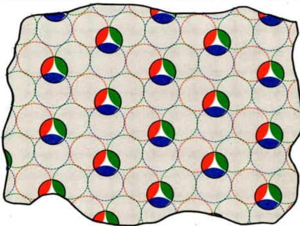
Figure 5-8. Relative placement of shadow mask to phosphor screen.
