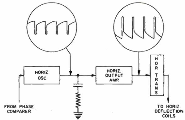
Figure 1-19. Horizontal deflection circuits
