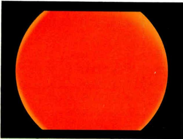
Figure 6-27. Improved red field purity by deflection yoke adjustment.
