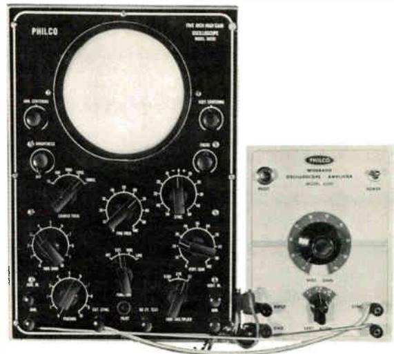
Figure 8-3. Philco Oscilloscope, Model S-8202 and Philco Wideband Oscilloscope Amplifier, Model 8300.
