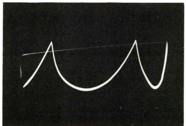
Figure 8-14. Convergence voltage at cathode of vertical output tube.
