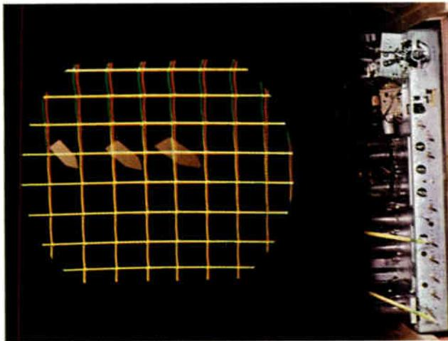
Figure 6-22. Adjustment of green horizontal dynamic phase control.
