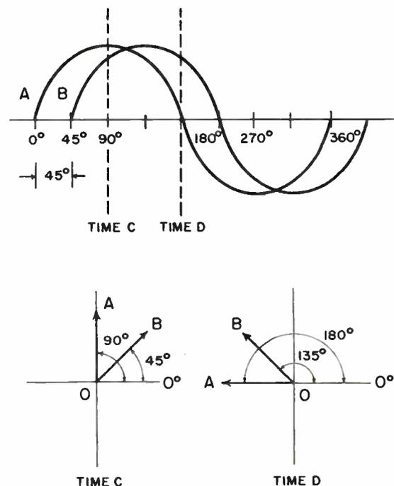
Figure 3-12. Comparison of two sinewaves of same frequency.
