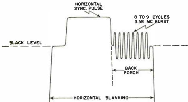
Figure 3-30. The burst signal.
