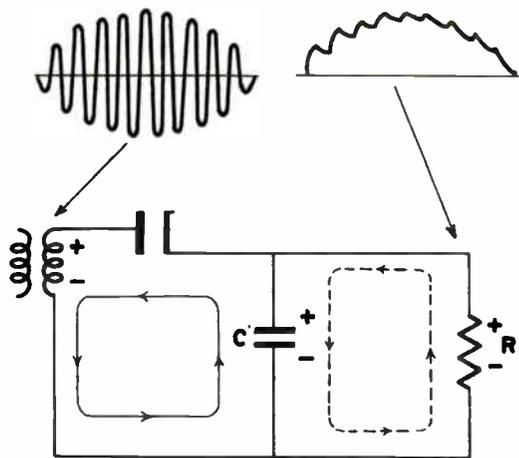
Figure 4-10. Basic series detector.
