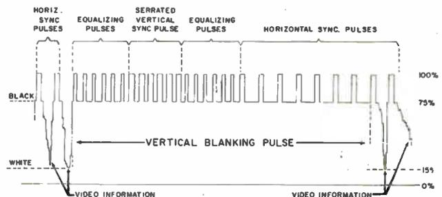
Figure 1-2 Composite video signal
