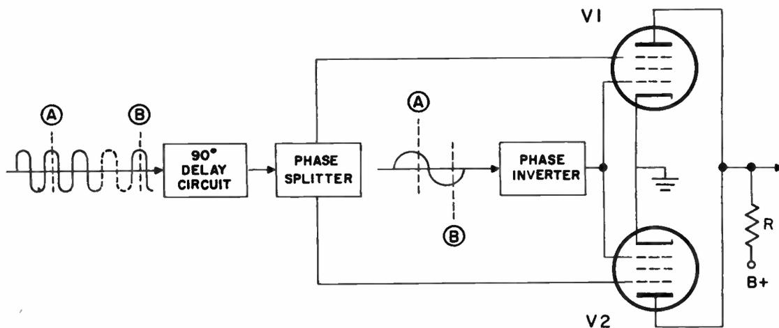
Figure 3-23. Suppressed-carrier modulation system with delayed carrier.
