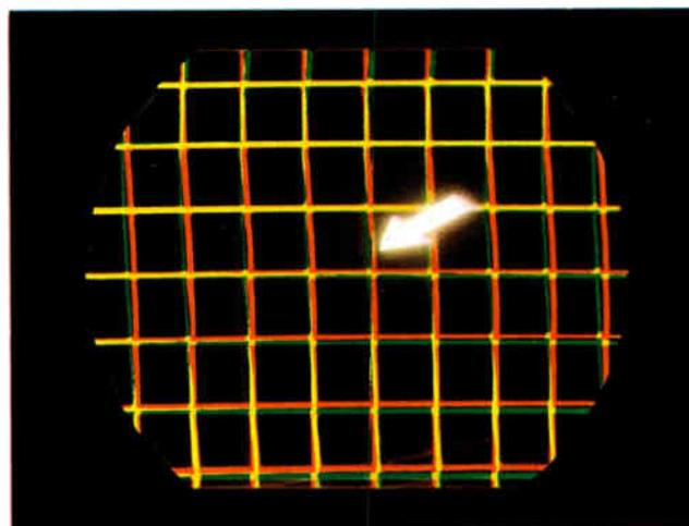
Figure 6-31. Adjustment of red vertical tilt control.
