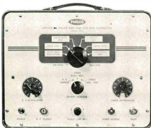
Figure 8-2. Philco Universal Color Bar and Dot Bar Generator, Model 7100.
