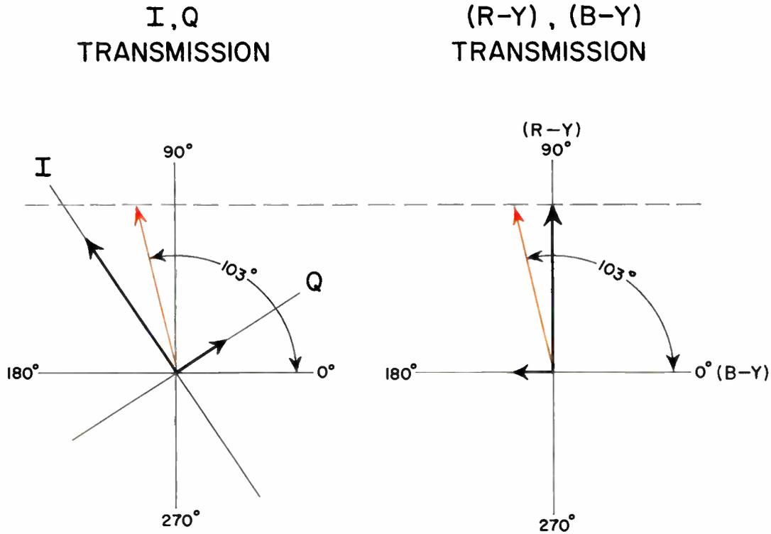
Figure 3-37. Vectorial analysis of identical signals transmitted by I-Q and (R-Y)-(B-Y) color-difference signals.
