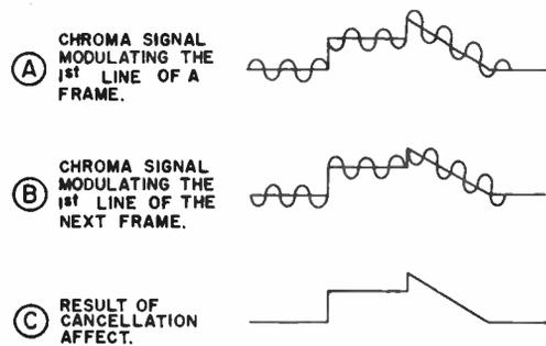
Figure 3-44. Interference cancellation in frequency interleaving.
