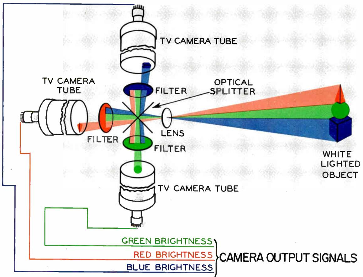
Figure 3-1. Fundamental arrangement for color pick-up.
