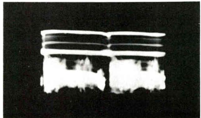
Figure 8-6. Video signal at the output of the video amplifiers.
