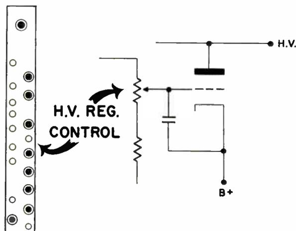
Figure 6-5. H.V. regulator control, location and circuitry.
