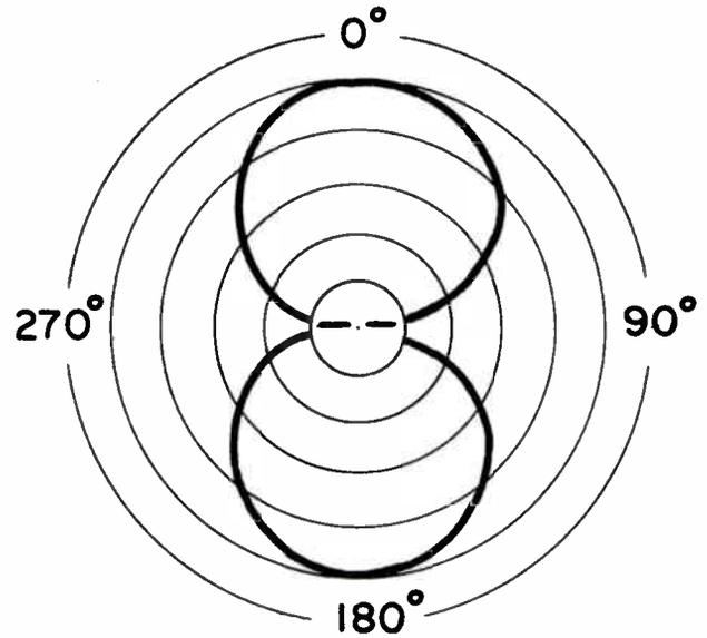
Figure 9-6. Field pattern of dipole.
