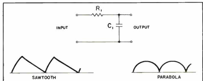
Figure 5-41. Integration of a sawtoothed wave.
