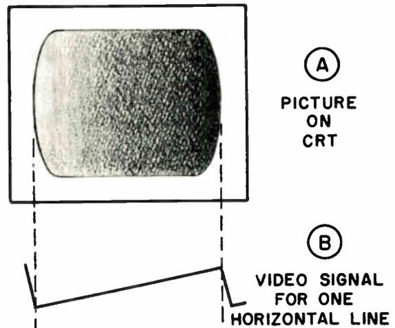
Figure 3-43. Sawtooth wave video signal.
