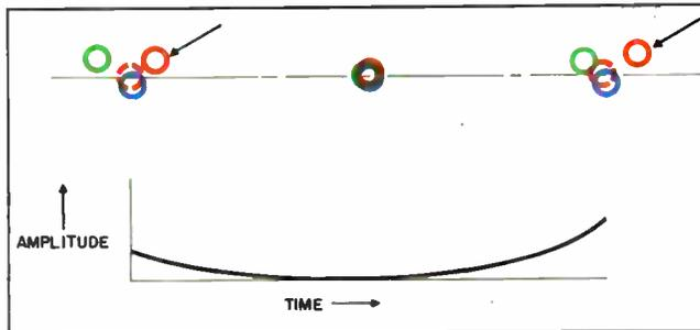
Figure 5-33. Horizontal dynamic convergence of red beam.
