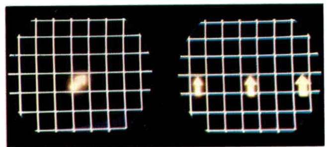
Figure 6-44. Adjustment of blue horizontal amplitude control (right) and final static convergence (left).
