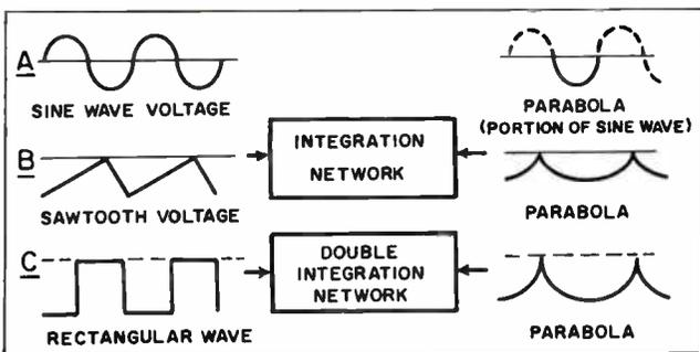
Figure 5-37. Development of parabolic voltages.
