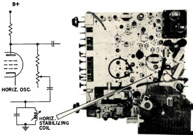
Figure 6-7. Horizontal stabilizing coil, location and circuitry.
