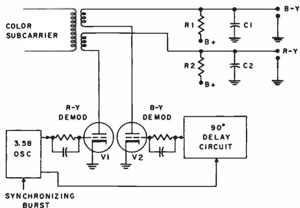
Figure 4-16. Basic demodulator.
