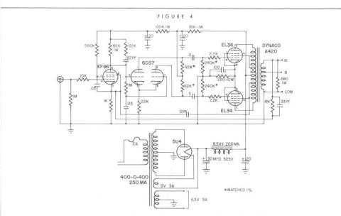
IMPROVED MULLARD 30 WATT AMPLIFIER USING DYNACO A-420 TRANSFORMER
