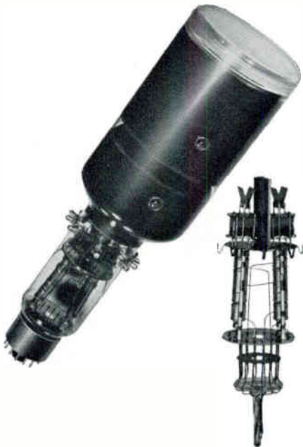
Figure 1. The Du Mont Type 5SP Dual-Beam Cathode-ray Tube showing the structure of its electron guns. The two guns are physically separate and are shielded to prevent interaction between the deflection plate associated with each.
