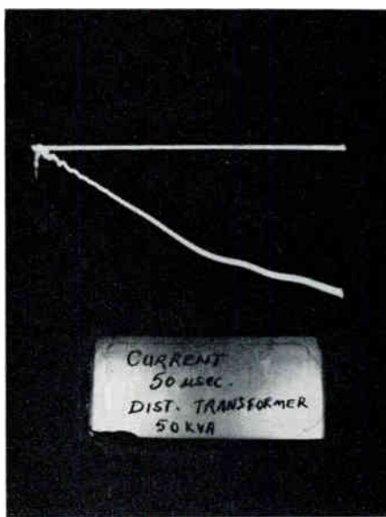
Figure 6. A current wave as recorded by the Du Mont Type 293 during an actual impulse test of a distribution transformer
