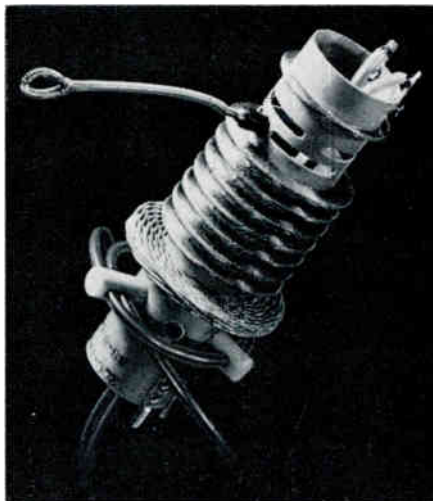
Figure 2. The r-f transformer of the Type 263-B High-Voltage Power Supply
