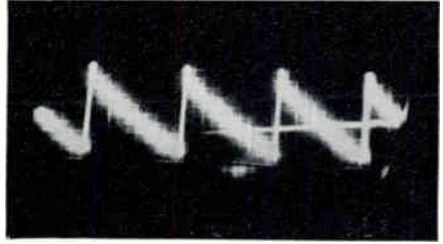
Figure 7. This oscillogram was deliberately overexposed to record the high-writing-speed portions of the trace
