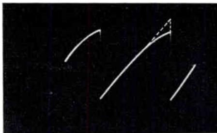
Figure 6. Oscillogram of a non-linear sawtooth voltage (solid line) showing comparison with a perfectly linear sawtooth (dotted line)
