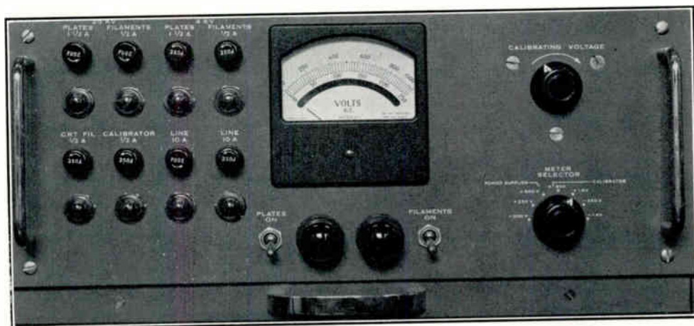
Figure 3. A portion of the control panel of the Type 293 showing the voltage-calibrator controls and meter
