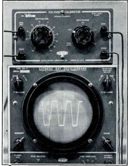
Figure 3. Same as Figure 2 except that the OUTPUT MULTIPLIER switch has been turned to the X.1 Position resulting in the calibration voltage appearing on the screen
