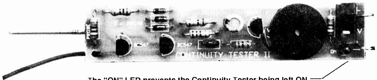
The "ON" LED prevents the Continuity Tester being left ON.
